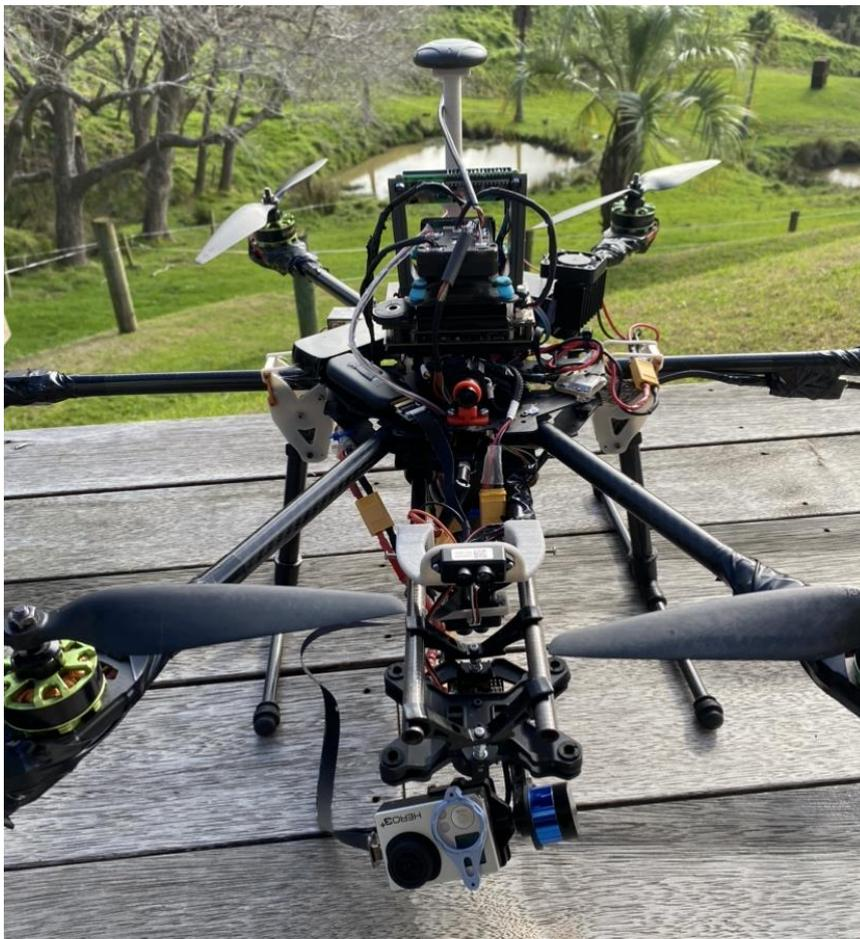
Figure 17: Drone Platform
