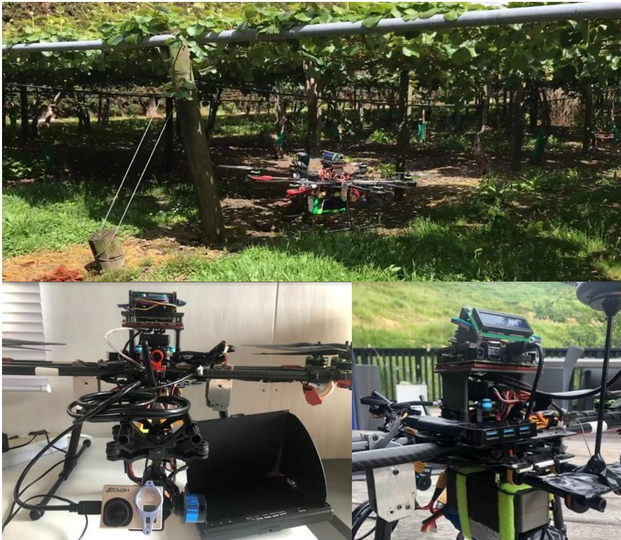
Figure 30: Early orchard test flight [Top], Upside down GoPro mount, without ribbon micro to standard HDMI cable [Left]. Rear of drone [Right].
