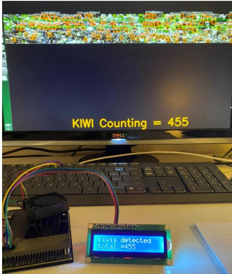
Figure 49: YOLOv7-Tiny on JETSON Nano + LCD
