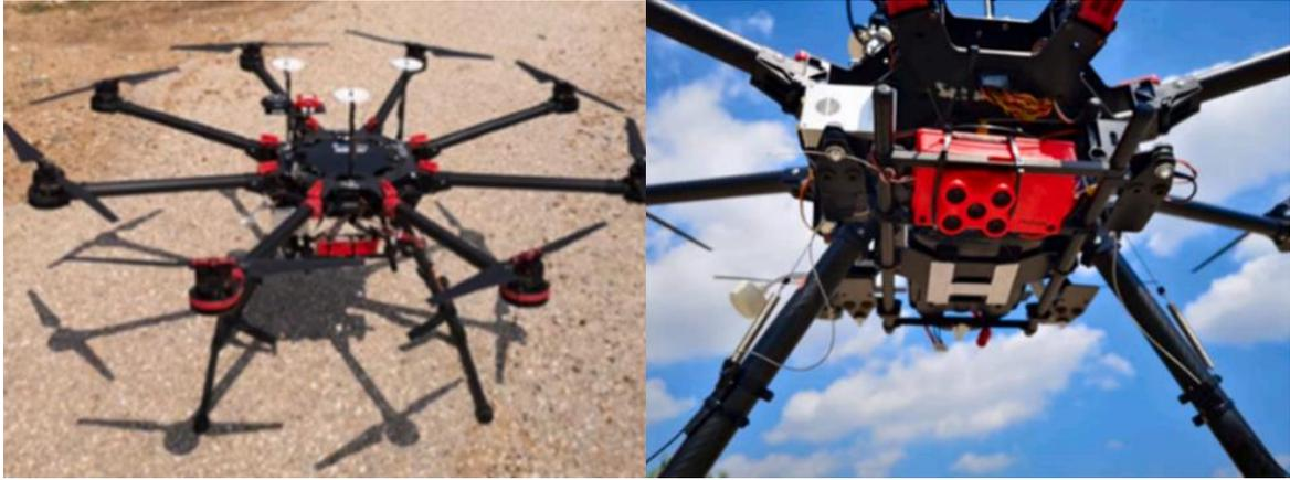
Figure 7: Octocopter, GPS triangulation Left, Multispectral camera Right.
