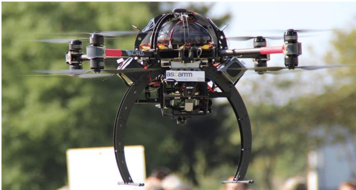
Figure 63: Droidwork Skyjib X4 with dual batteries. [74].
