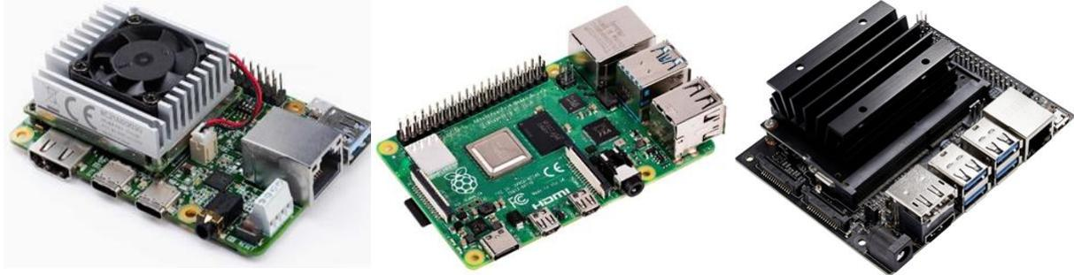
Figure 15: Microprocessors. Coral Edge Board [Left], Raspberry Pi 4 [Middle], Nvidia Jetson Nano [ Right].
