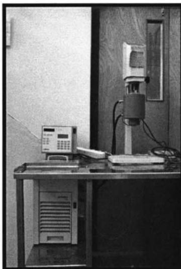
Figure 3.11: Paar Physica MC1 and Julabo water bath
