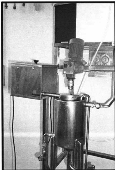
Figure 3.4: Powder mixing system
