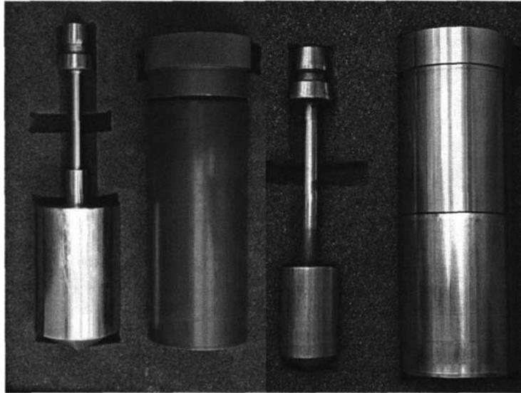
Figure 3.12: Paar Physica MC1 spindles Z2,1 (left bob and cup) and Z3 (right bob and cup)
