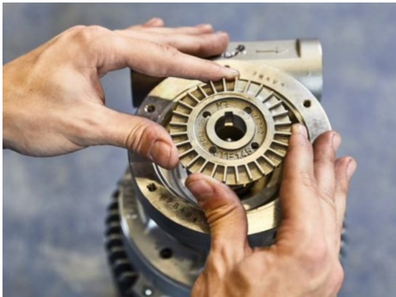
Figure 8, showing the pump impellor used in the EDUR multiphase pump, (edur.com,2023)
