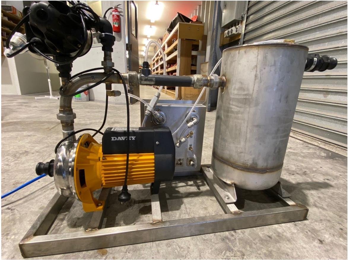
Figure 13 - The NBA Nanobubble Generator showing the commercially available NBT, (rear view). The water inlet is on the left hand side and the outlet on the right
