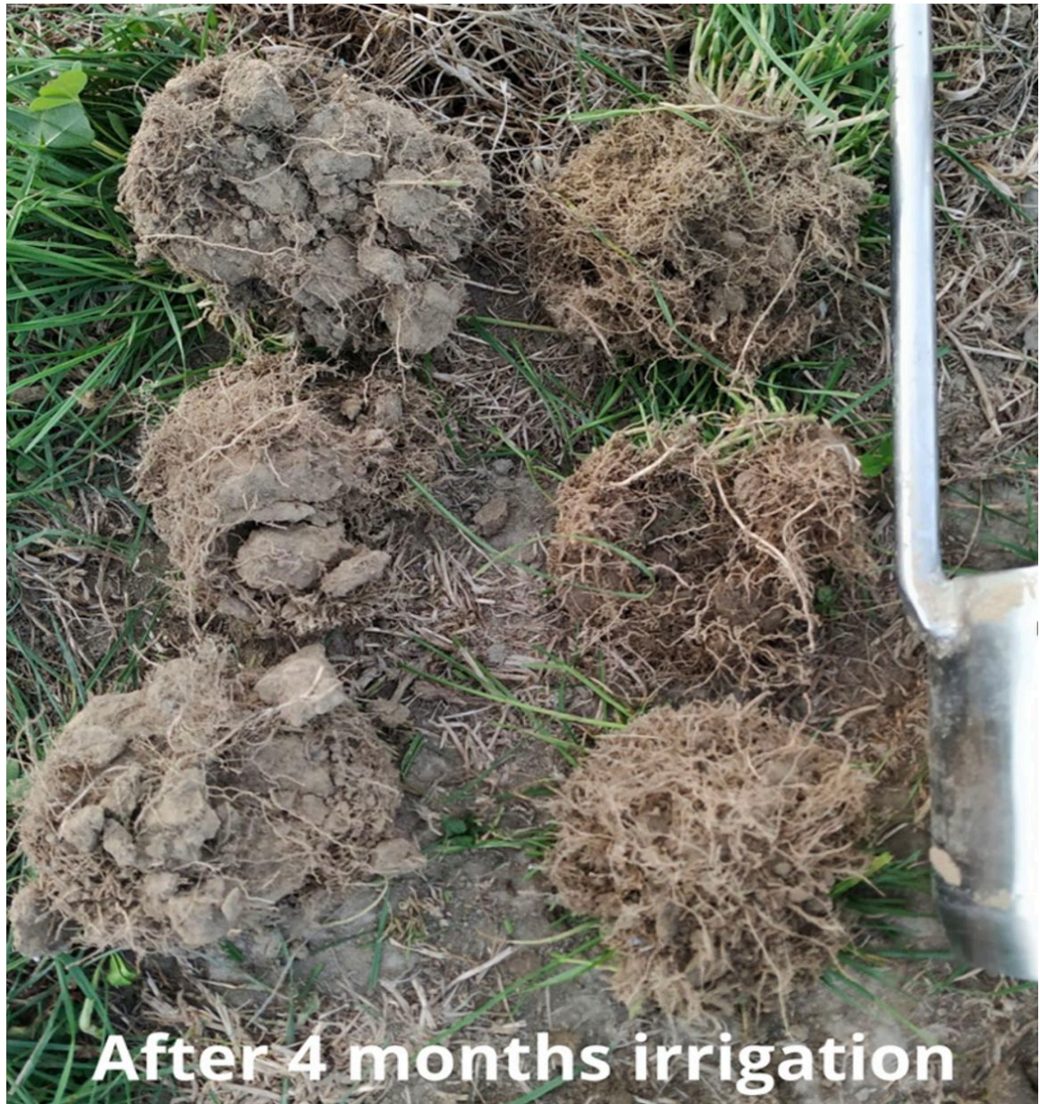
Figure 29 - Image showing 100 mm core diameter, soil samples: The samples on the left hand side of the image have been irrigated using untreated water; the samples on the right hand side of the image have been irrigated using water enriched with oxygen nanobubbles.
