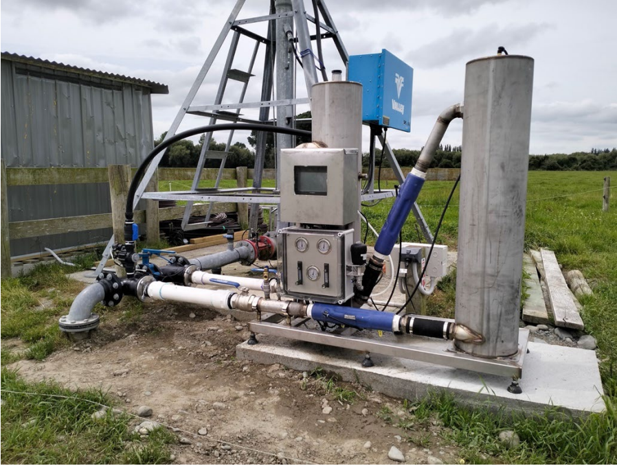
Figure 35 - Nanobubble Agritech Generator, South Island dairy farm
