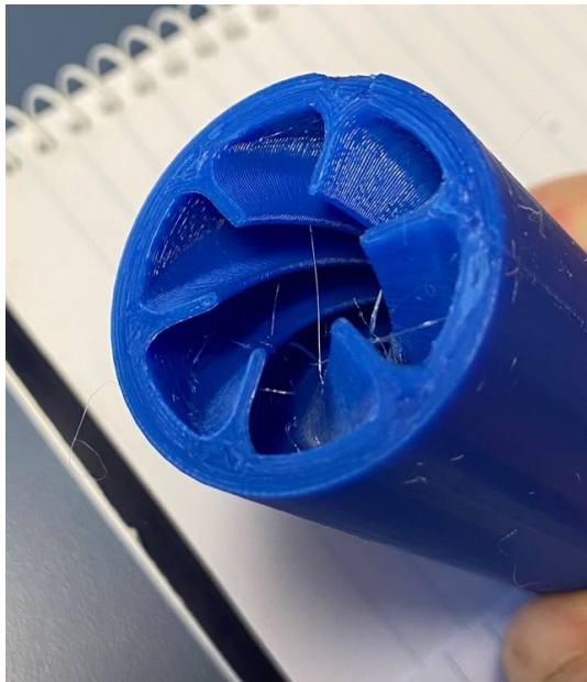
Figure 23 - Nanobubble tube showing 6 fins
