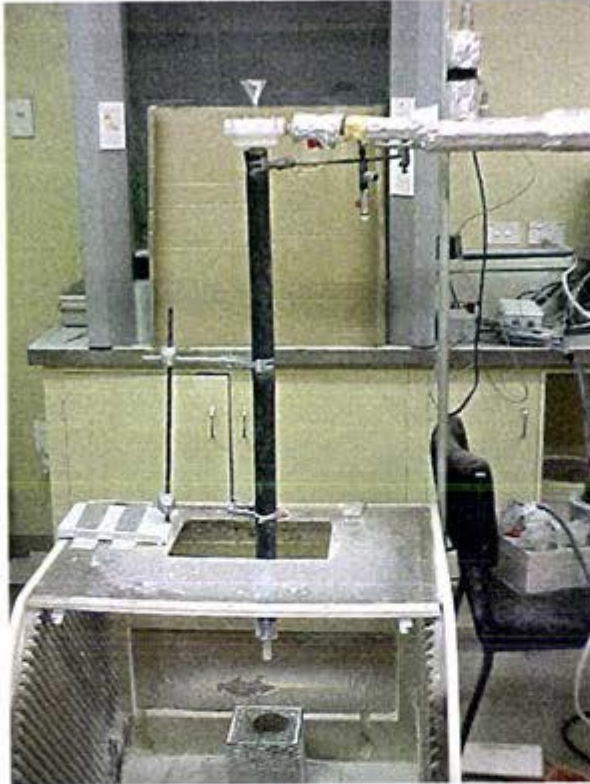
Figure 3.4 This part of the particle-gun shows where powder feed from the glass funnel and firing on the stainless steel plate occur.
