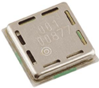
Fig.5.3 (a) MA40H1S-R transmitter
