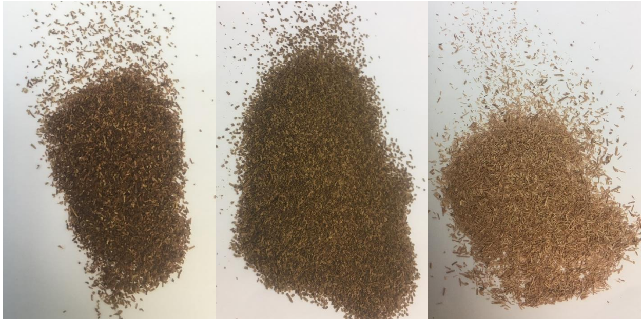
Figure 3: (Left to Right) RYO tobacco, HEETS and kānuka sample at 250-600 microns.
