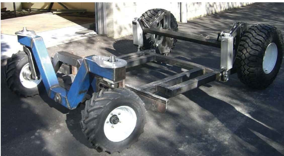
Figure 7-1: Chassis during construction, pre finishing
