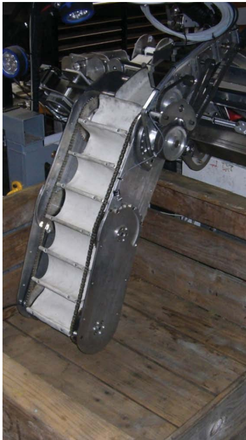
Figure 6-31 Depositing arm shown without its top fruit retaining enclosure
