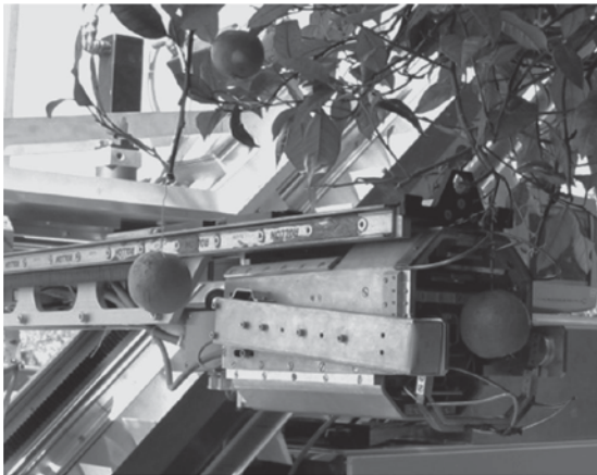
Figure 6-10: Hand implemented on the latest prototype harvester, (Muscato, et al., 2005).
