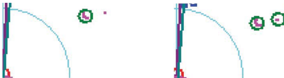
Figure 7-57: Two consecutive LIDAR scans showing occlusion hindering correct classification (left). The LIDAR scanner is positioned in the lower left hand edge of each scan image.
