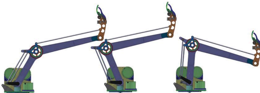
Figure 6-3: Parallel linkage maintaining a vertical hand throughout range of motion
