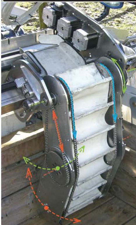
Figure 6-34: Bin filling manipulator drive
