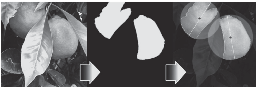
Figure 5-2 Image processing to locate the oranges in an image (Muscato, et al., 2005)
