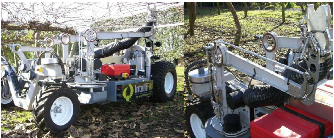
Figure 6-18: Left: Image of the robotic arm mounted on the chassis in the harvesting position. Right: Image of the hand and arm assembly showing all of the external components and linkages.
