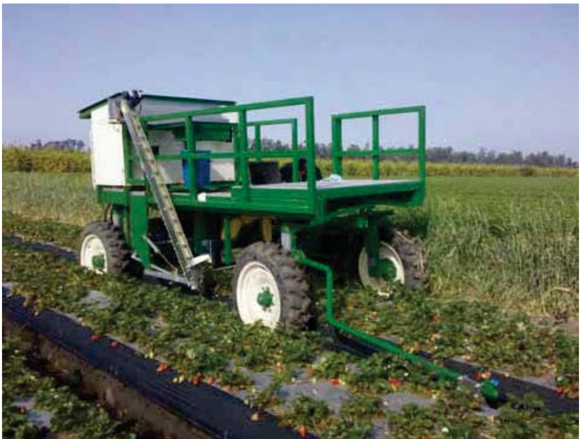
Figure 2-7: Robotic Harvesting LLC strawberry harvesting robot. Image from (Rose, 2010).
