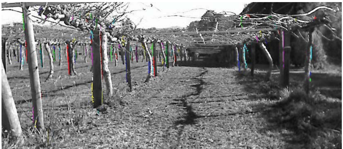
Figure 7-31: Edge identification from Sobel operator – where vertically spanning clusters of a targeted size are identified and drawn. Image converted to black and white to emphasise results.
