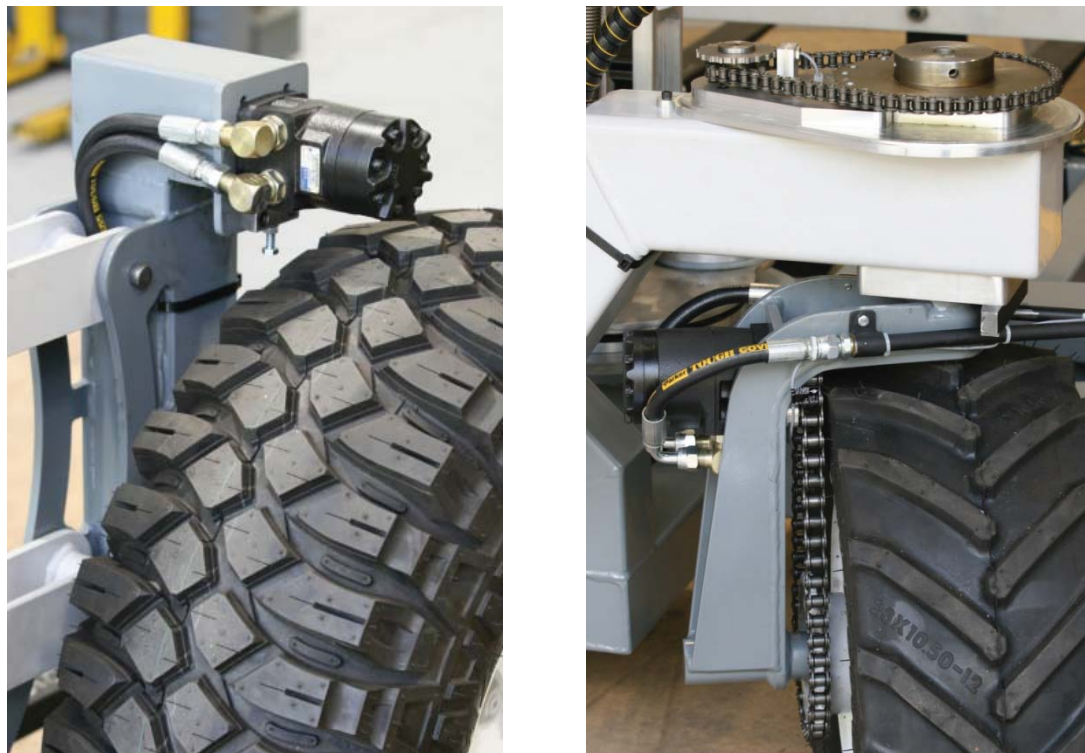
Figure 7-2: (Left) Rear wheel and drive assembly, (right) Front wheel trunnion and steering assembly
