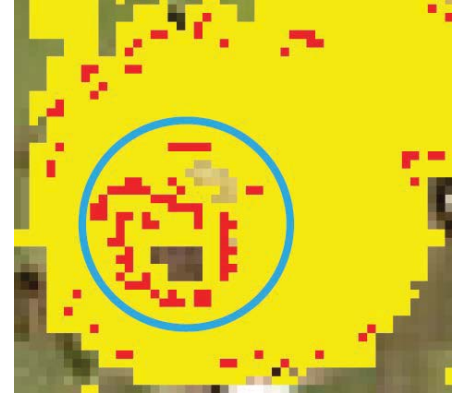
Figure 5-8: The search template (shown as a blue circle) at a positive fruit identification point
