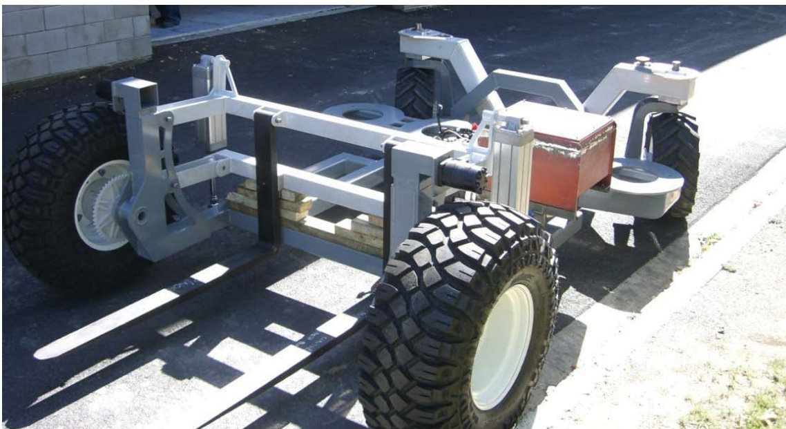
Figure 7-3: Assembled chassis after powder coating.
