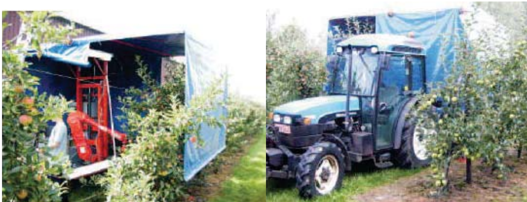
Figure 2-4 Robotic Apple Harvester (Baeten, et al., 2007)
