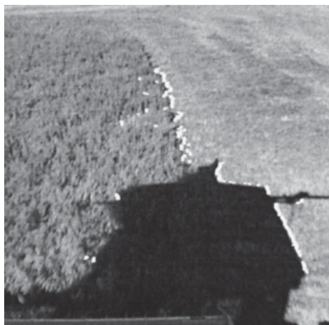
Figure 7-18: The Demeter System for visual navigation. The erroneous points from the tractor's shadow are shown (Pilarski, et al., 2002).
