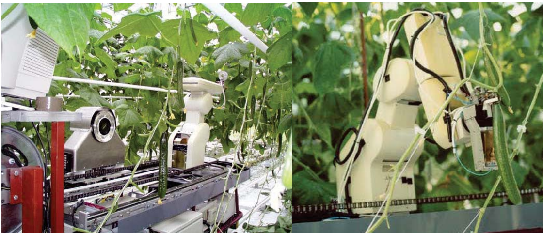
Figure 2-6 Cucumber harvesting robot (Van Henten, et al., 2003)
