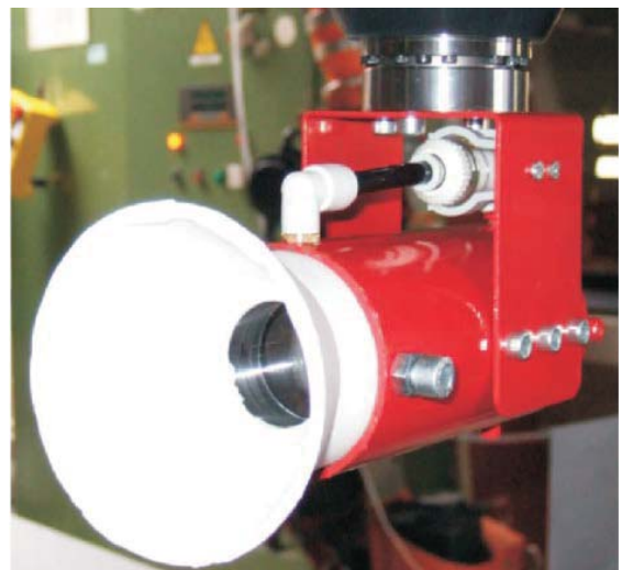
Figure 6-6: Apple harvesting robot silicone suction cup hand (Baeten, et al., 2007).
