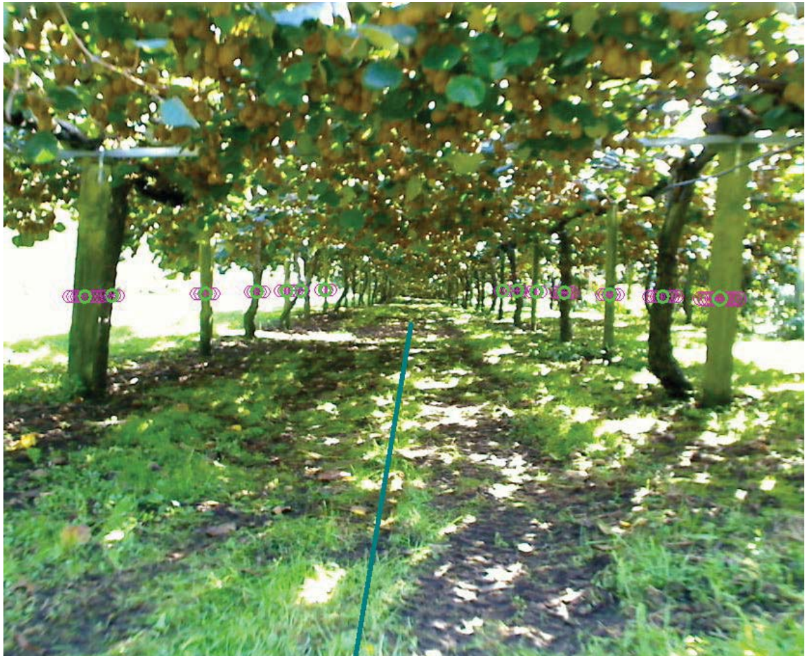
Figure 7-60: LIDAR determined row information superimposed onto a corresponding in-row image. The red circles represent the laser beams size and incident position at detection distance, where the green circles are the centre of the LIDAR data cluster, used to determine the driveline (superimposed in darker green)
