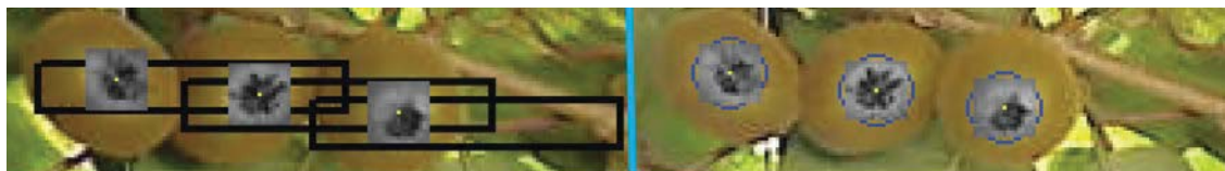
Figure 5-11: Stereo fruit matching. Result from finding the right hand fruit in the left image. The yellow dots, right hand image, are required to correspond to the same position in the left hand image.
