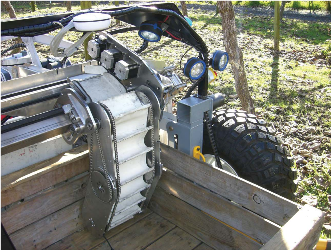
Figure 6-40: The bin filling arm on the AKH on-orchard
