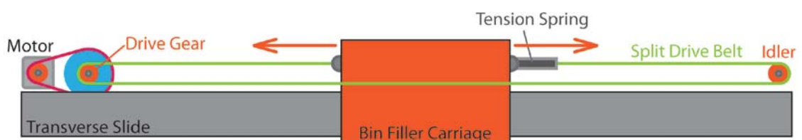
Figure 6-33: Axis One split belt drive
