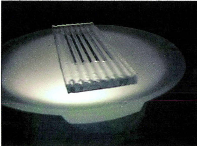
Figure 56 Oblique view of grooved-glass 'root chamber' glass microscope slide containing maize root segments
