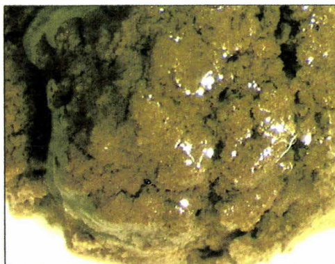
Figure 40 Permanent pasture artificial soil aggregate – no added nutrients, soil structure is slaking in 25% ethanol solution
