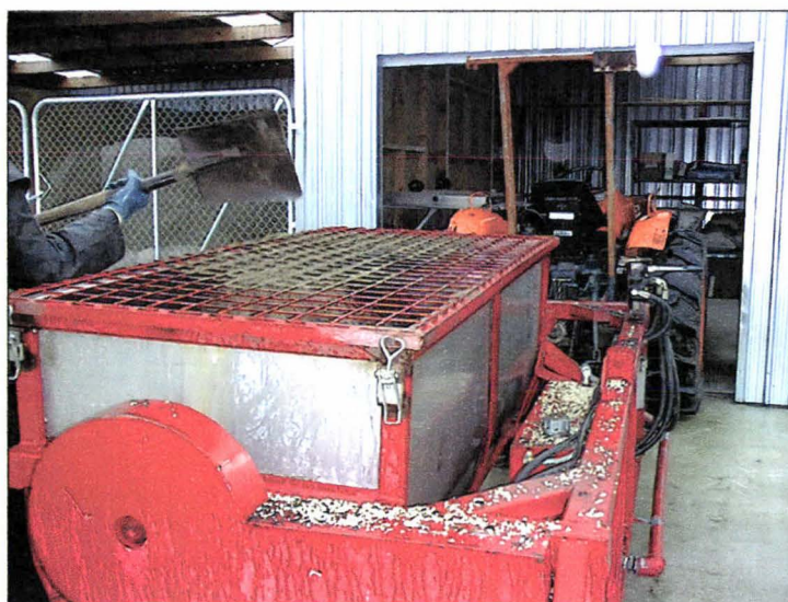
Figure 36 Steam pasteuriser used to pasteurise low-nutrient sandy silt-loam soil media for propagation of root-fungal bioassays of two pasture soils studied .
