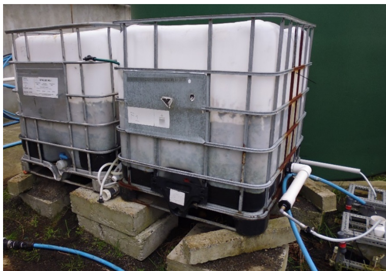
Figure 5.4 Pilot soil filters at Dannevirke STP (tipping bucket flow meters shown in the bottom right-hand corner).
