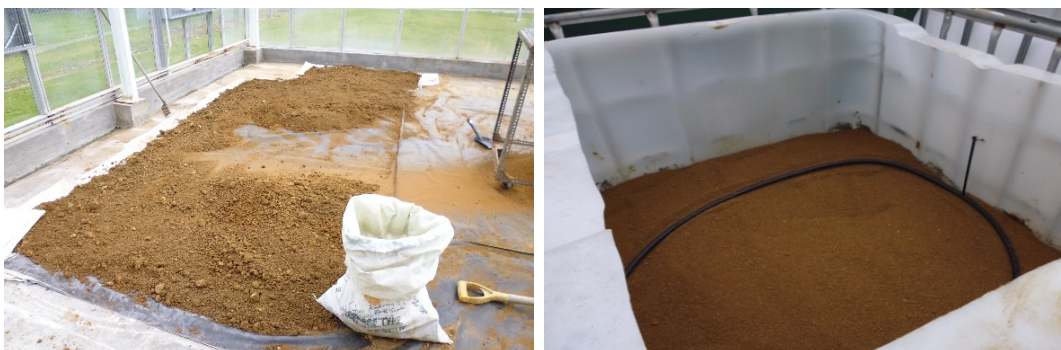
Figure 5.5 The Dannevirke STP pilot filter soil before (left) just prior to passing through a <4 mm sieve and reinstallation into a filter container after sieving (right).
