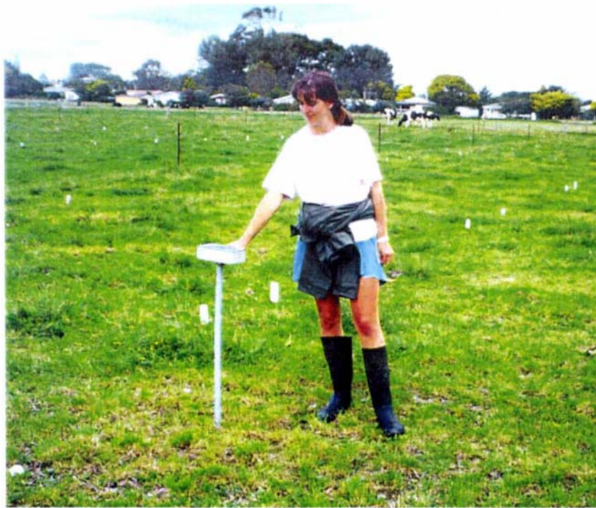
Plate 3.3. DRC technician estimating the post-grazing herbage mass of pasture with a capacitance probe in March 1998.
