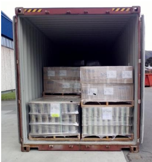
Figure 2.8 Cargo staked on pallets and secured with shrink wrap and unloaded by forklift (R. Hinz)
