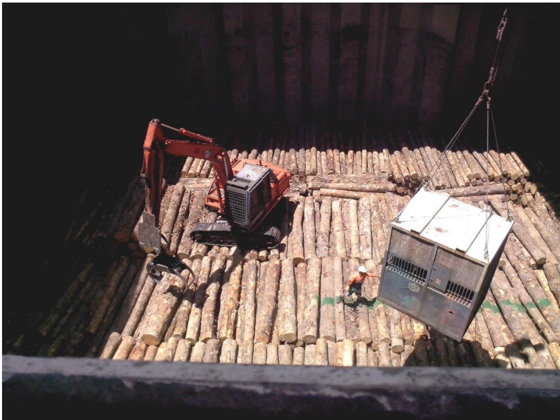
Figure 2.19 Previously fumigated logs being loaded into the hold of the ship. Logs are getting spray painted to mark which part of the cargo is getting unloaded at the first port before transiting to the next port for unloading (R. Hinz)
