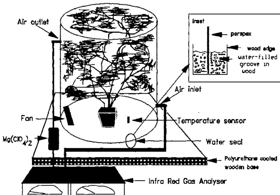
Figure 4.1 Closed system design for plant respiration studies.
