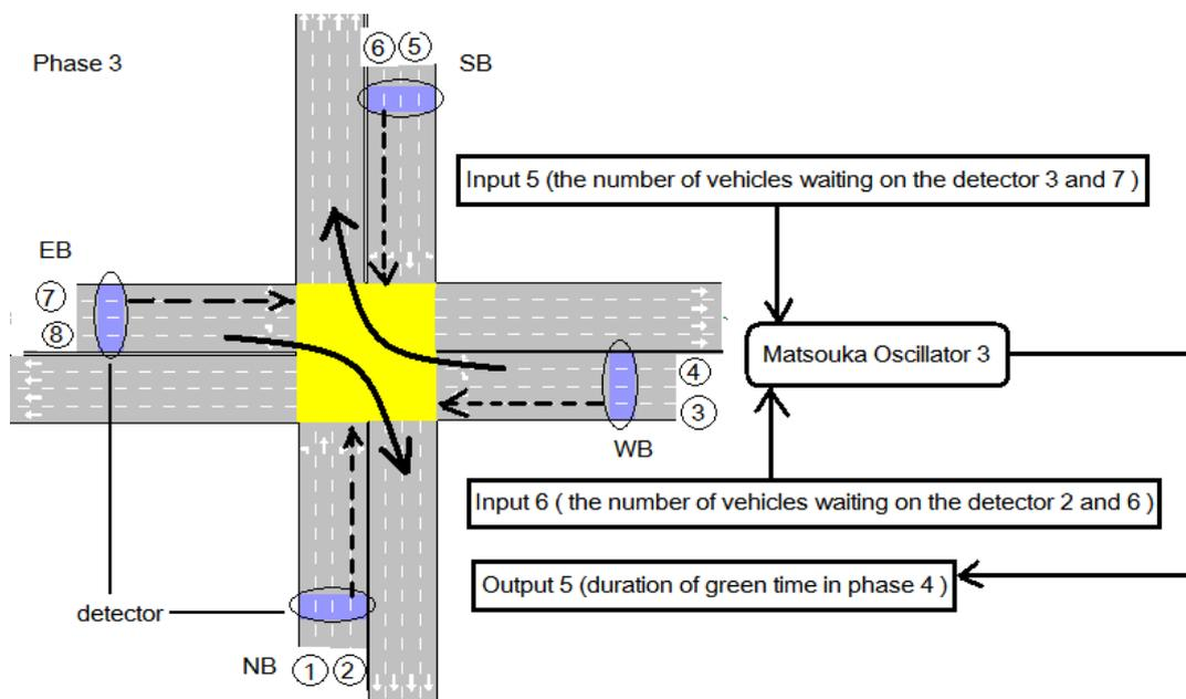
Figure 4-8 The graph of phase 3 (Matsuoka Oscillator 3 is implemented).
