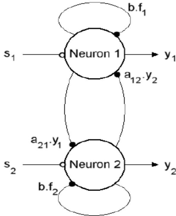
Figure 3-2 Matsuoka Oscillator with two neurons. (Taken from Bouhet et al, 2007).
