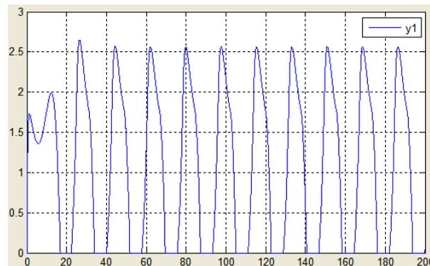
Figure 3-4 The stationary periodic output of Matsuoka Oscillator
