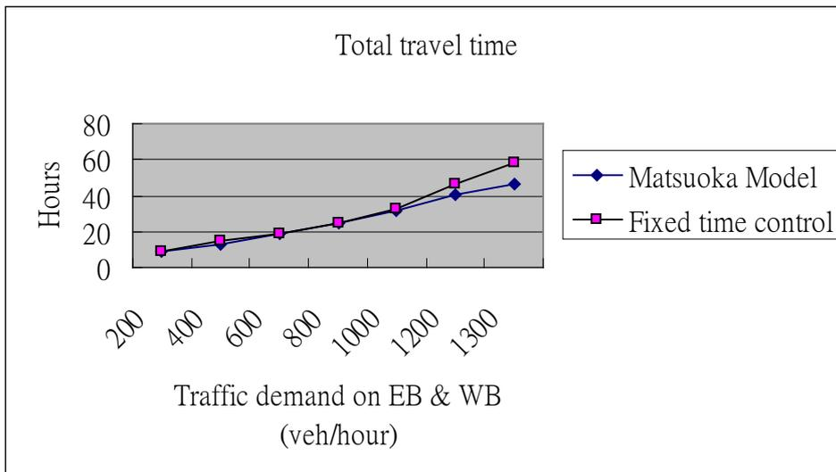
**Figure 4-24 Comparison of total travel time (Matsuoka model v.s. Fixed time control).**
