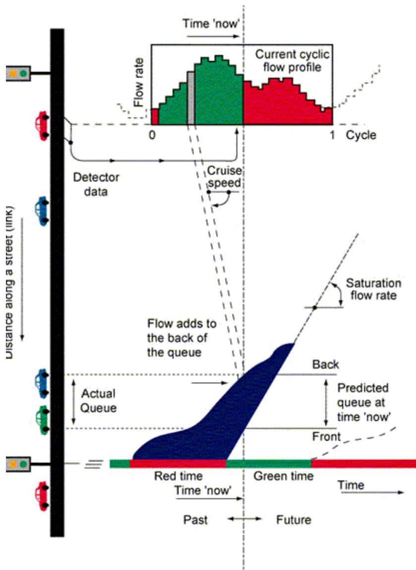
Figure 2-1 The operation of SCOOT model (taken from <http://www.scoot-utc.com/DetailedHowSCOOTWorks.php?menu=Technical>)
