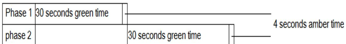
**Figure 3-7** The table of fixed cycle time
