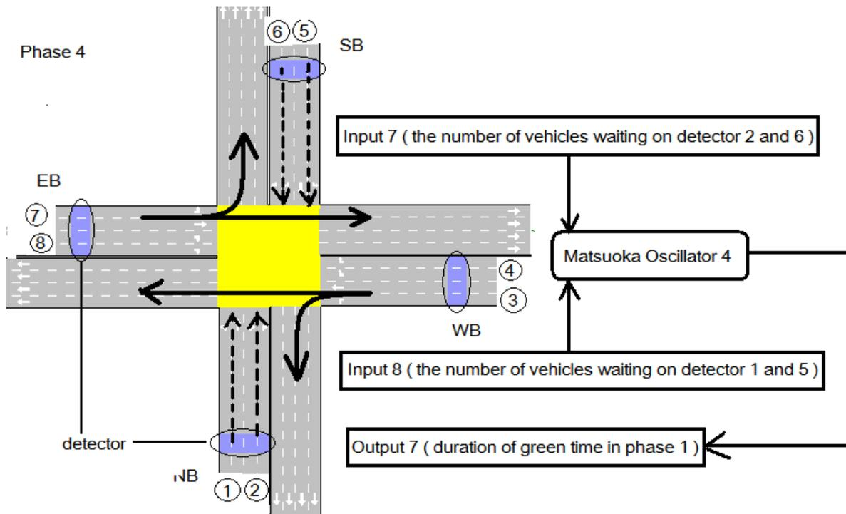
Figure 4-9 The graph of phase 4 (Matsuoka Oscillator 4 is implemented).
