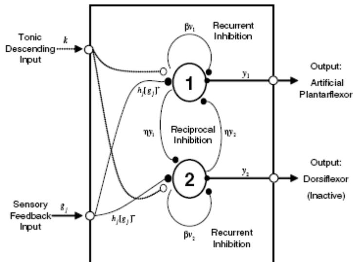
Figure 2-10 Artificial neural oscillator schematic (Taken from Evan et al, 2008).
