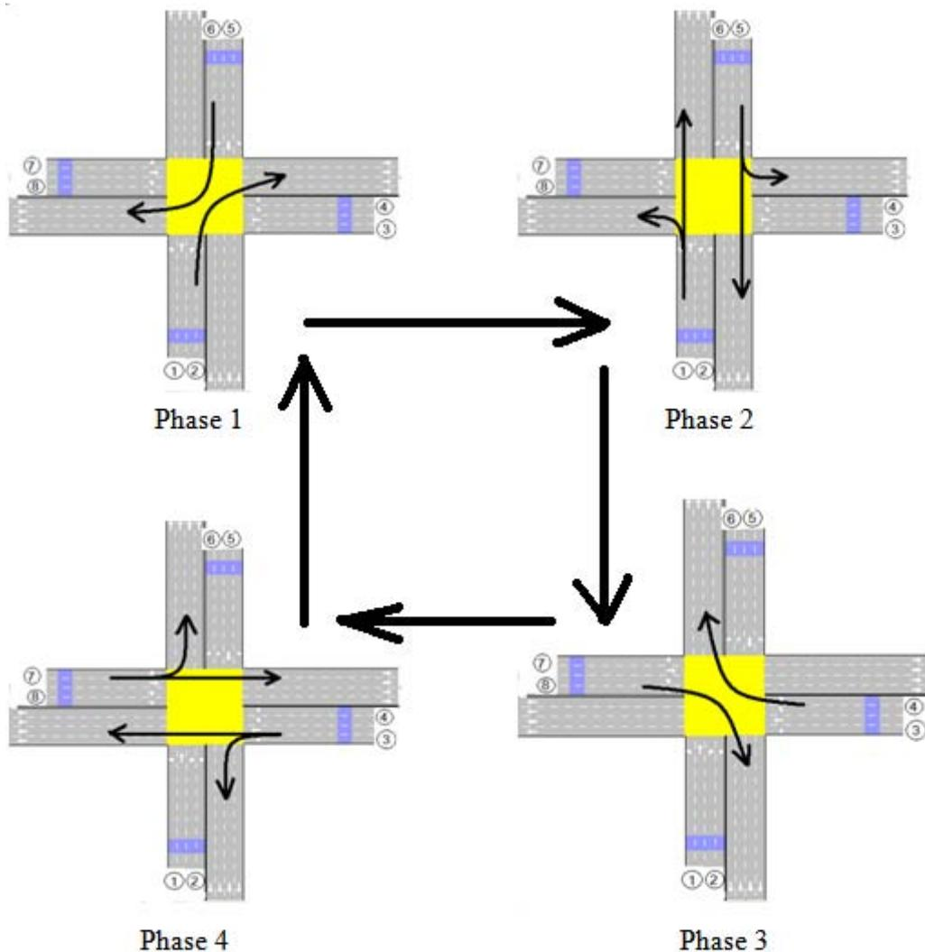
Figure 4-1 An isolated intersection with four phases
