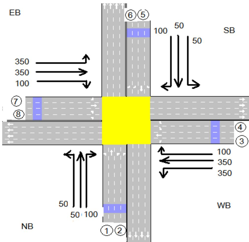
Figure 4-10 An isolated intersection with an unbalanced traffic demand scenario
