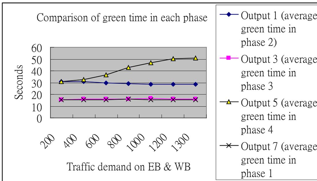
Figure 4-19 The comparison of green time in each phase.
