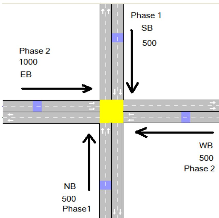
Figure 3-26 Unbalance traffic demand scenario with increasing travel volume on the EB.
