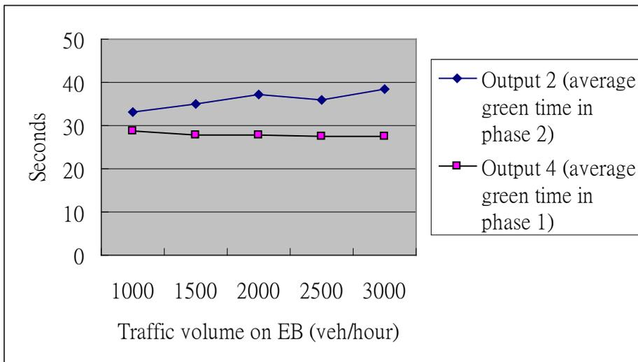
**Figure 3-29 The average green time in phase 1 and phase 2 with different total traffic demand scenarios.**
