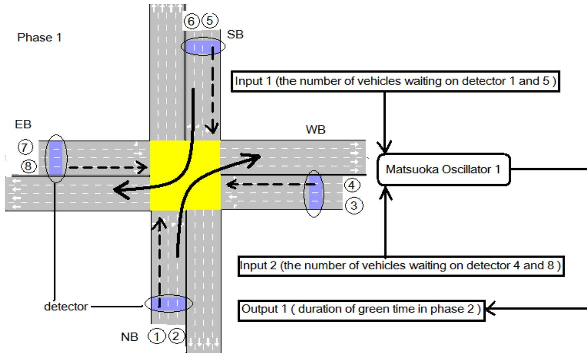
Figure 4-6 The graph of phase 1 (Matsuoka Oscillator 1 is implemented).
