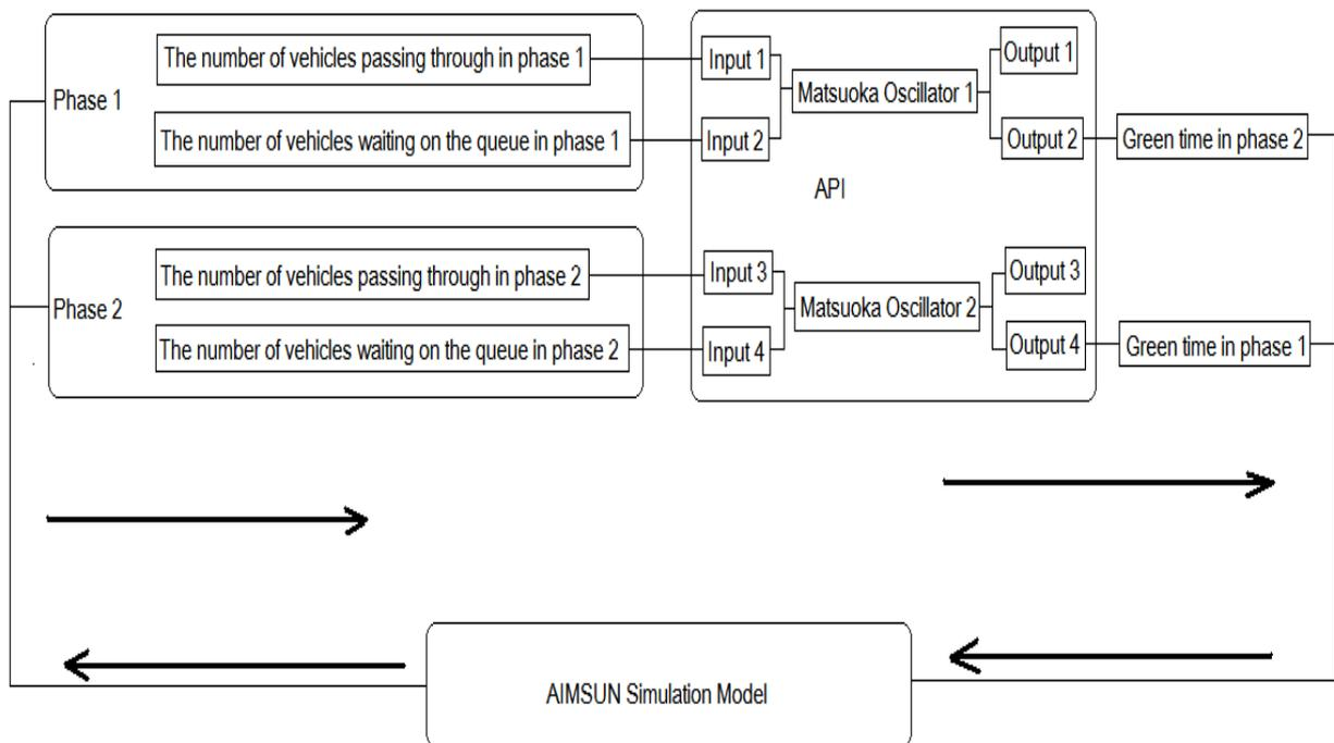
Figure 3-12 The structure of traffic system with two Matsuoka Oscillators.
