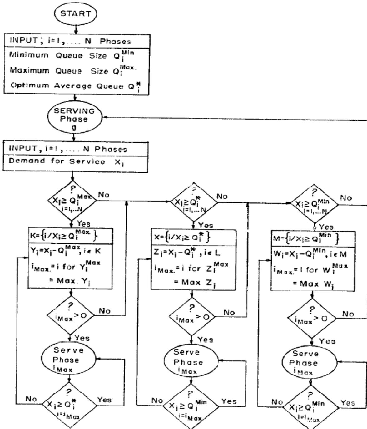
Figure 2-6 A Simplified State Dependent-Server-Vacation Signal Timing (Taken from Anthony et al, 1986)
