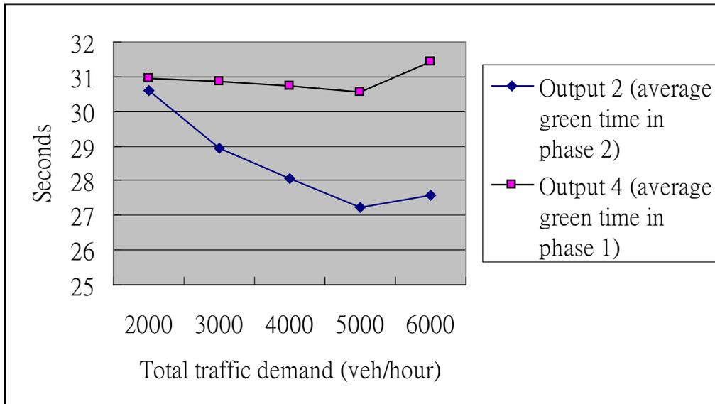
**Figure 3-22 The average green time in phase 1 and phase 2 with different total traffic demand scenarios.**
