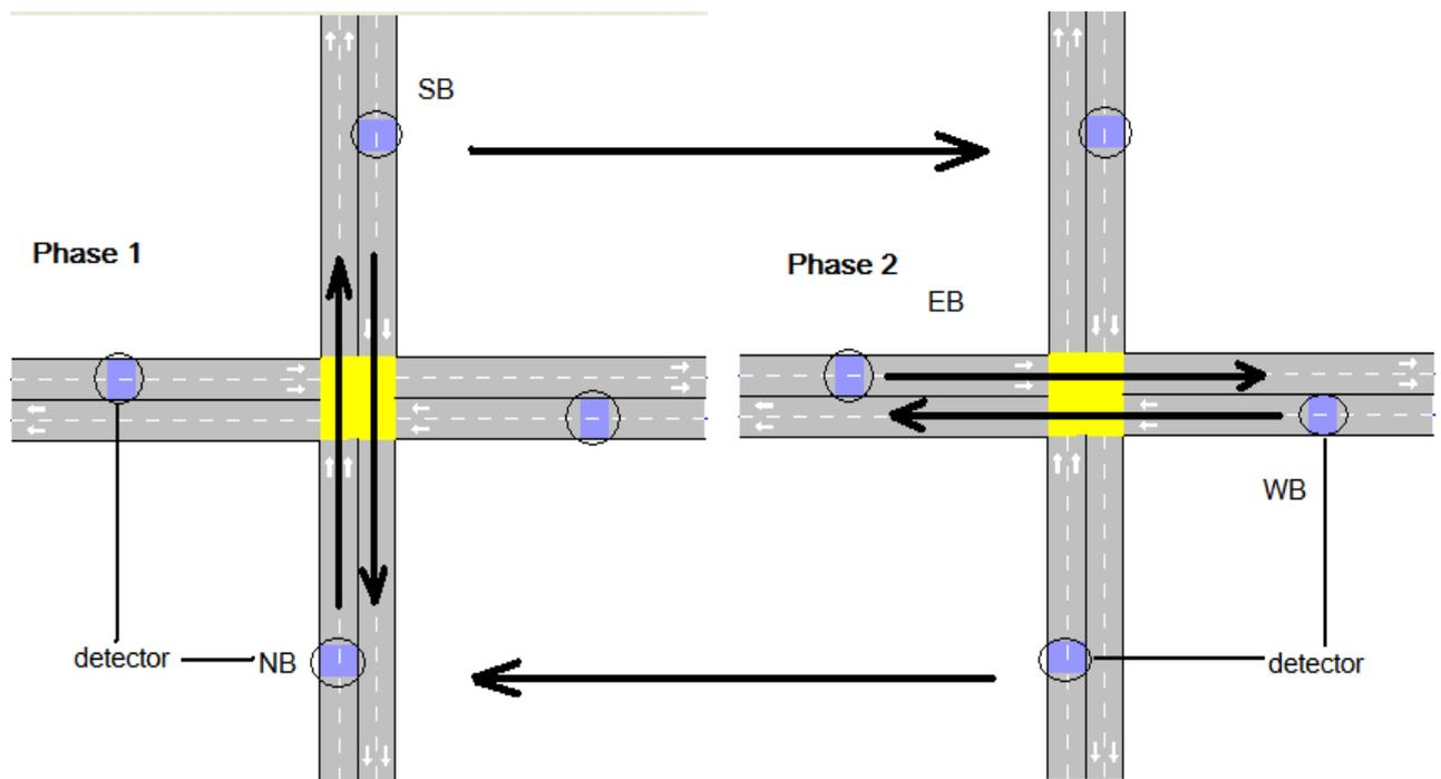
Figure 3-14 An insulated intersection with two phases
