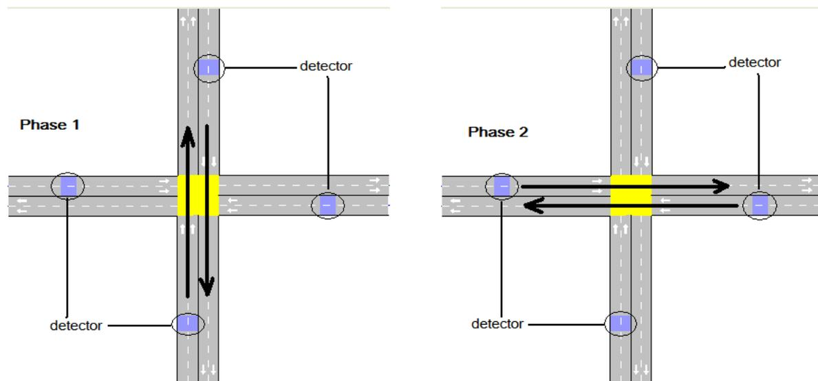
Figure 3-1 The intersection with two phases
