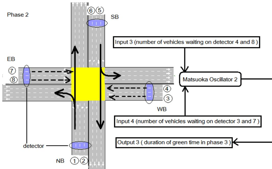
Figure 4-7 The graph of phase 2 (Matsuoka Oscillator 2 is implemented).
