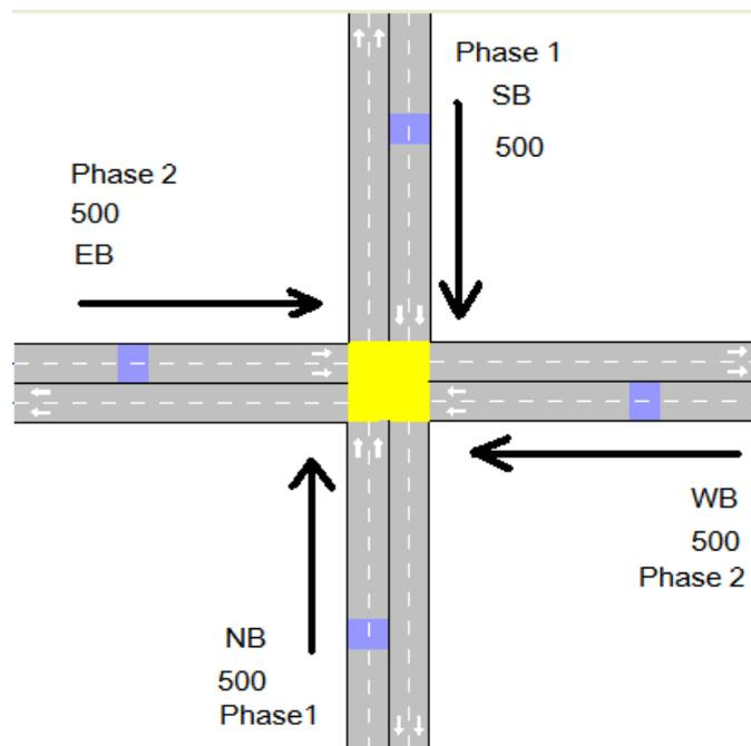
Figure 3-19 The simulated isolated intersection with same traffic volume scenario
