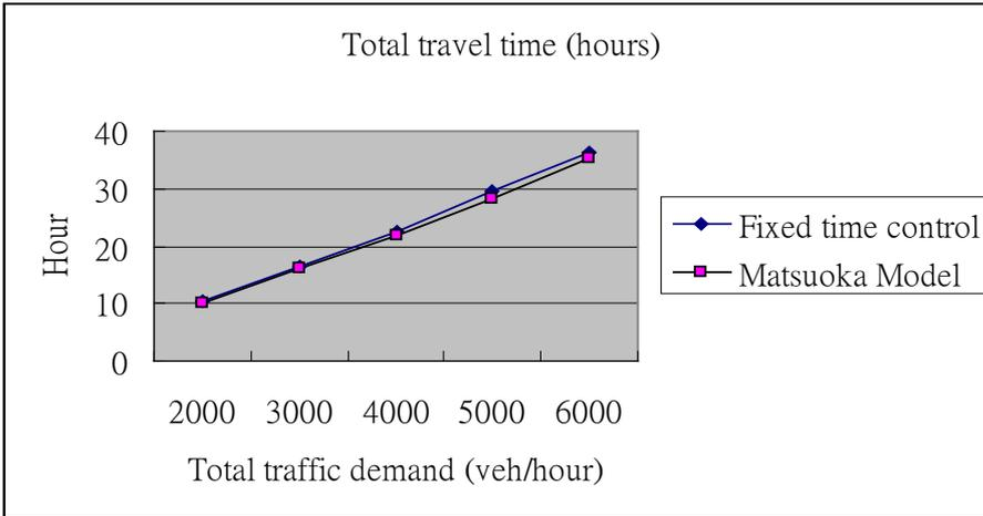
**Figure 3-23 Comparison of total travel time (Matsuoka model v.s. Fixed time control).**
