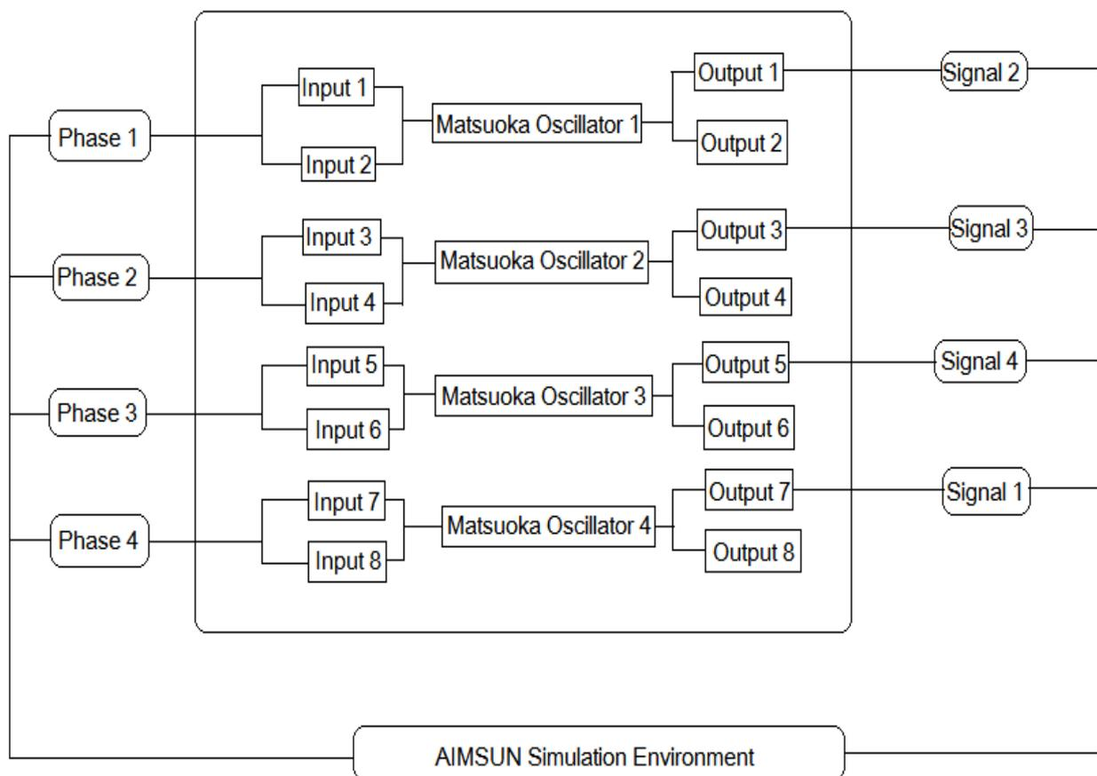
Figure 4-5 The structure of the four-phase intersection with four Matsuoka Oscillators
