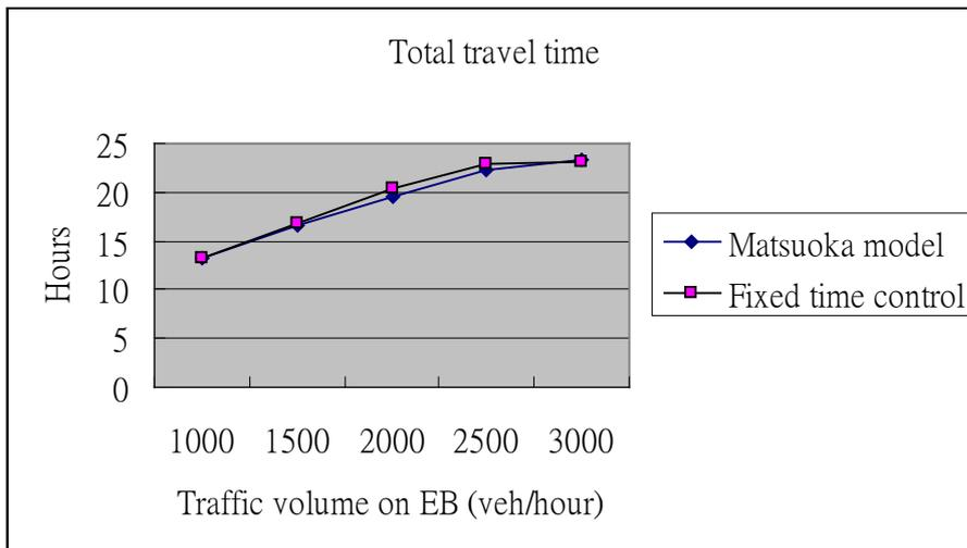
**Figure 3-34 Comparison of total travel time (Matsuoka model v.s. Fixed time control).**
