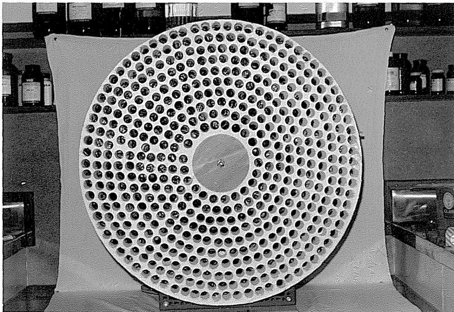
Figure 8. Rotating wheel for coleoptile bioassays
