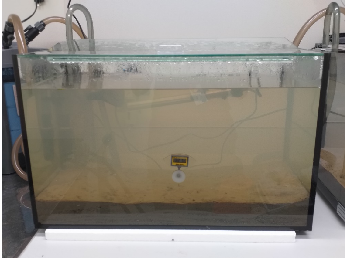
Figure 53: What the tanks looked like after adding sediment and being filled with a mixture of chlorine-free filtered RO water and stream water. The water began to look much clearer 24 hours after this photo was taken, as the fine sediment suspended in the water column settled. Following this period, the filters were switched on and left on for the microbiota to develop and mature.
