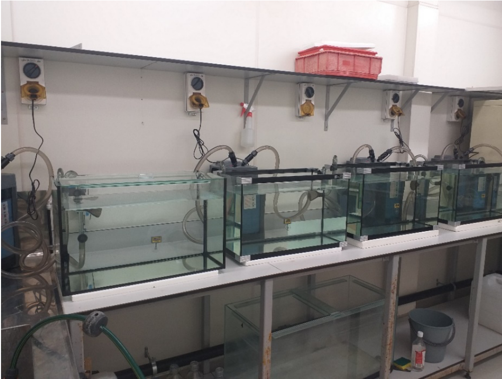
Figure 48: Aquarium and filtration set up in the Freshwater Laboratory. The four aquariums were set up next to each other on a lab bench, with an external canister filter located behind each.
