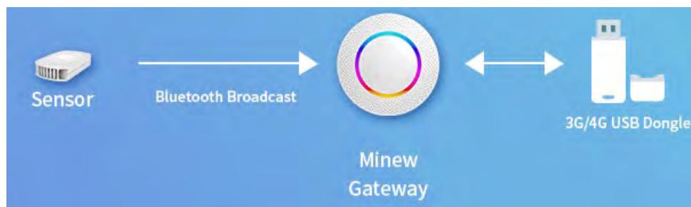
FIGURE 4.12: Minew Sensor and Gateway Data Flow Process
