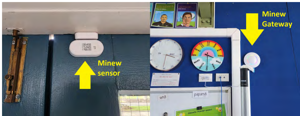
FIGURE 4.11: Minew Sensor (left) and Gateway Instrument (right)
