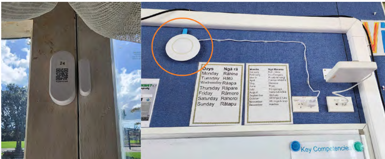
FIGURE 4.9: Placement of sensors
