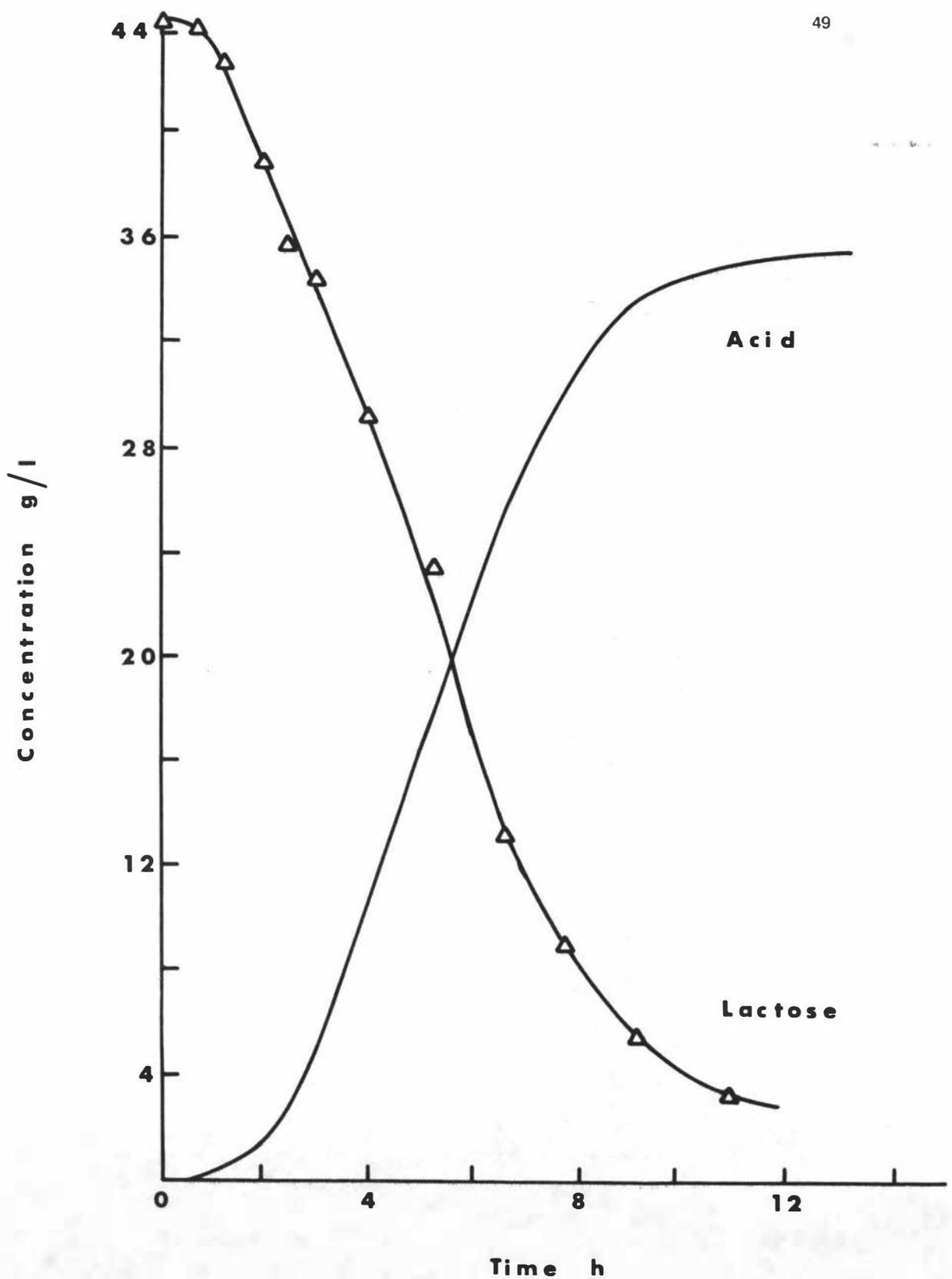
Figure 4.4 Acid and lactose concentrations during the batch culture of whey. Whey 75 g/l with supplementary nutrients, pH5.5, 46°C.
