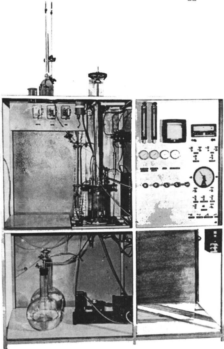
Figure 3.2 The culture vessel and controls.
