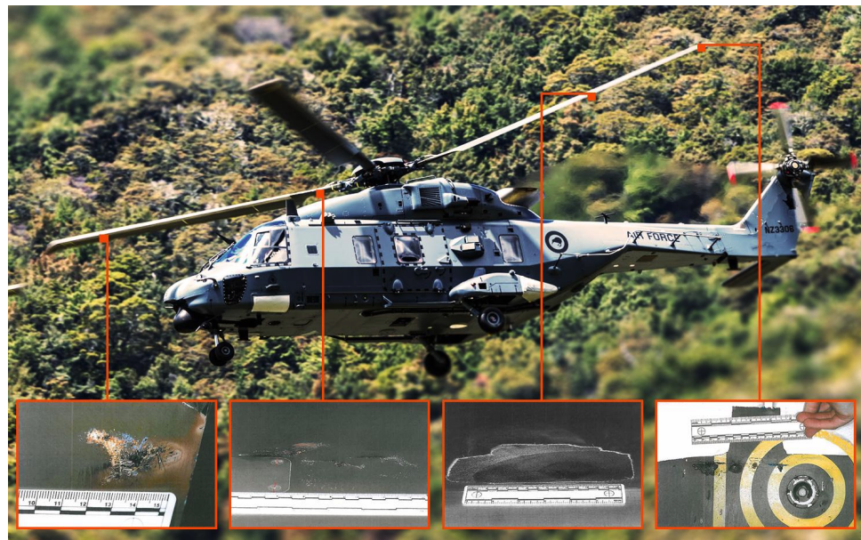
Figure 8 Lightning Strike Damage to NH90 378
