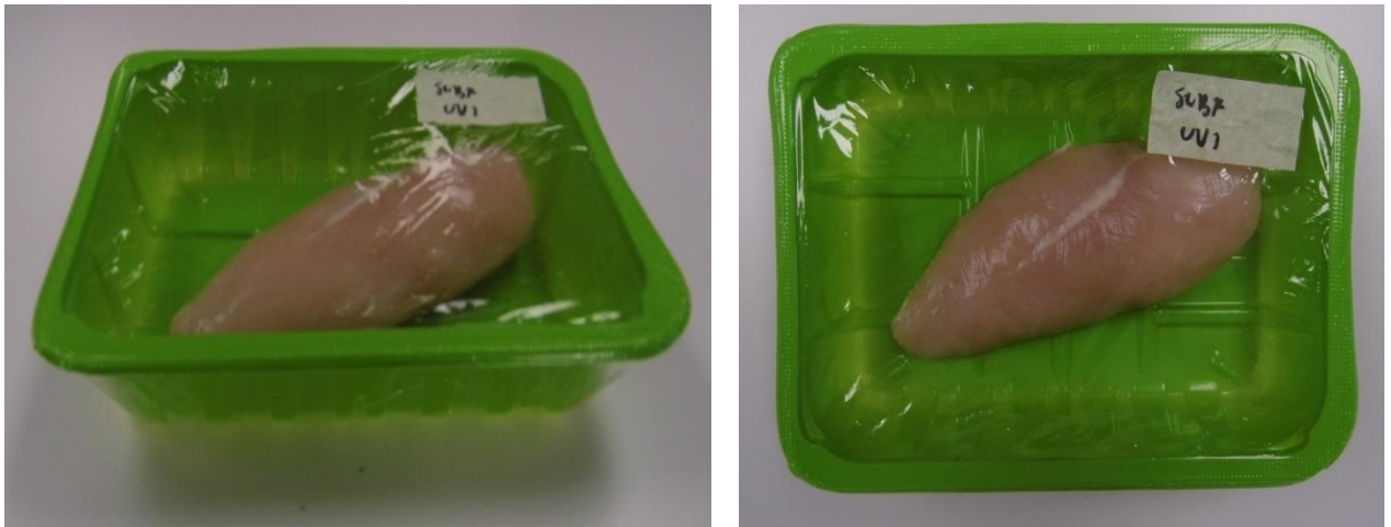
Figure 3.5. Fresh chicken samples packed in recycled polyethylene terephthalate (RPET) tray with a polyethylene sealant layer.
