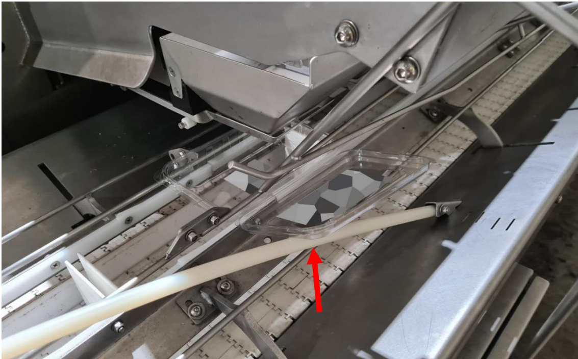
Fig. 46 The punnet, which would be full of berries, at the start of the process of having its lid flipped over by a nylon rail.
