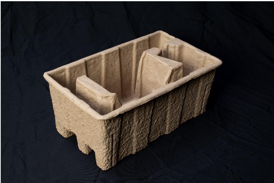
Fig. 28. A moulded pulp packaging item. Note the smoother texture inside where the pulp was pulled onto the mesh mould with a vacuum.
