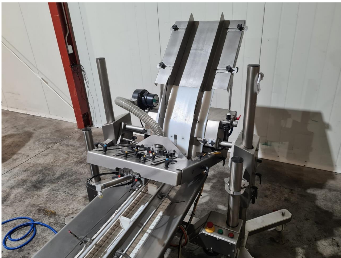
Fig. 41. magazine and dispenser mechanism for empty punnets, with a part of the conveyor that carries the punnets visible at bottom right.
