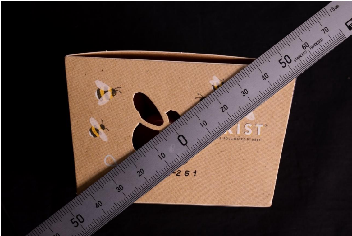
Fig. 17. Beekist paperboard carton with ruler in MM to display the size of the smallest cut-out they use.
