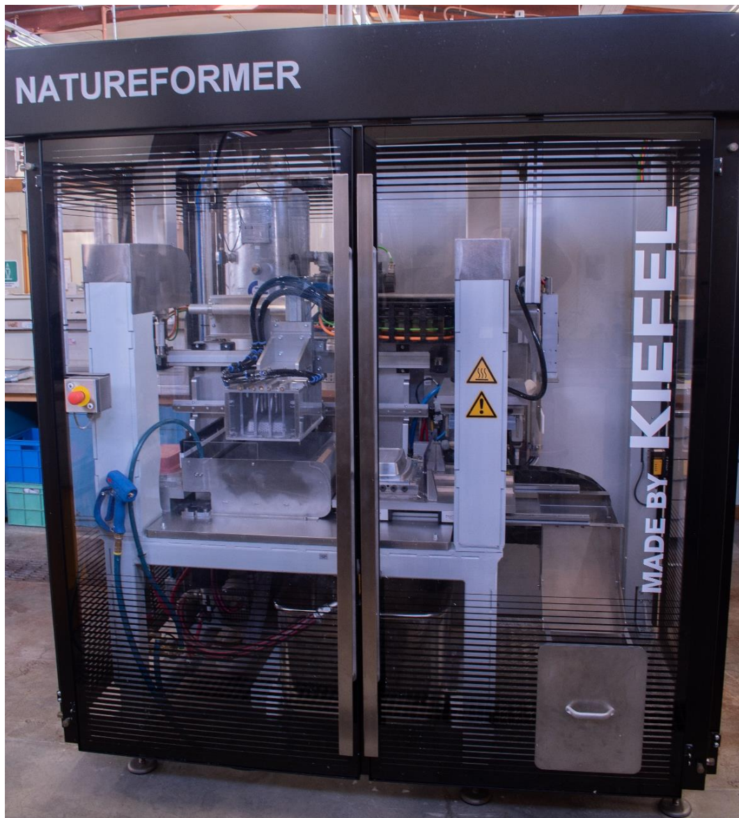
Fig. 31. Kiefel Natureformer, a small-scale thermoforming machine.
