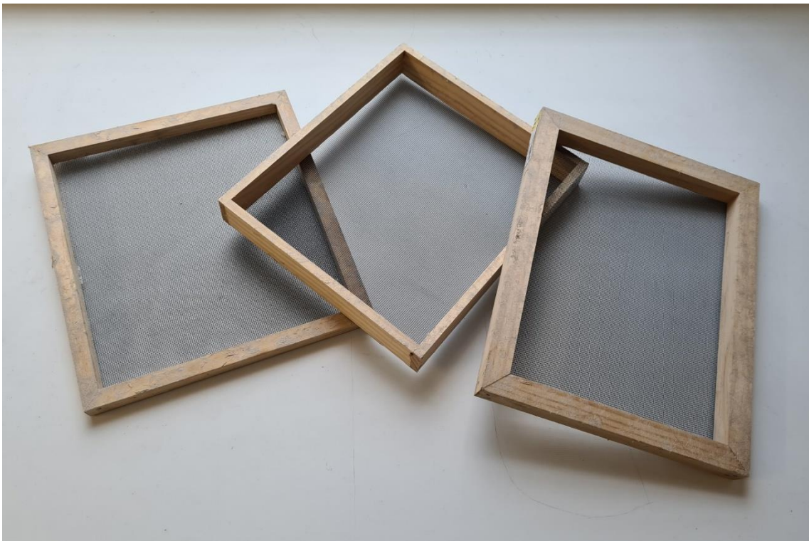
Fig. 52. Mould and deckles used in paper making, made by me using screen door mesh and pine.
