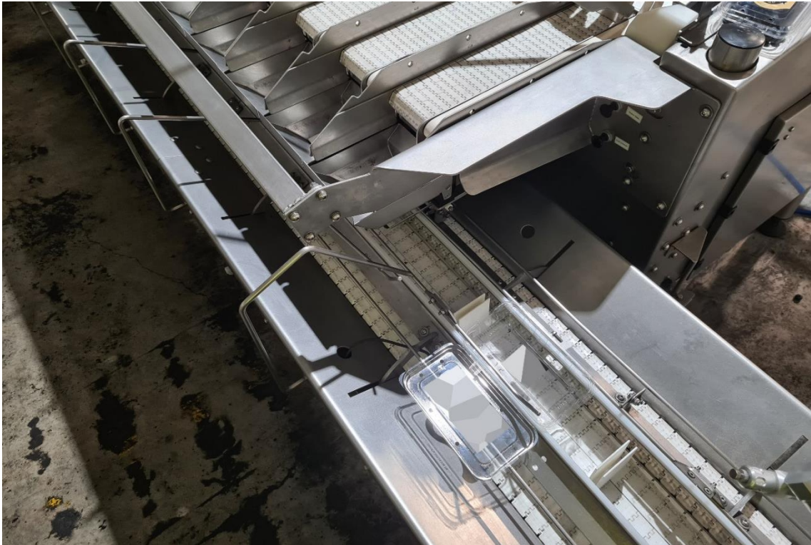
Fig. 43 The empty punnet, as if it is about to go under the weighing gates.
