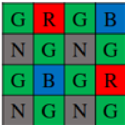
Figure 31: The ideal RGB-NIR MSFA. Proven by Monno et al. in [1] [Reproduced by permission of IEEE, Copyright © 2019]
