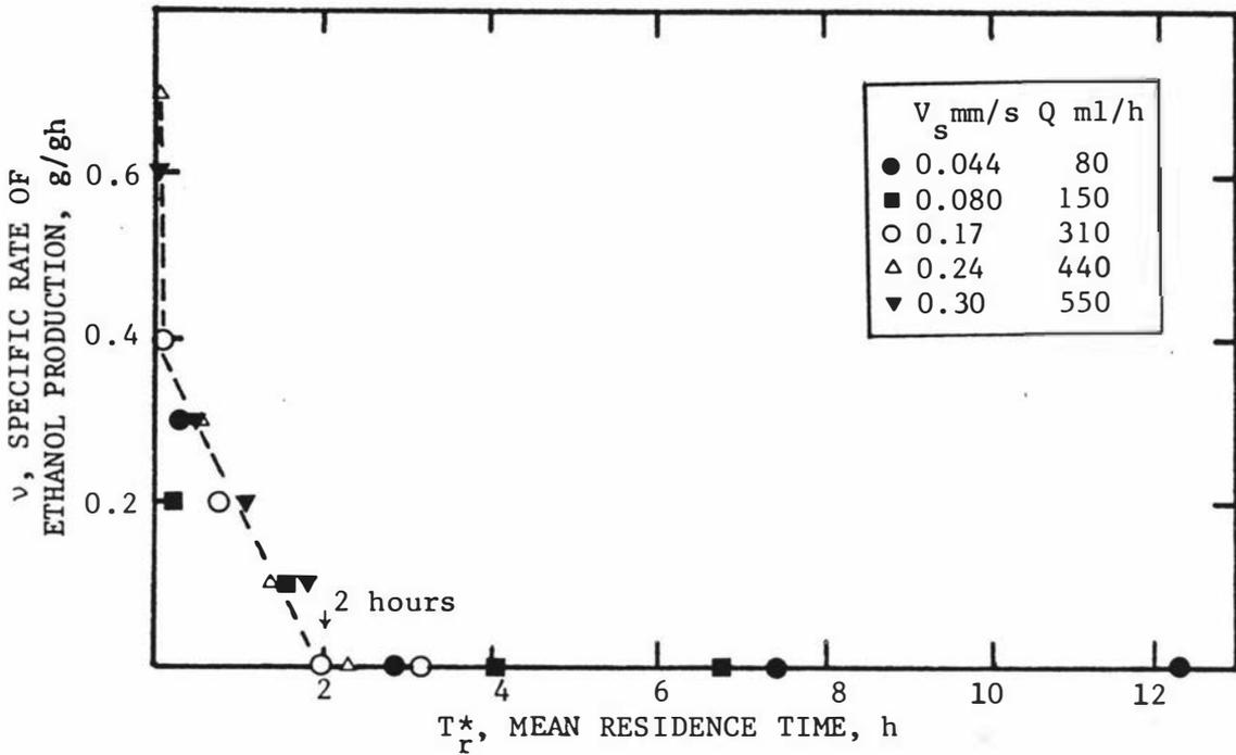
Fig.4.17 Specific rate of ethanol production vs mean residence time at various superficial liquid velocities.
