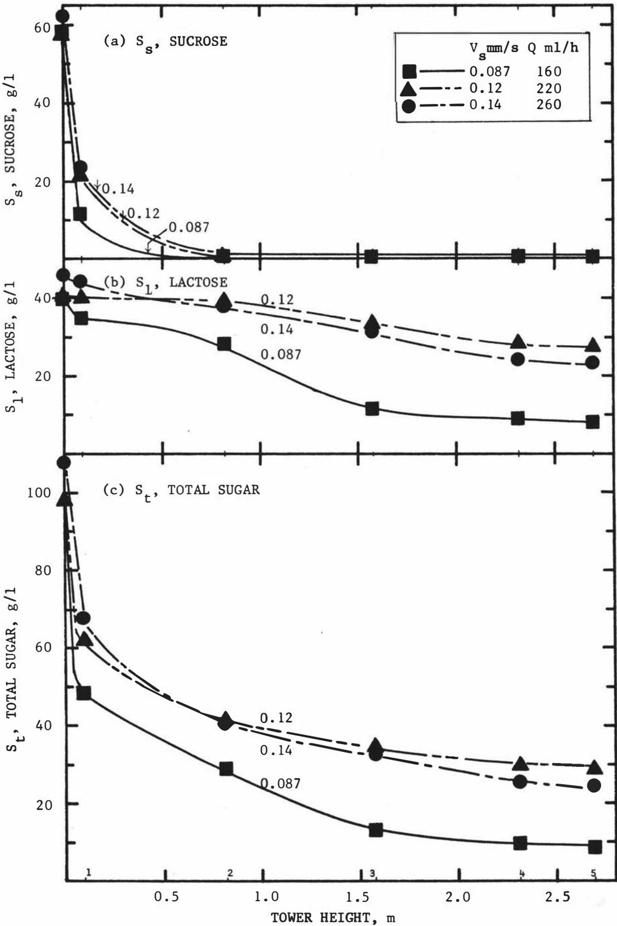
Fig. 5.1 Sugar concentration vs tower height at various superficial liquid velocities. (a) Sucrose , (b) Lactose , (c) Total sugar.
