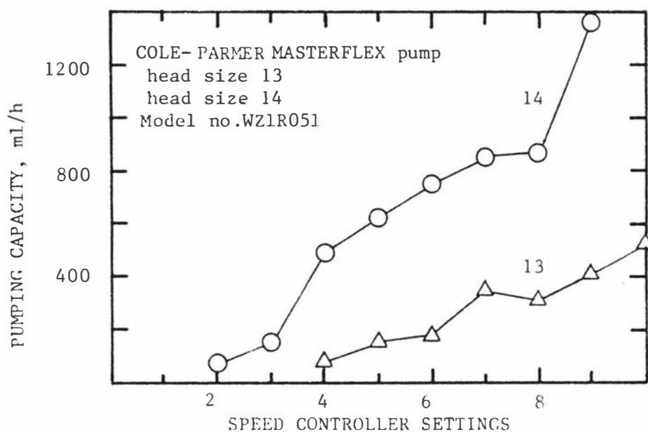
Fig.A.1 Pump capacity curves for 25 mm $\phi$  tower fermenter.
