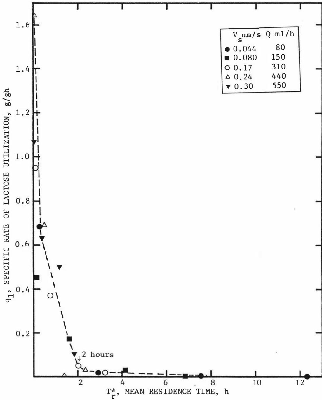
Fig.4.16 Specific rate of lactose utilization vs mean residence time at various superficial liquid velocities.
