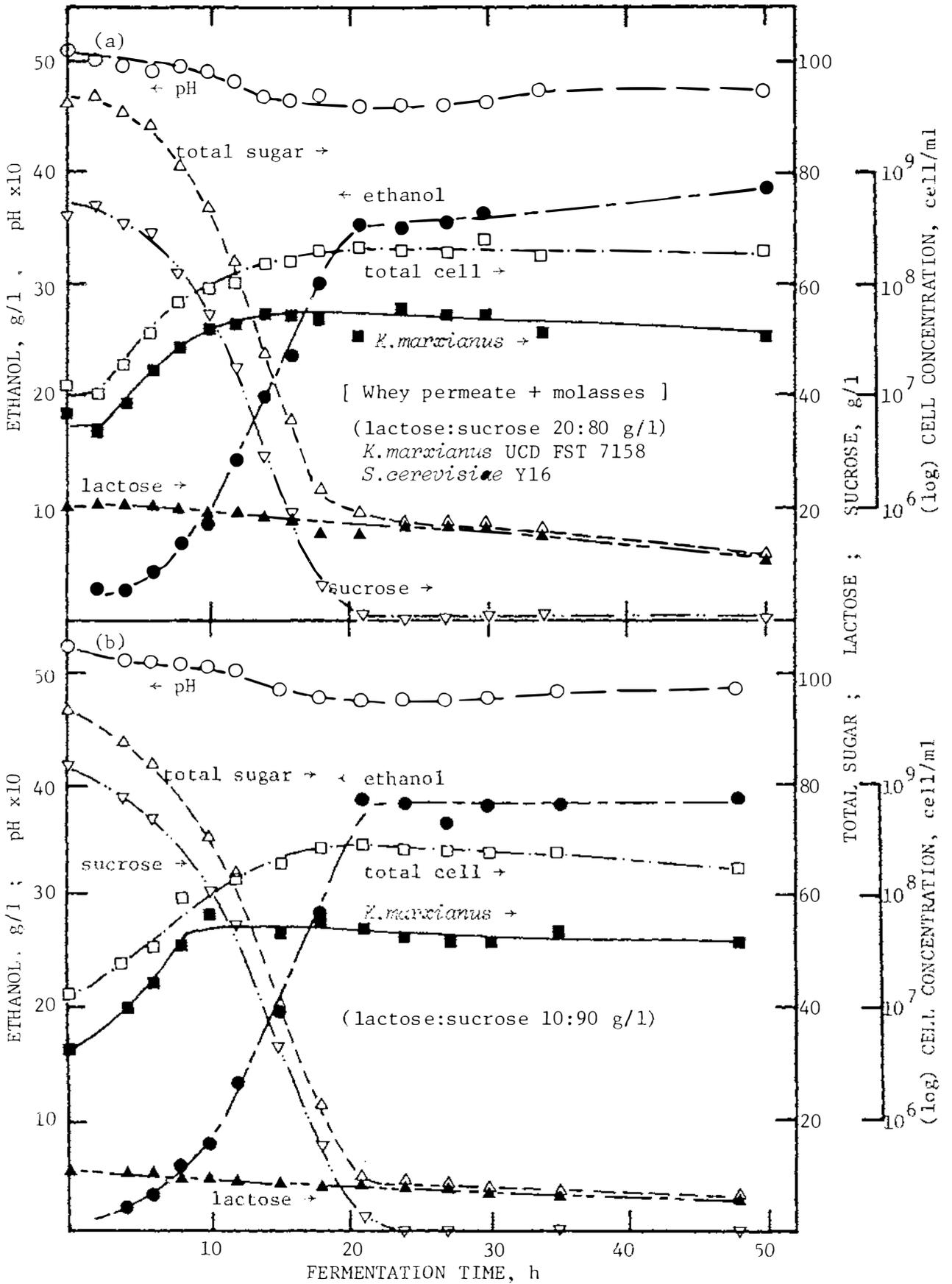
Fig. 7.3 Batch fermentation of whey permeate enriched with molasses using lactose : sucrose ratio of (a) 20:80, and (b) 10:90 g/l by *K.marxianus* and *S.cerevisiae*.
