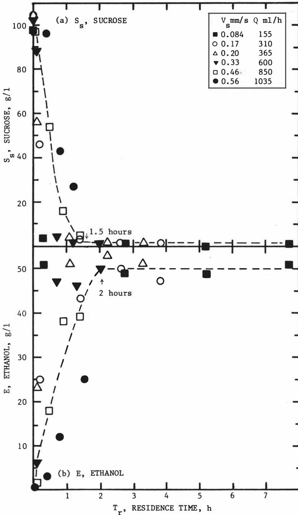
Fig.C.7 (a) Sucrose and (b) ethanol concentrations vs residence time at various superficial liquid velocities.
