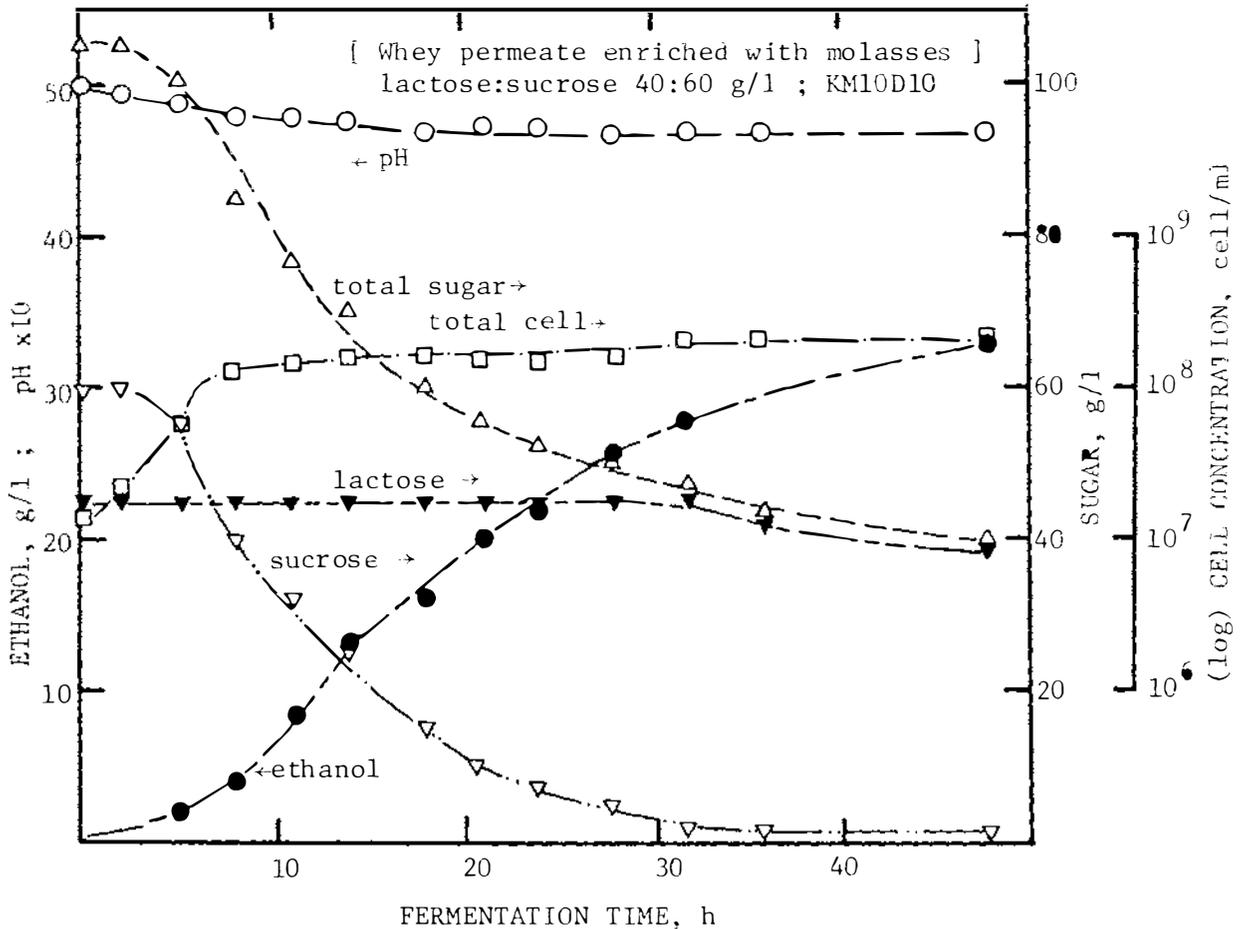
Fig.7.7 10 litre batch fermentation of whey permeate enriched with molasses by KM10D10 (lactose:sucrose 40:60 g/l).
