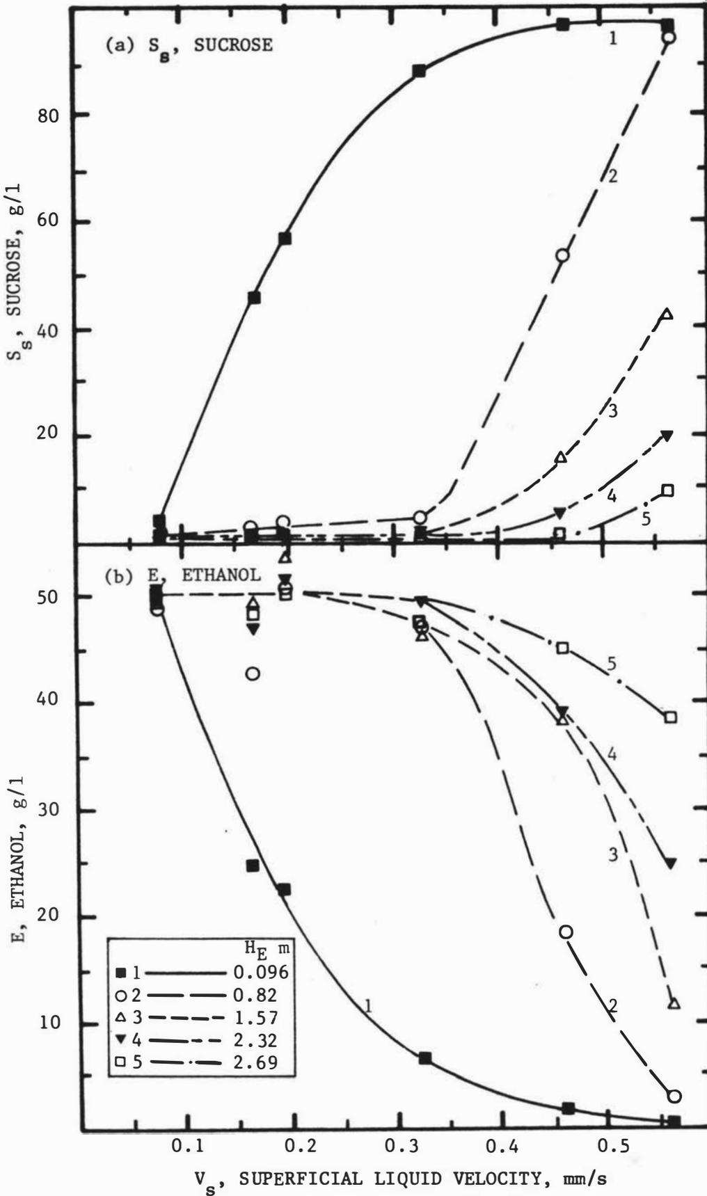
Fig. C.10 (a) Sucrose and (b) ethanol concentrations vs superficial liquid velocity at various tower heights.
