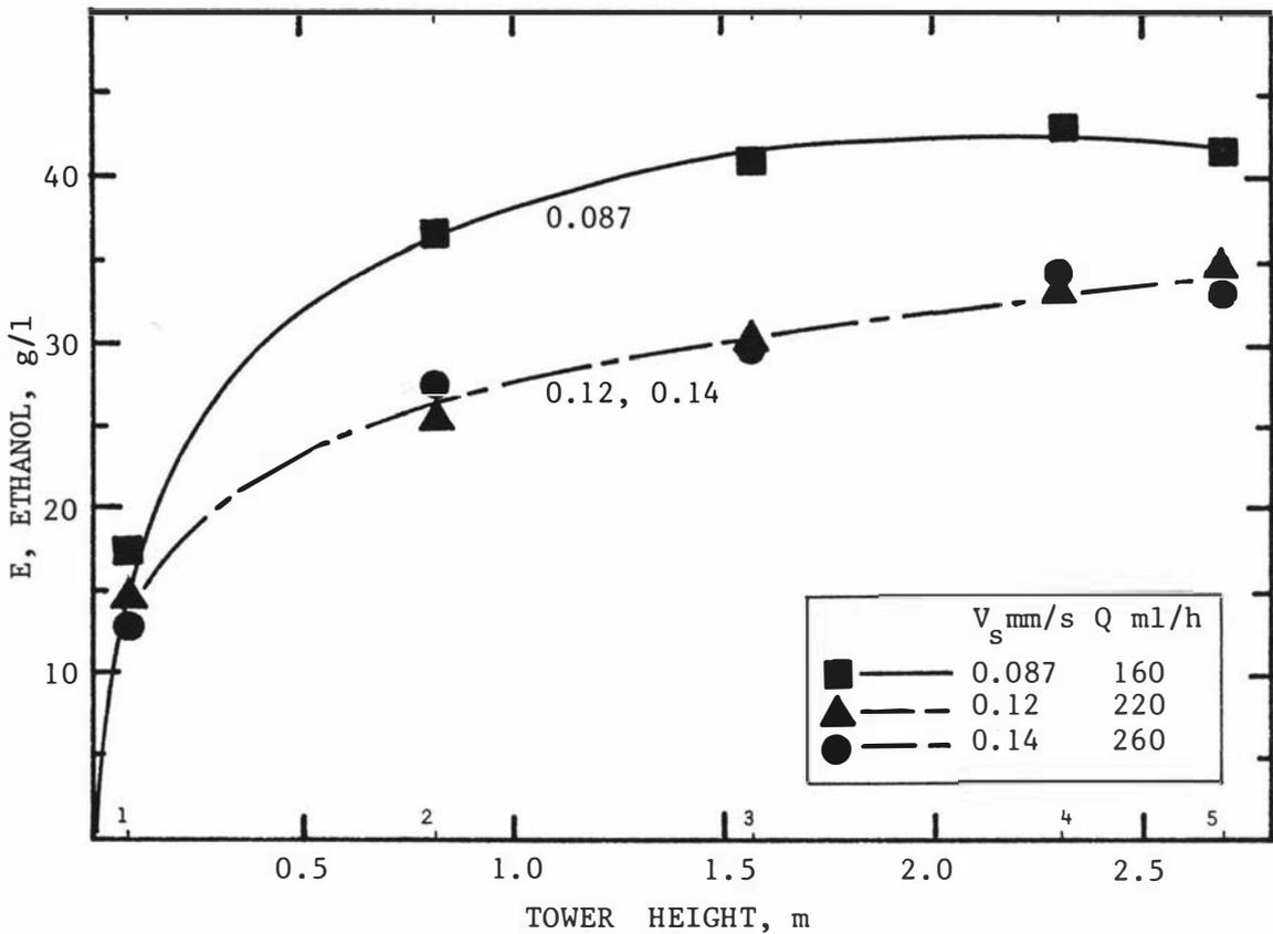
Fig. 5.4 Ethanol concentration vs tower height at various superficial liquid velocities.
