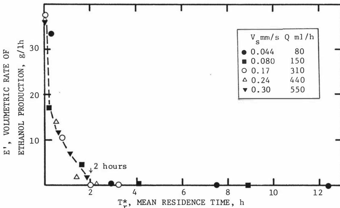
Fig.4.15 Volumetric rate of ethanol production vs mean residence time at various superficial liquid velocities.
