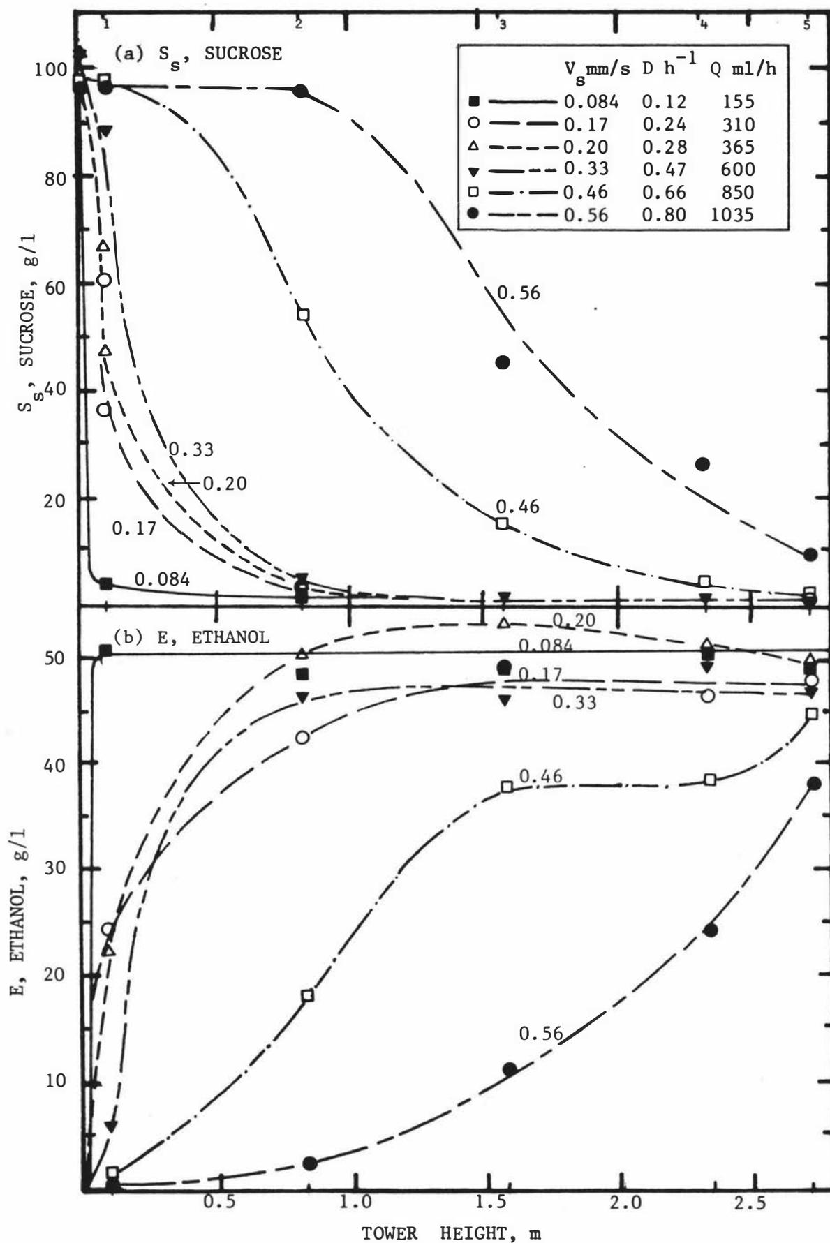
Fig.C.1 (a) Sucrose and (b) ethanol concentrations vs tower height at various superficial liquid velocities.
