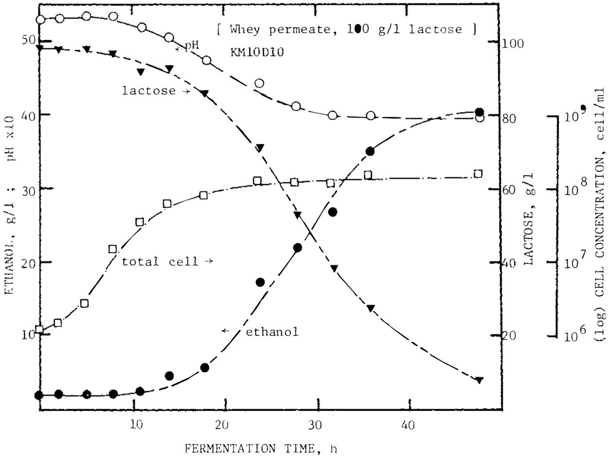
Fig.7.6 10 litre batch fermentation of whey permeate (100 g/l lactose) by KM10D10.
