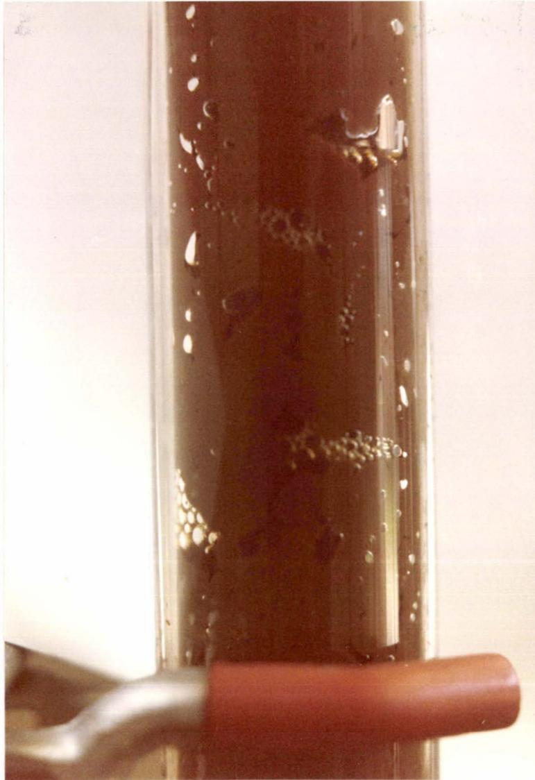
Fig. 5.9 Channelling inside the tower during mixed culture and mixed substrate tower fermentation.
