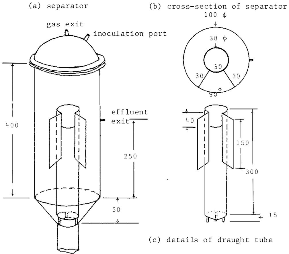
All dimensions are in mm.  $\phi$  = internal diameter
