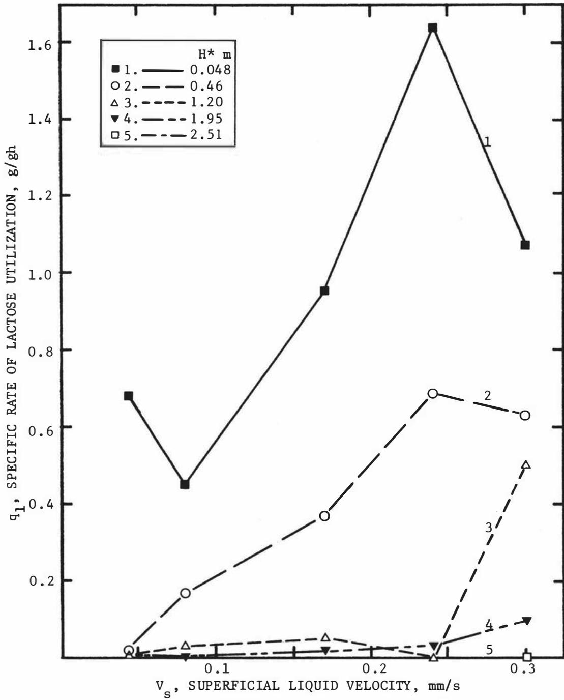
Fig.4.21 Specific rate of lactose utilization vs superficial liquid velocity at various mean tower heights.
