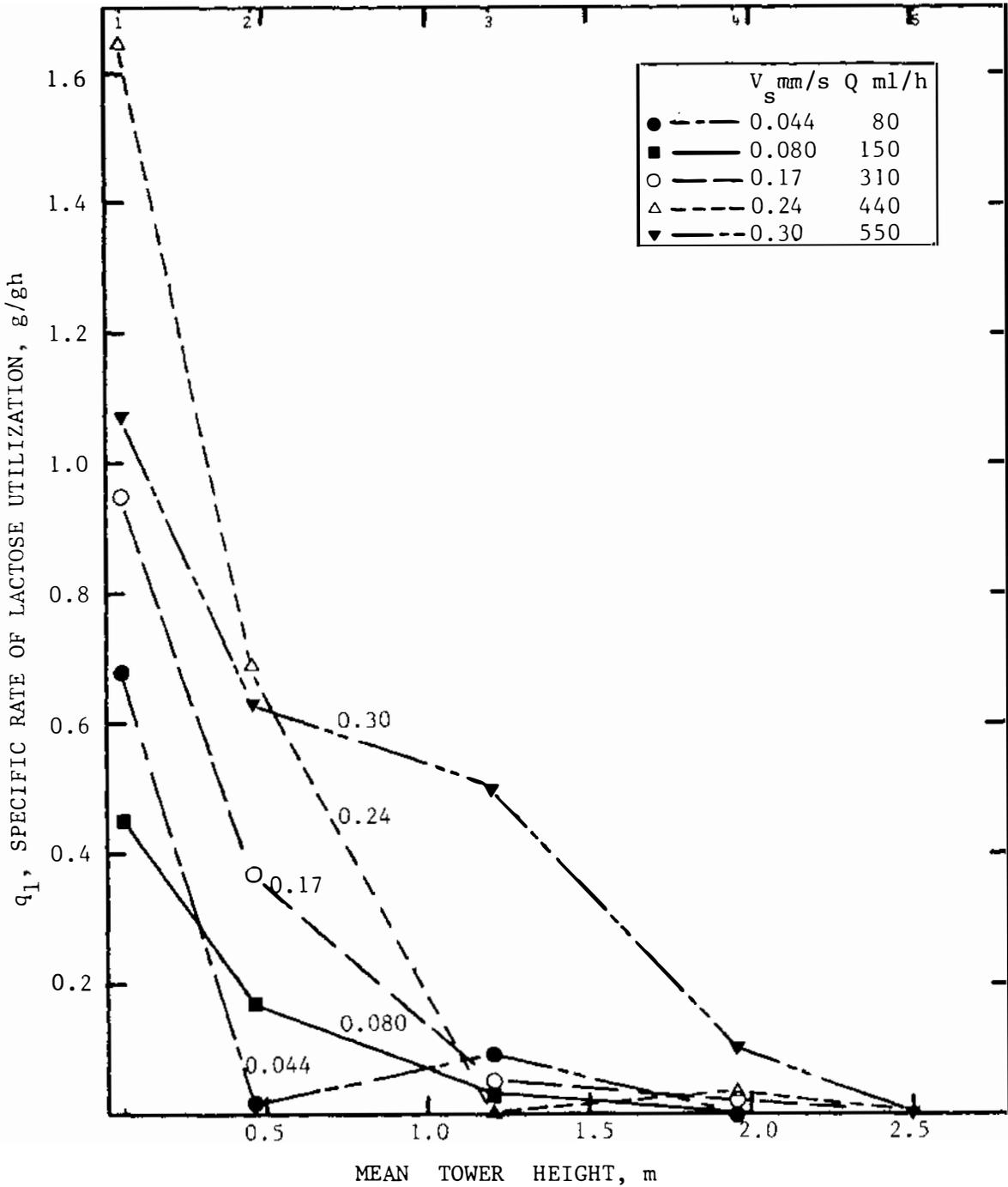
Fig.4.3 Specific rate of lactose utilization vs mean tower height at various superficial liquid velocities.
