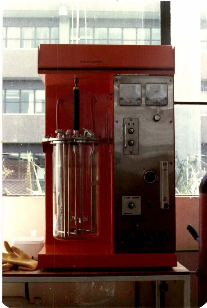
Fig.3.5 Batch fermenter (10 litre working volume).
