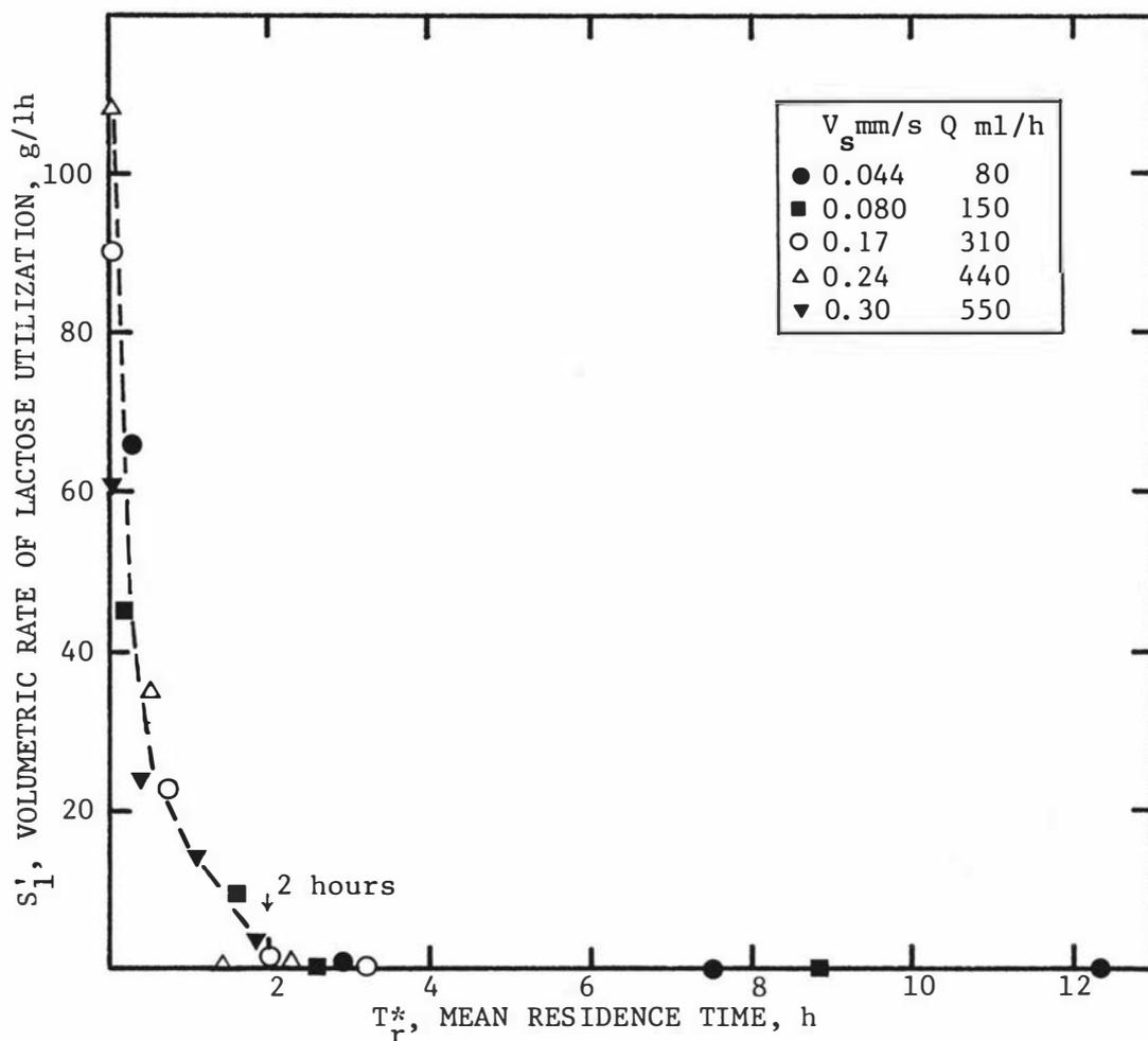
Fig.4.14 Volumetric rate of lactose utilization vs mean residence time at various superficial liquid velocities.
