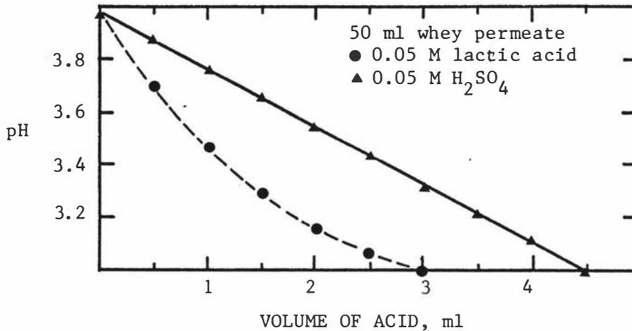
Fig.4.25 (a) Tower operation-monitoring curves for steady state determination at different medium feed rates, (b) Titration curves of a new batch of whey permeate with 0.05 M H<sub>2</sub>SO<sub>4</sub> and 0.05 M lactic acid in order to show the small amount of acid required to reduce the pH to below 4.0.
