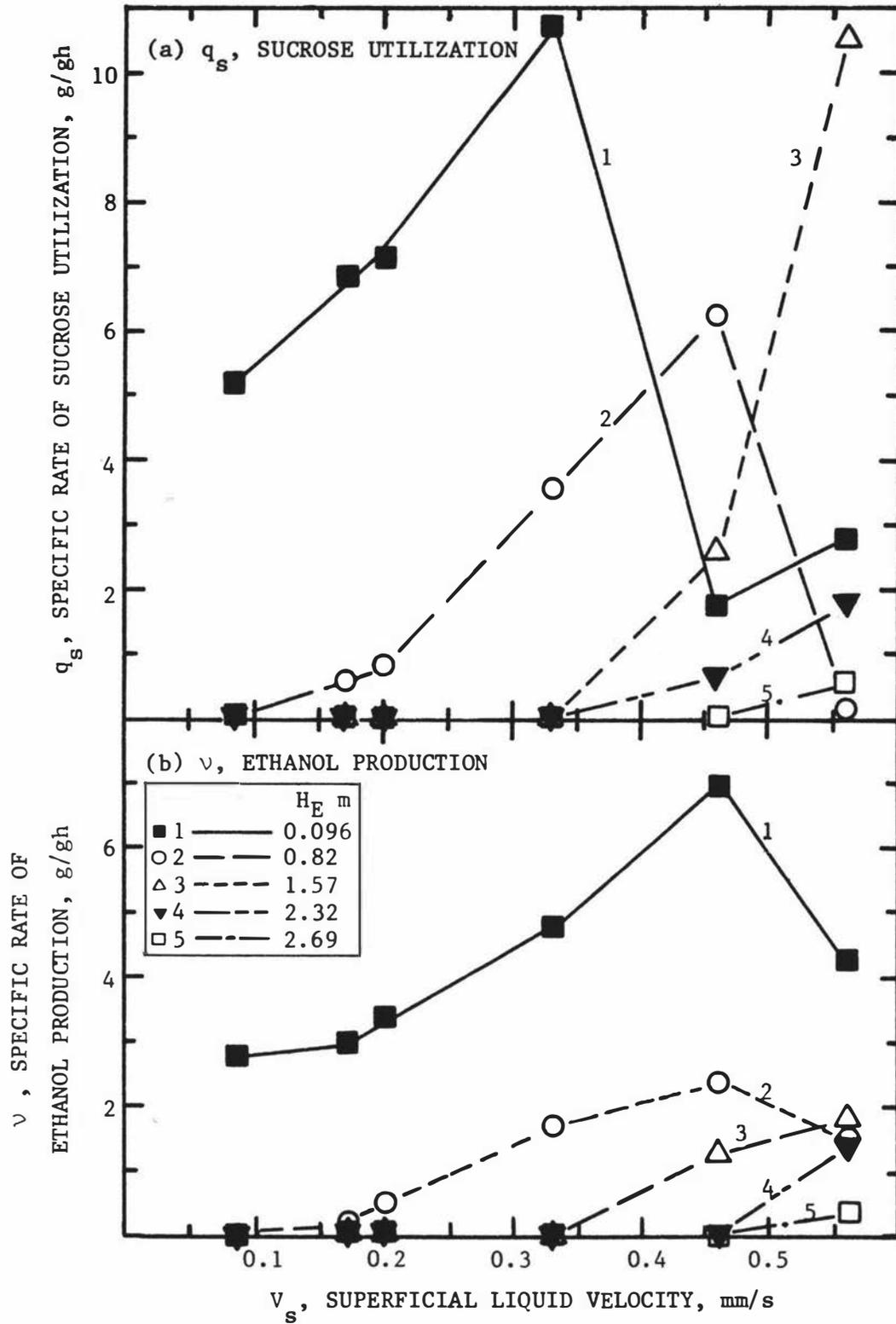
Fig. C.12 Specific rates of (a) sucrose utilization and (b) ethanol production vs superficial liquid velocity at various mean tower heights.
