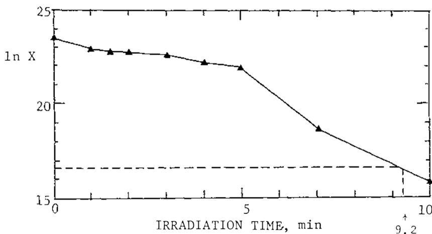
Fig.3.8 Survival of cells irradiated with UV light. KM10D10. (246 nm, distance 300 mm, in 9 g/l saline solution)
