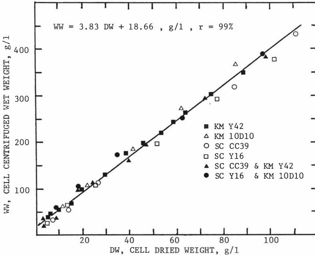
Fig.B.2 Cell centrifuged wet weight vs cell dried weight.
