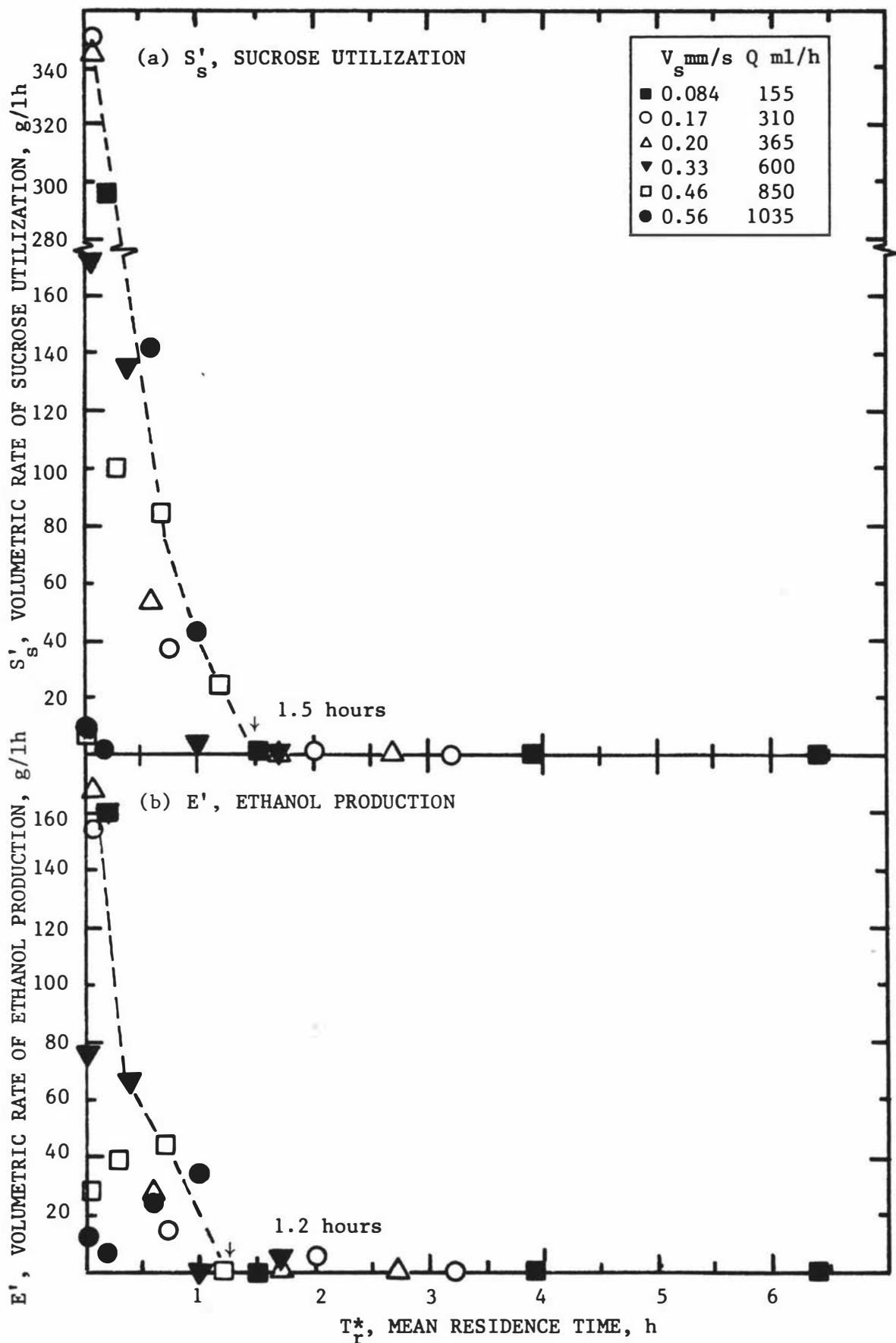
Fig. C.8 Volumetric rates of (a) sucrose utilization and (b) ethanol production vs mean residence time at various superficial liquid velocities
