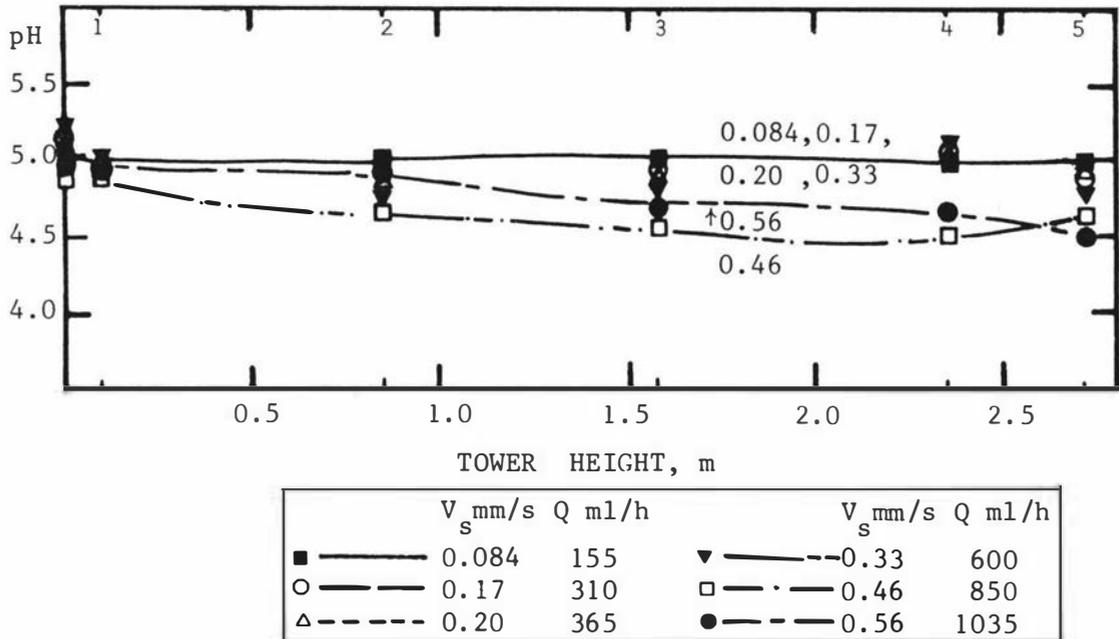
Fig.C.6 Medium pH vs tower height at various superficial liquid velocities
