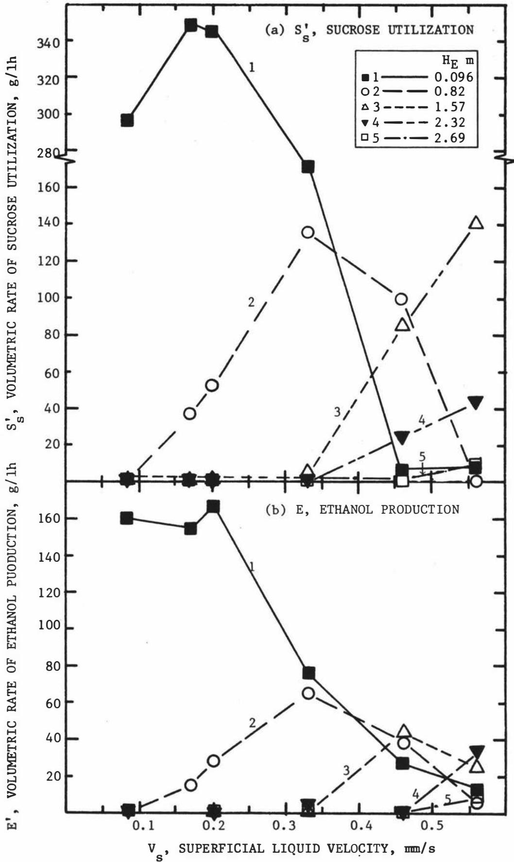
Fig. C.11 Volumetric rates of (a) sucrose utilization and (b) ethanol production vs superficial liquid velocity at various mean tower heights.
