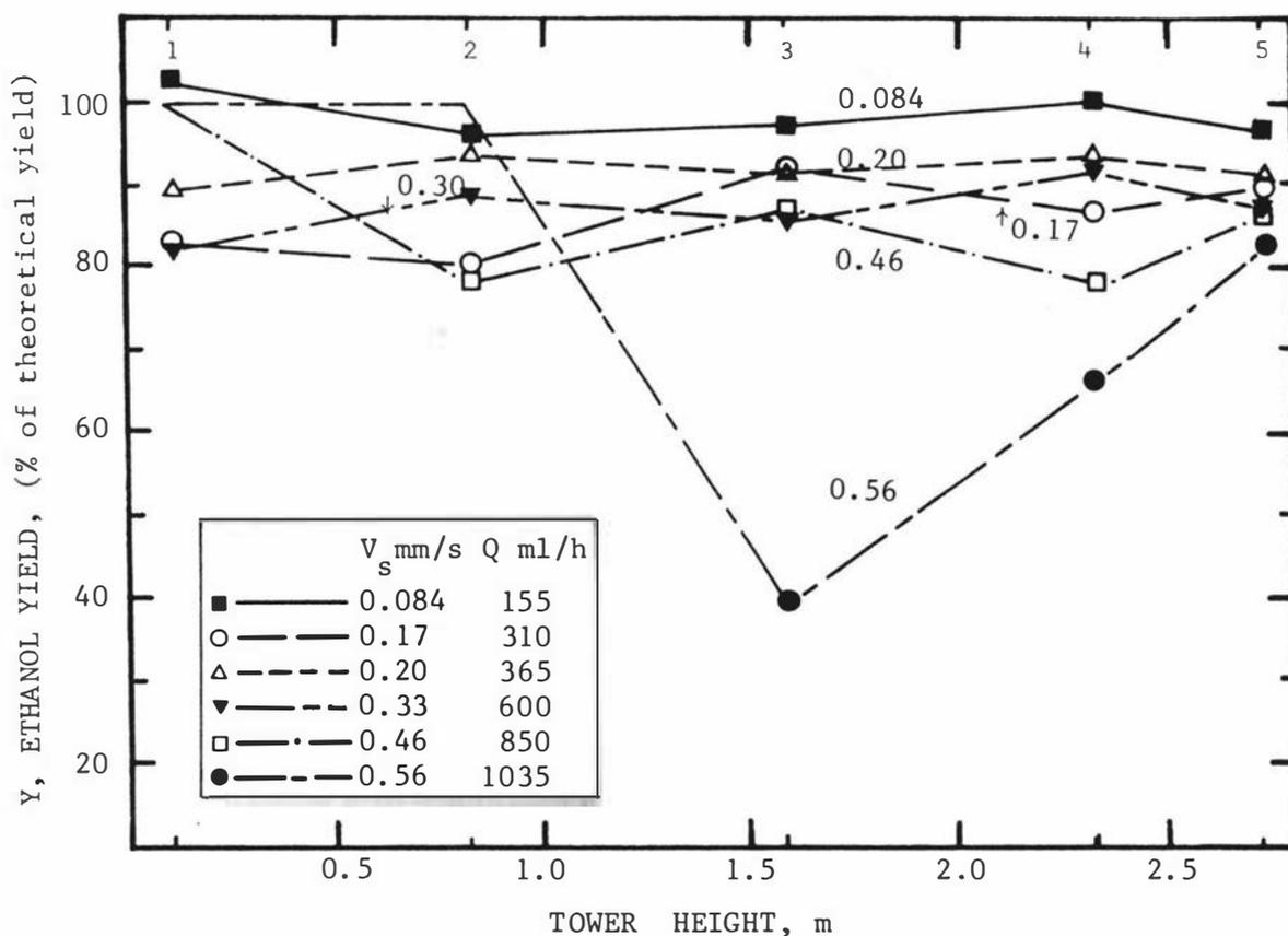
Fig.C.4 Ethanol yield (% of theoretical yield based of sucrose utilized) vs tower height at various superficial liquid velocities.
