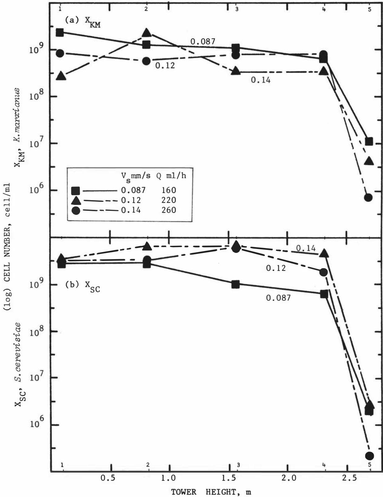
Fig. 5.7 Cell numbers vs tower height at various superficial liquid velocities. (a) *K. marxianus*, (b) *S. cerevisiae*. The corresponding estimated cell concentrations are given in table 5.4.
