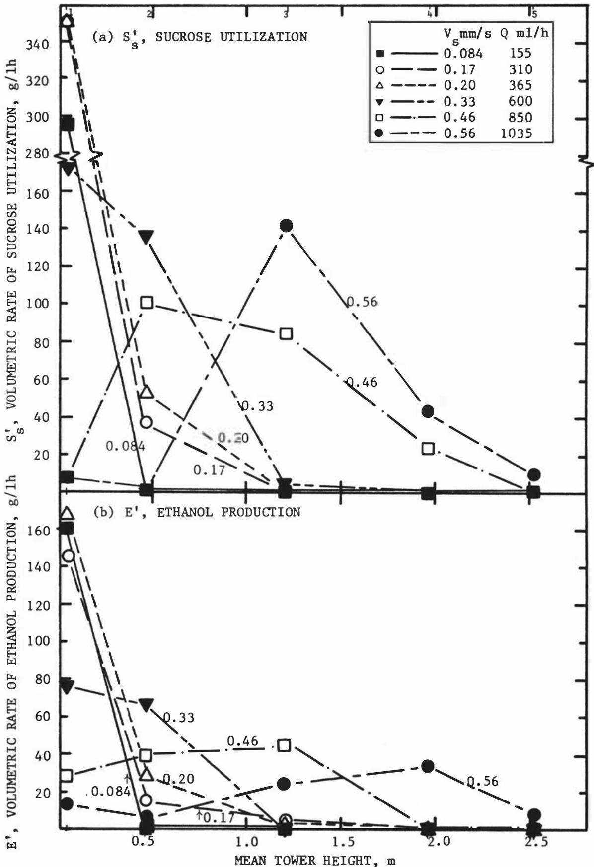
Fig.C.2 Volumetric rates of (a) sucrose utilization and (b) ethanol production vs mean tower height at various superficial liquid velocities.
