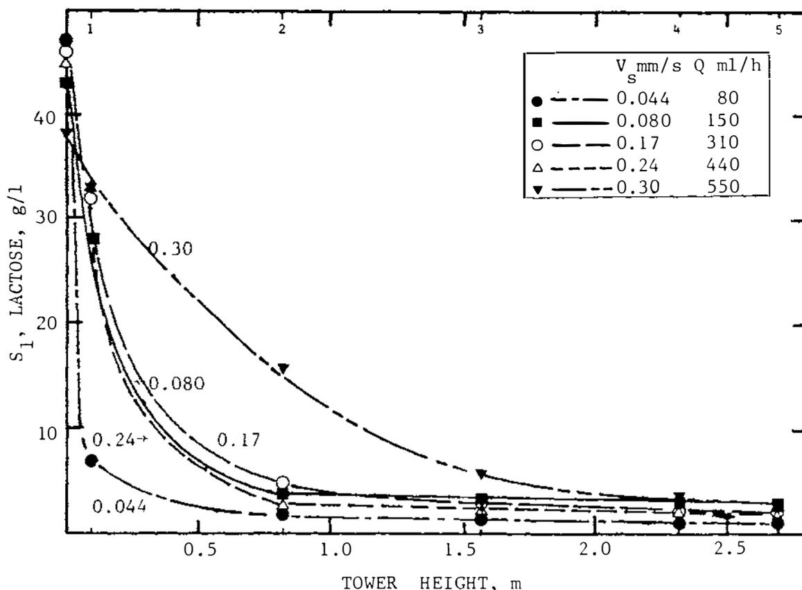
Fig.4.1 Lactose concentration vs tower height at various superficial liquid velocities.
