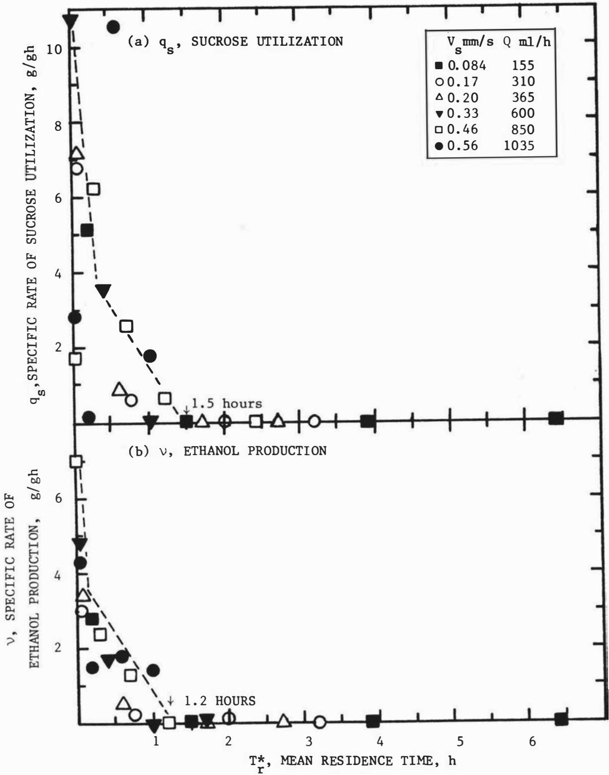
Fig. C.9 Specific rates of (a) sucrose utilization and (b) ethanol production vs mean residence time at various superficial liquid velocities.
