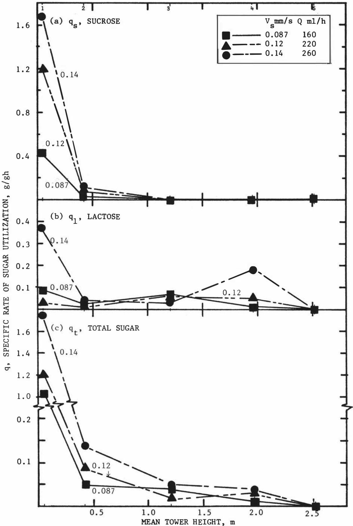
Fig. 5.3 Specific rate of sugar utilization vs mean tower height at various superficial liquid velocities.
