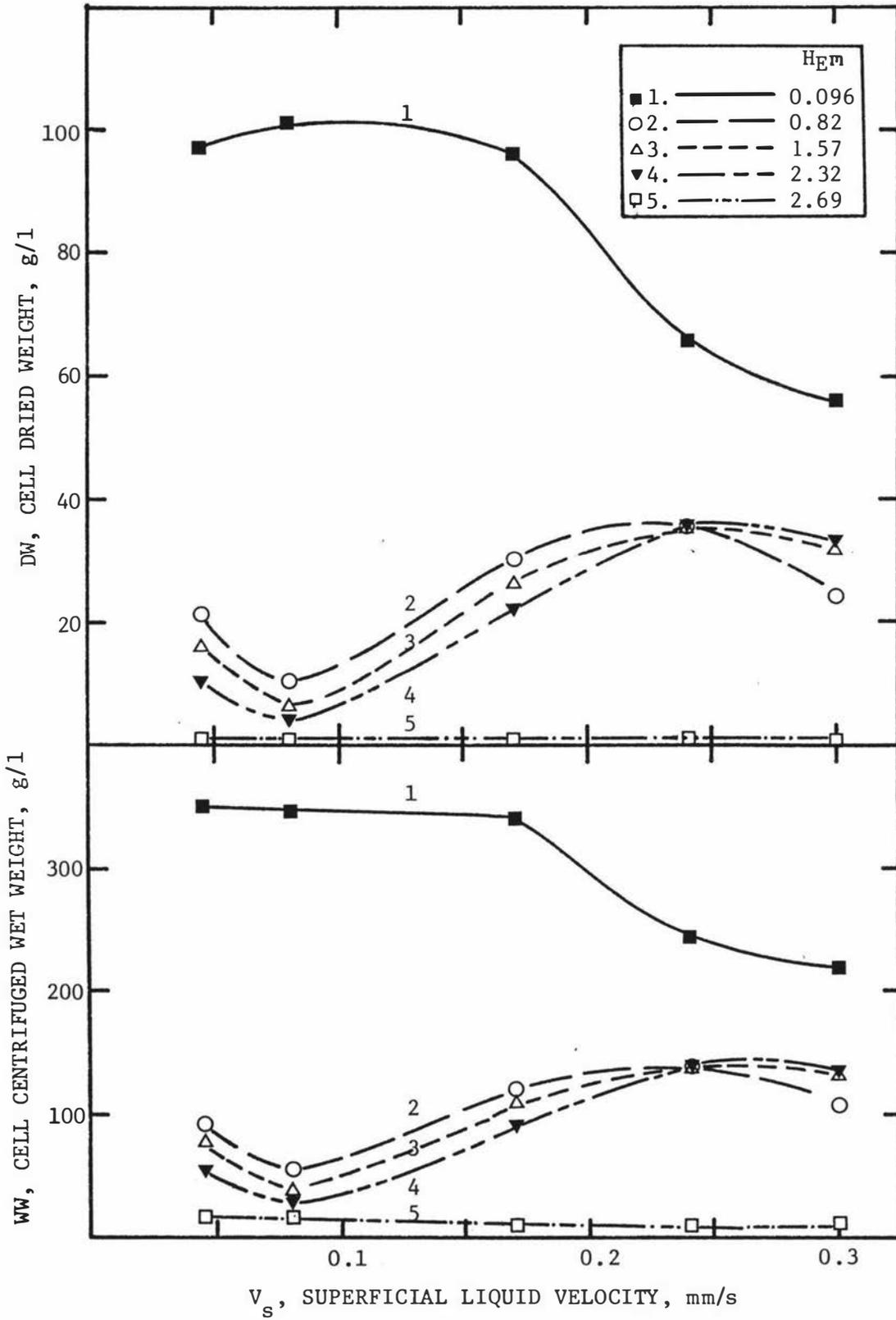
Fig.4.24 Cell concentration vs superficial liquid velocity at various tower heights.
