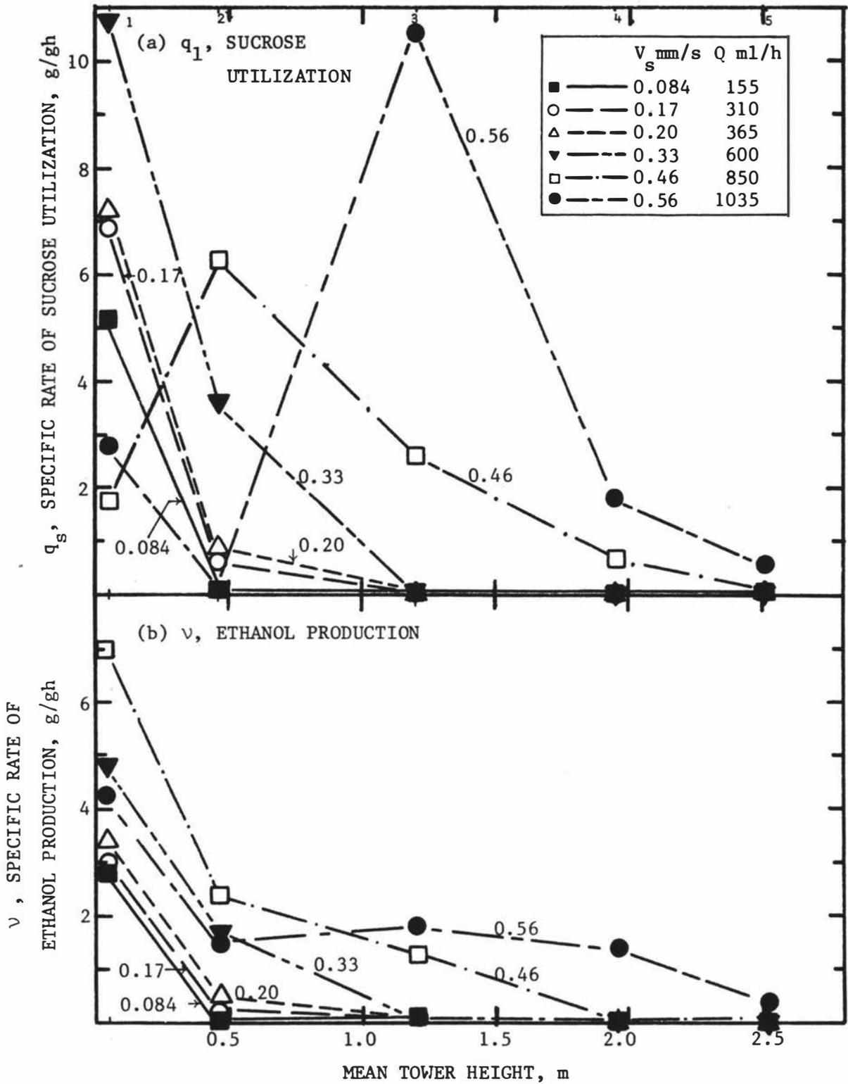
Fig.C.3 Specific rates of (a) sucrose utilization and (b) ethanol production vs mean tower height at various superficial liquid velocities.
