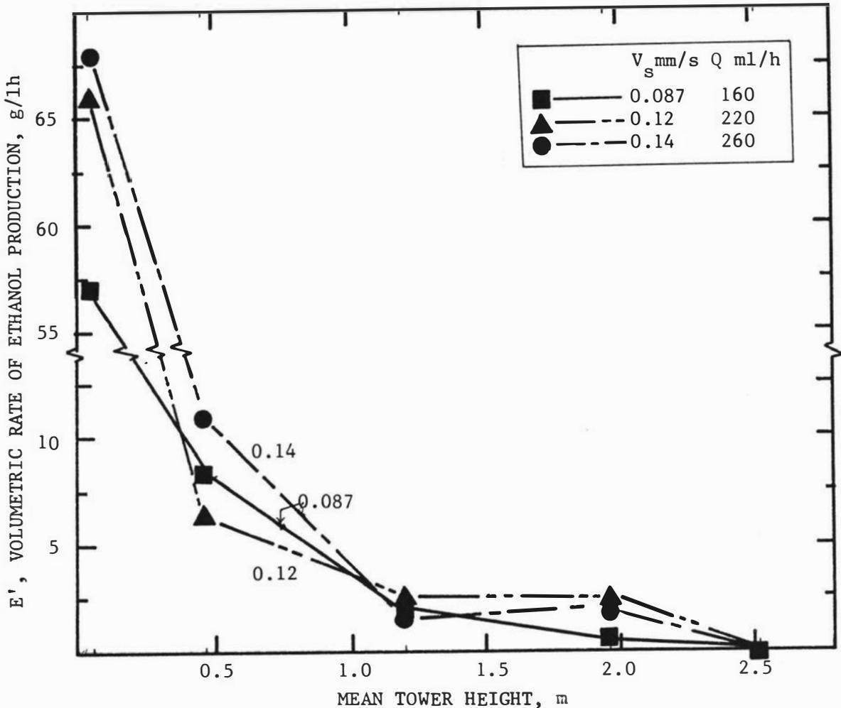
Fig. 5.6 Volumetric rate of ethanol production vs mean tower height at various superficial liquid velocities.
