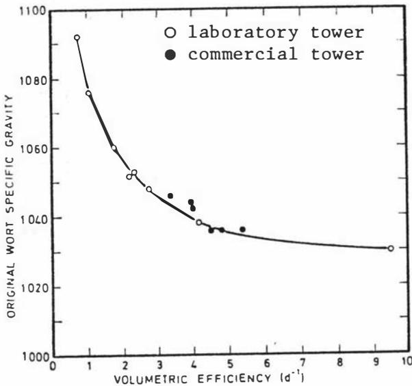
Fig.2.5 The effect of original feed liquor specific gravity on the limiting volumetric efficiency for a physically limited yeast.
