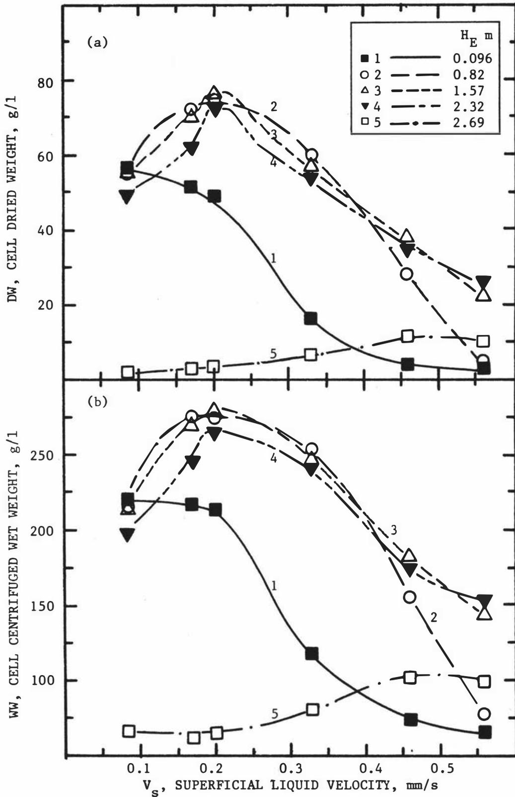
Fig.C.13 Cell concentration vs superficial liquid velocity at various tower heights.
