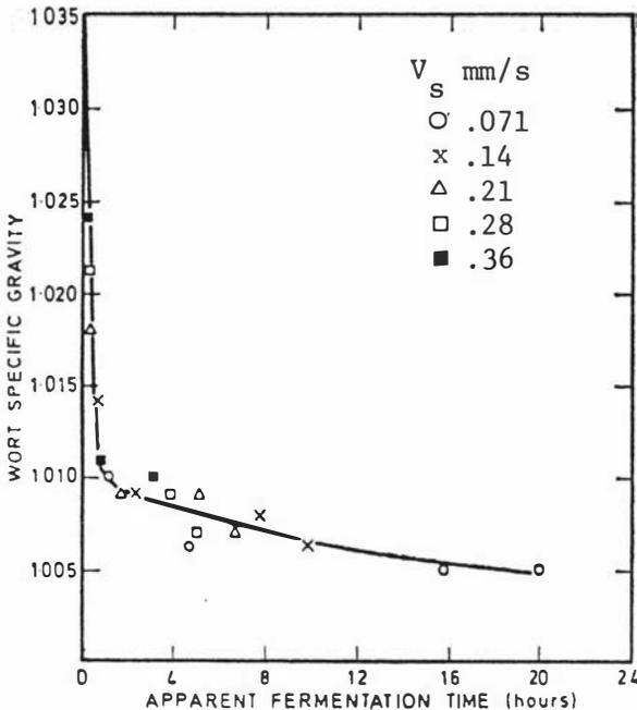
Fig.2.4 The relationship between feed liquor specific gravity and apparent fermentation time in tower fermentation of beer using physically limited yeast. (Klopper et al 1965)
