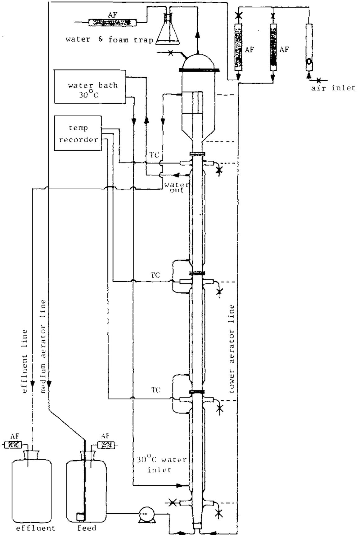
Fig.3.4 Water heating and air filtration systems for the tower fermenter. AF - air filter ; TC - thermocouple
