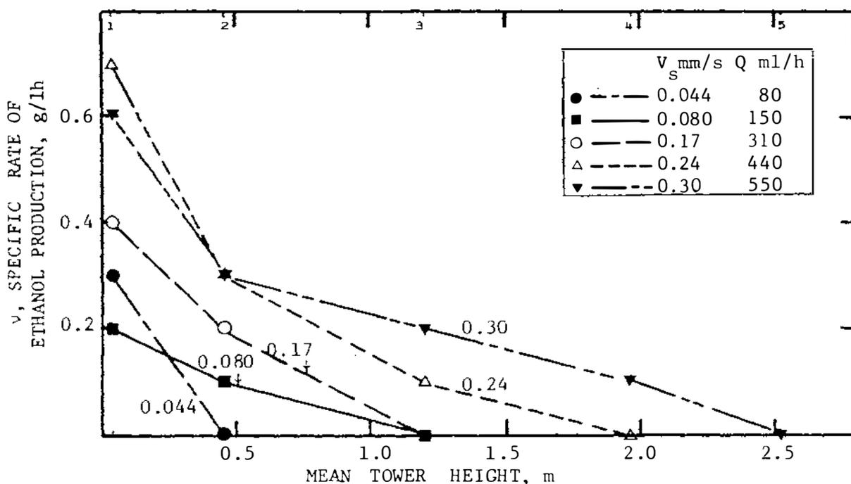
Fig.4.7 Specific rate of ethanol production vs mean tower height at various superficial liquid velocities.
