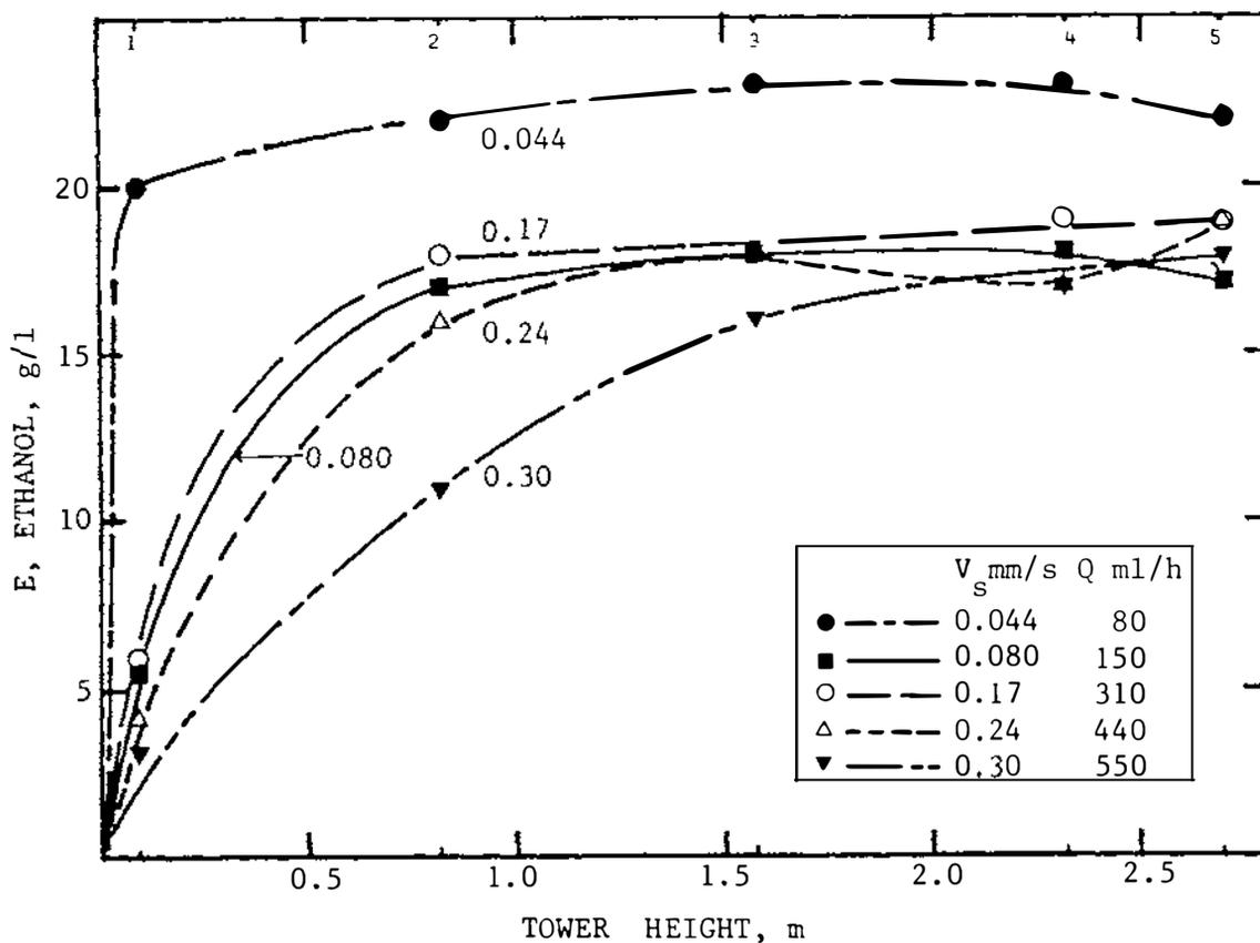
Fig.4.4 Ethanol concentration vs tower height at various superficial liquid velocities.
