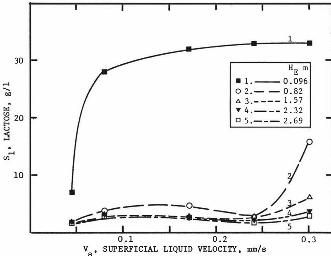
Fig.4.18 Lactose concentration vs superficial liquid velocity at various tower heights.
