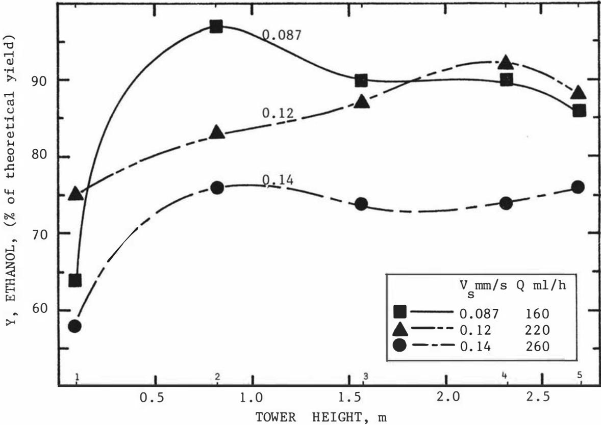
Fig. 5.5 Ethanol yield vs tower height at various superficial liquid velocities.
