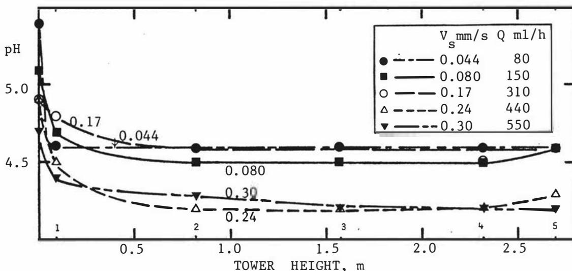
Fig.4.11 Medium pH vs tower height at various superficial liquid velocities.
