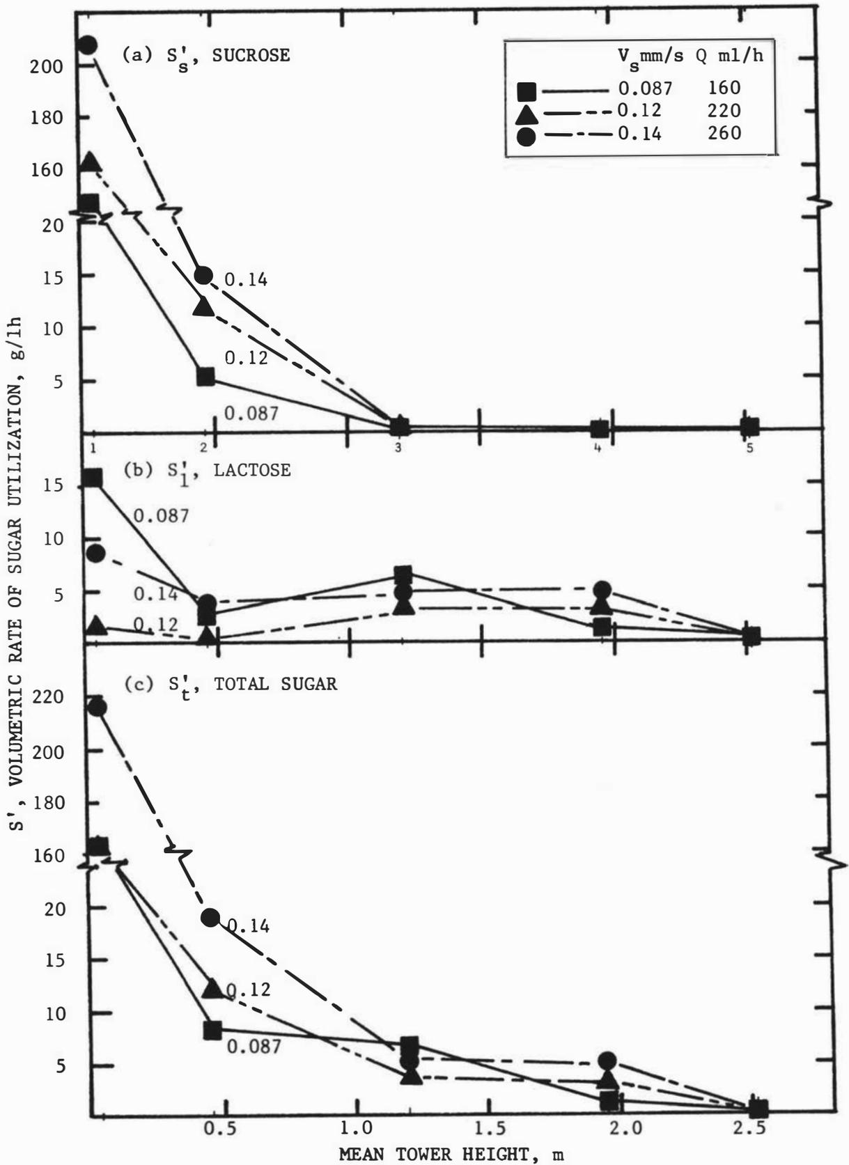
Fig. 5.2 Volumetric rates of sugar utilization vs mean tower height at various superficial liquid velocities. (a) Sucrose, (b) Lactose, (c) Total sugar.
