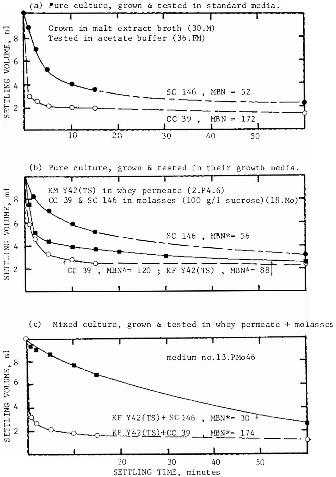
Fig.6.1 Flocculation of KM Y42(TS), SC146, and CC39 grown and tested in different media.
