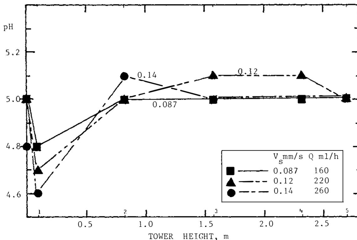
Fig. 5.10 Medium pH vs tower height at various superficial liquid velocities.
