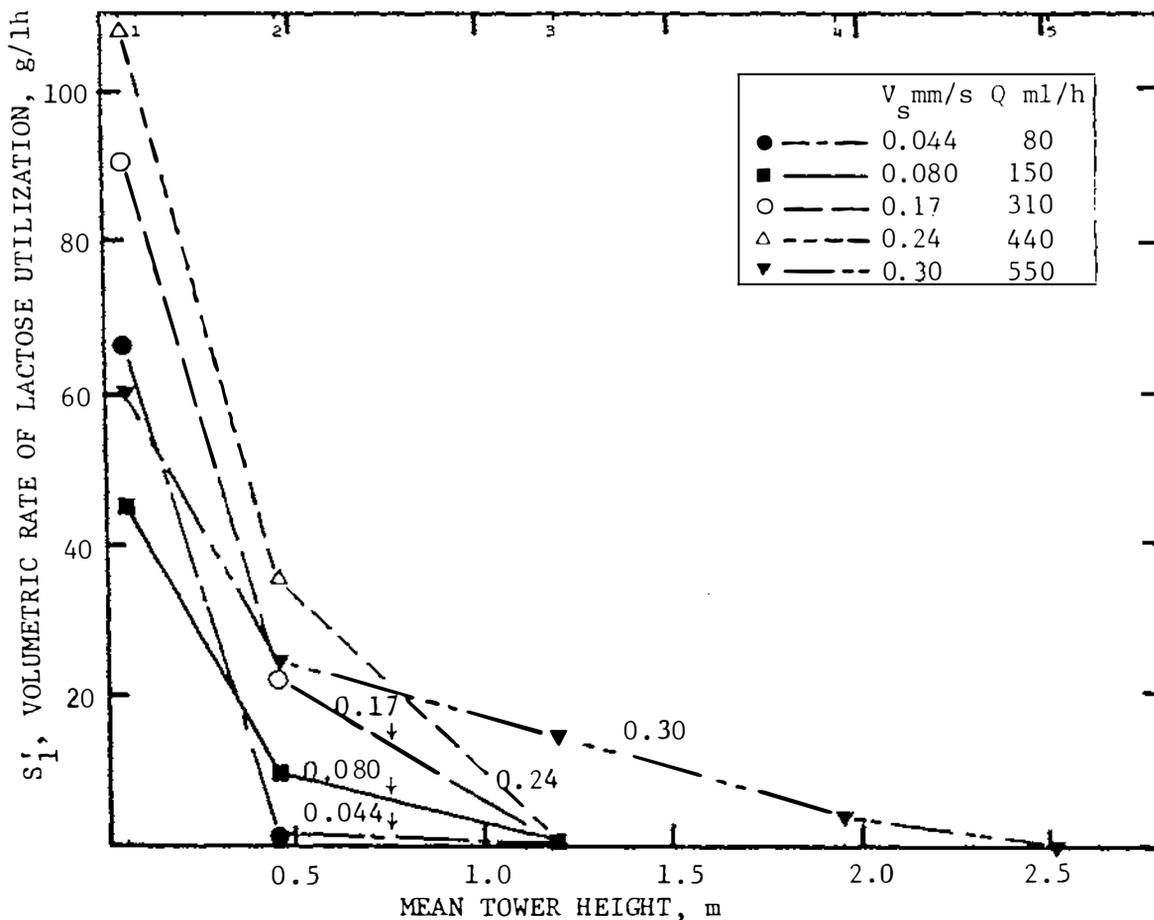
Fig. 4.2 Volumetric rate of lactose utilization vs mean tower height at various superficial liquid velocities.
