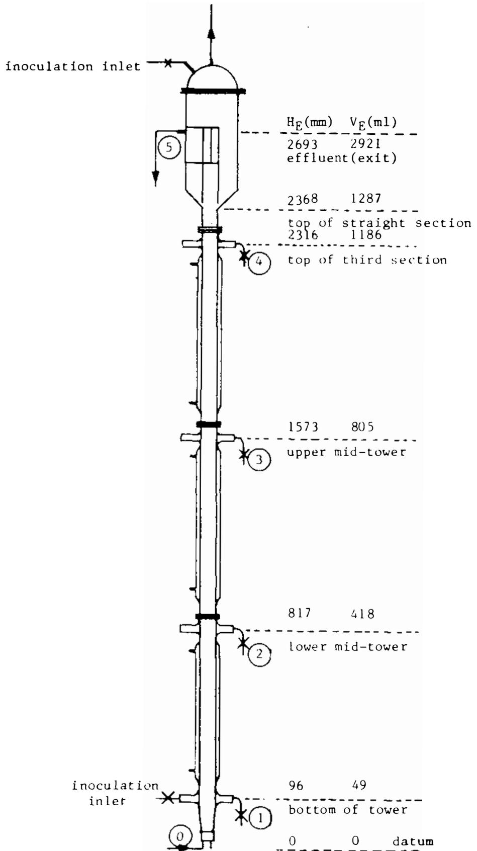
Fig. 3.2 Schematic diagram of the tower fermenter.
