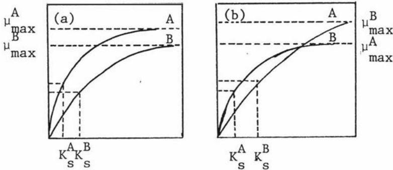
Fig.2.8  $\mu$ - $S$  relationship of two organisms A and B. (a)  $K_s^A < K_s^B$  and  $\mu_{max}^A > \mu_{max}^B$ ; (b)  $K_s^A < K_s^B$  and  $\mu_{max}^A < \mu_{max}^B$  (Veldkamp & Jannasch 1972).
