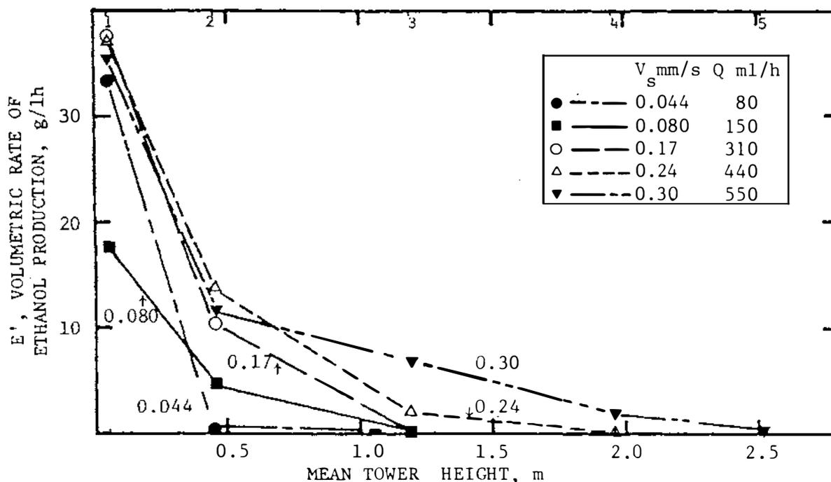
Fig.4.6 Volumetric rate of ethanol production vs mean tower height at various superficial liquid velocities.
