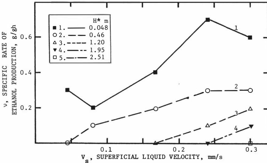
Fig.4.23 Specific rate of ethanol production vs superficial liquid velocity at various tower heights.
