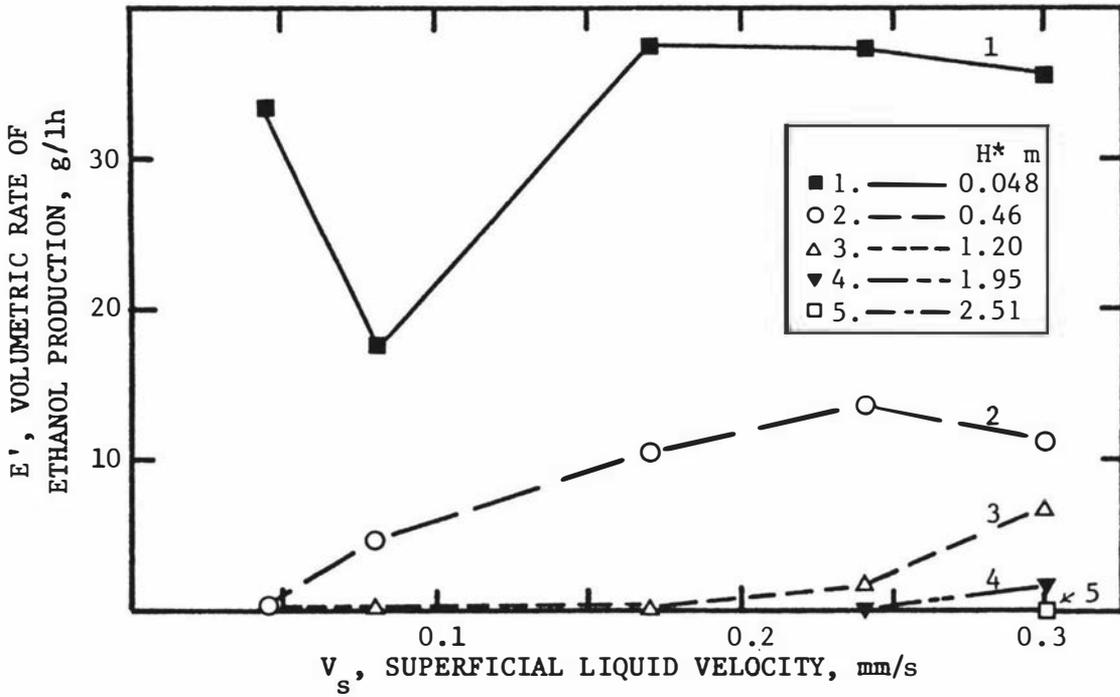
Fig.4.22 Volumetric rate of ethanol production vs superficial liquid velocity at various mean tower heights.
