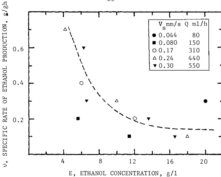
Fig. 4.8 Specific rate of ethanol production vs ethanol concentration at various superficial liquid velocities.
