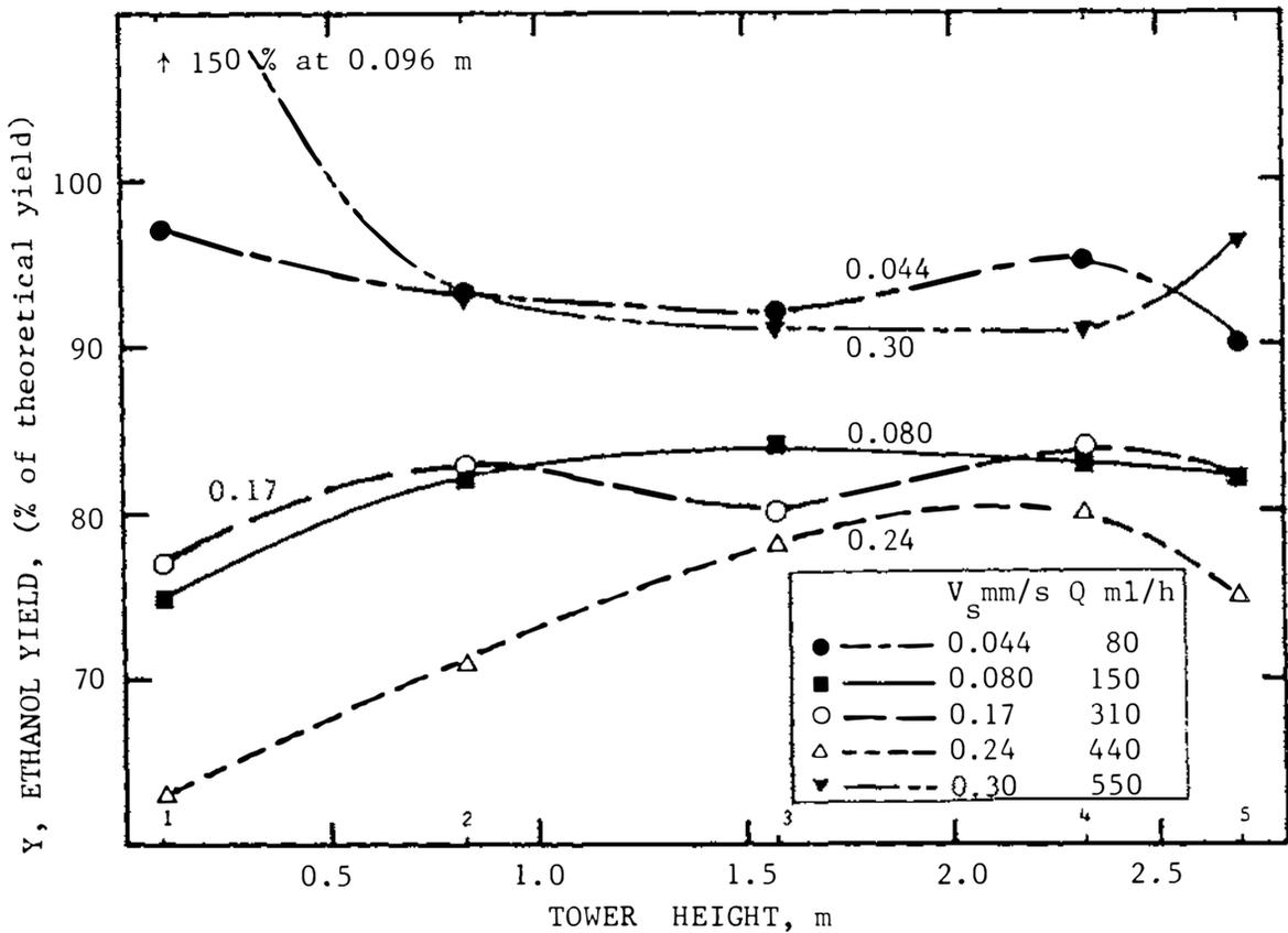
Fig.4.5 Ethanol yield vs tower height at various superficial liquid velocities.
