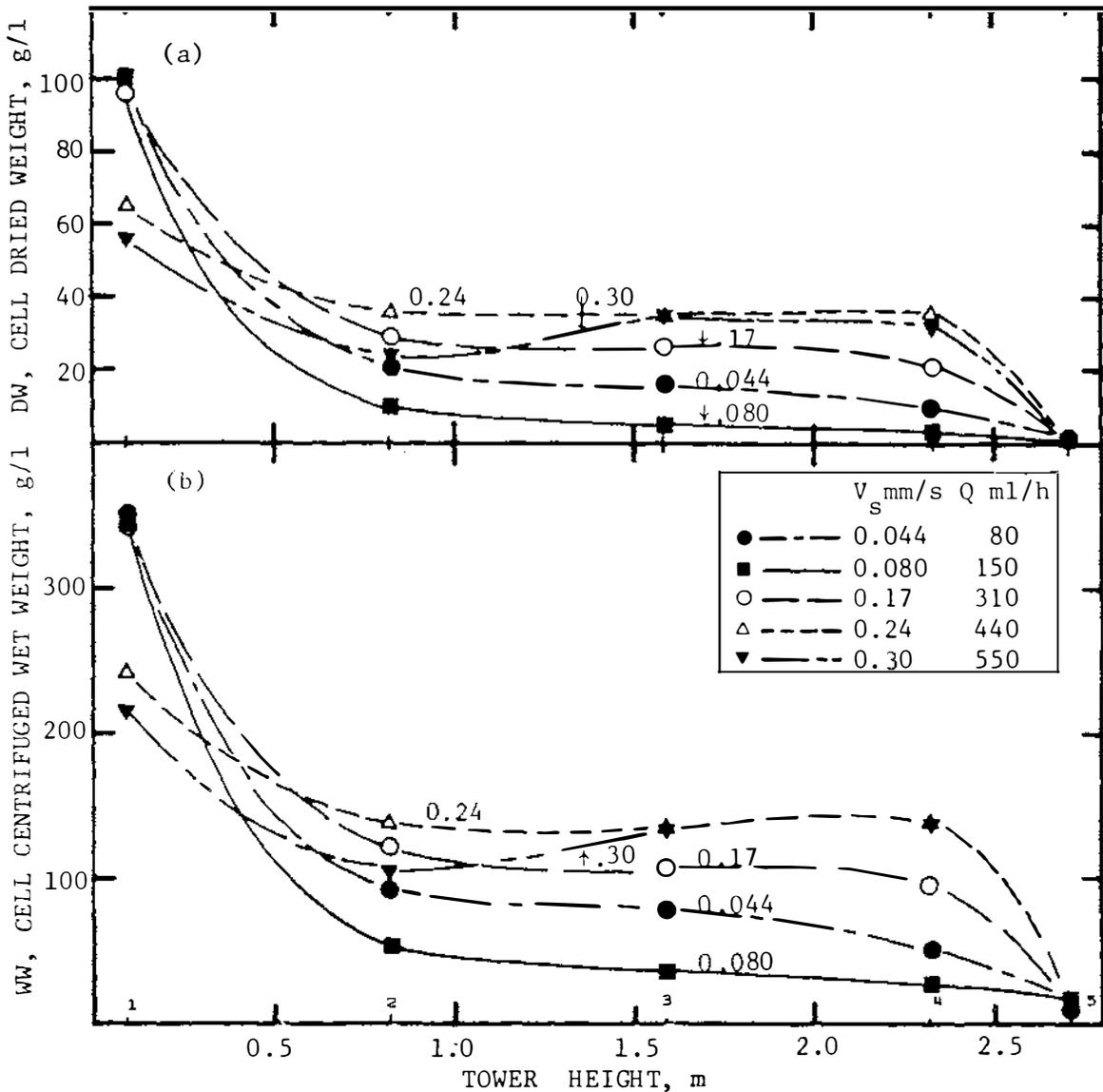
Fig.4.9 Cell concentration vs tower height at various superficial liquid velocities.
