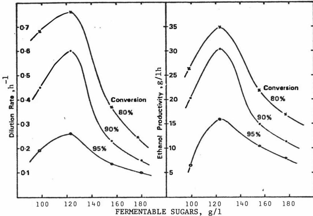
Fig.2.6 The effect of fermentable sugars concentration on the dilution rate and ethanol productivity of tower fermentation of cane juice (Prince Barford 1982).
