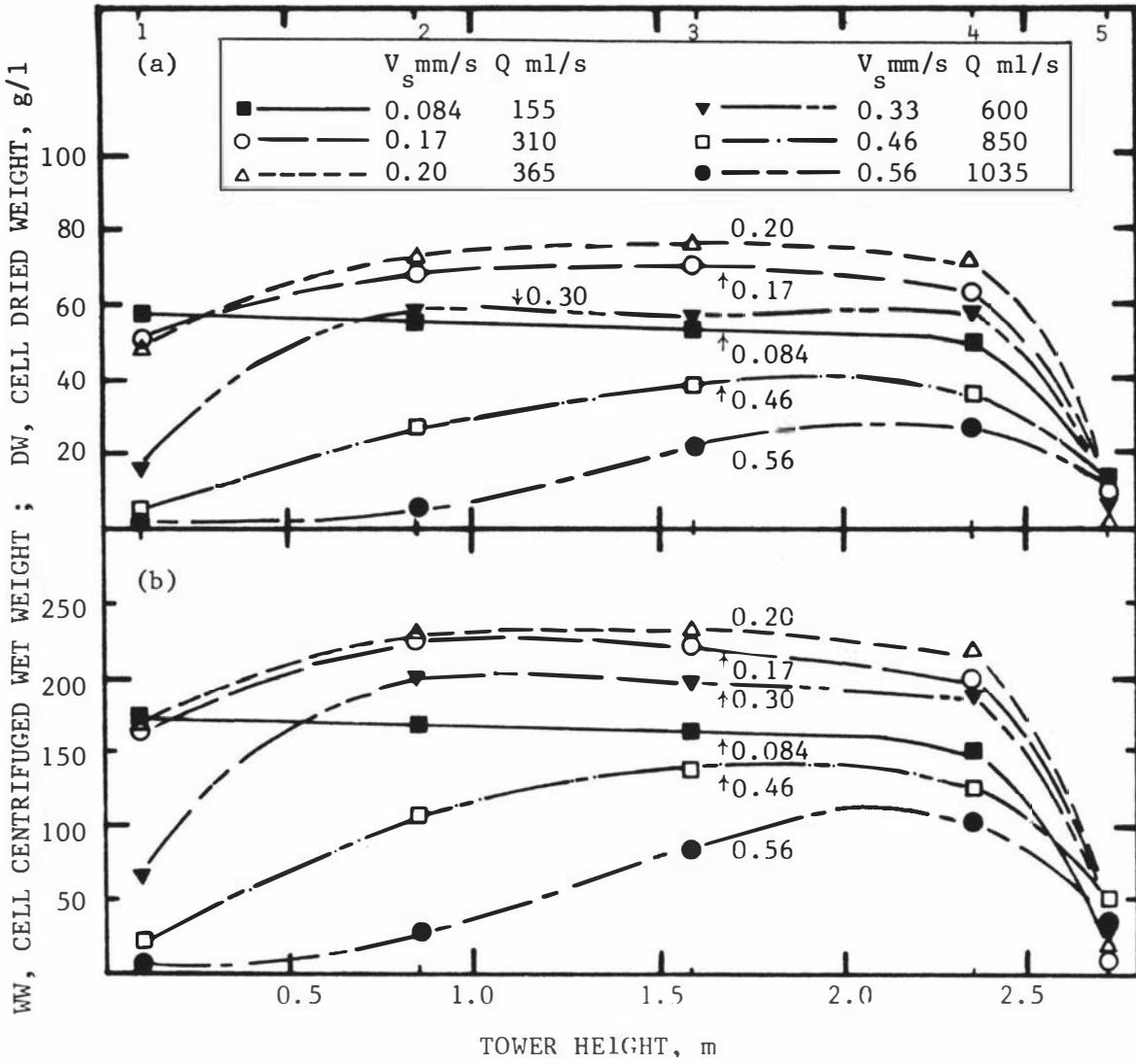
Fig.C.5 Cell concentration vs tower height at various superficial liquid velocities.
