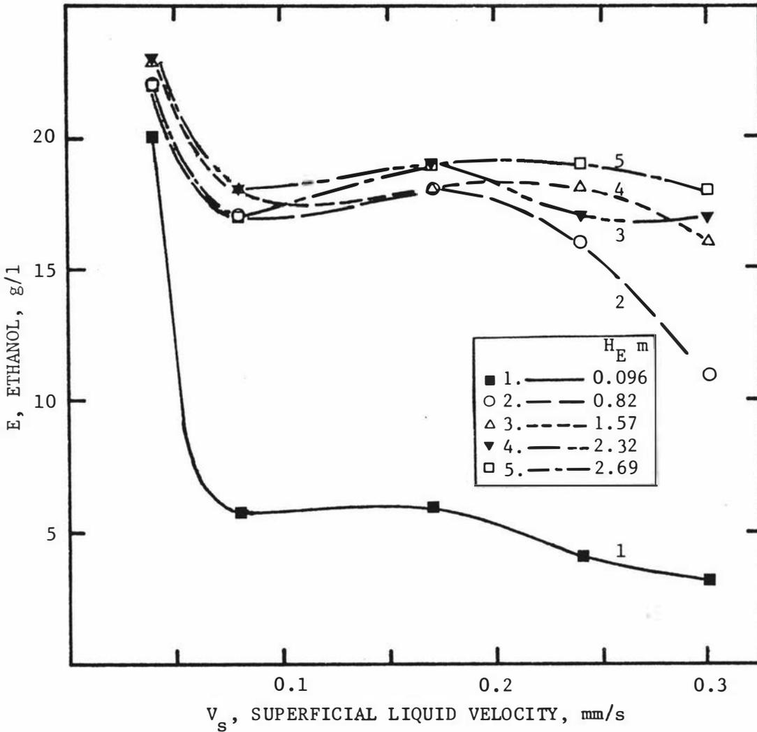
Fig.4.19 Ethanol concentration vs superficial liquid velocity at various tower heights.
