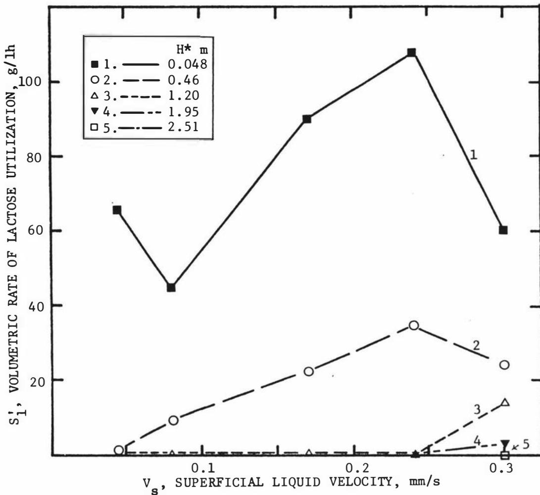
Fig.4.20 Volumetric rates of lactose utilization vs superficial liquid velocity at various mean tower heights.
