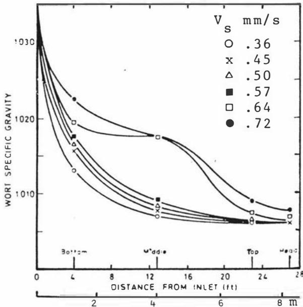
Fig.2.3 Progressive reduction of wort gravity in a tower fermenter at various flow rates using physically limited yeast. (Greenshields & Smith 1971)
