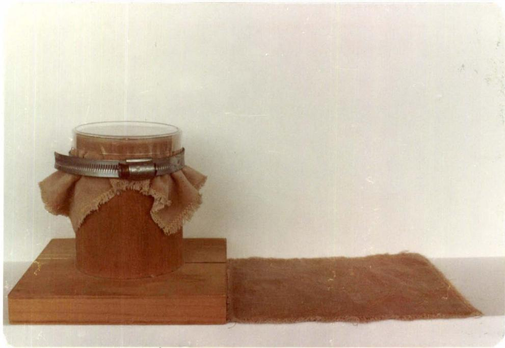
Fig.3.6 Replication equipment. Wooden supporting base and replicating cloth.
