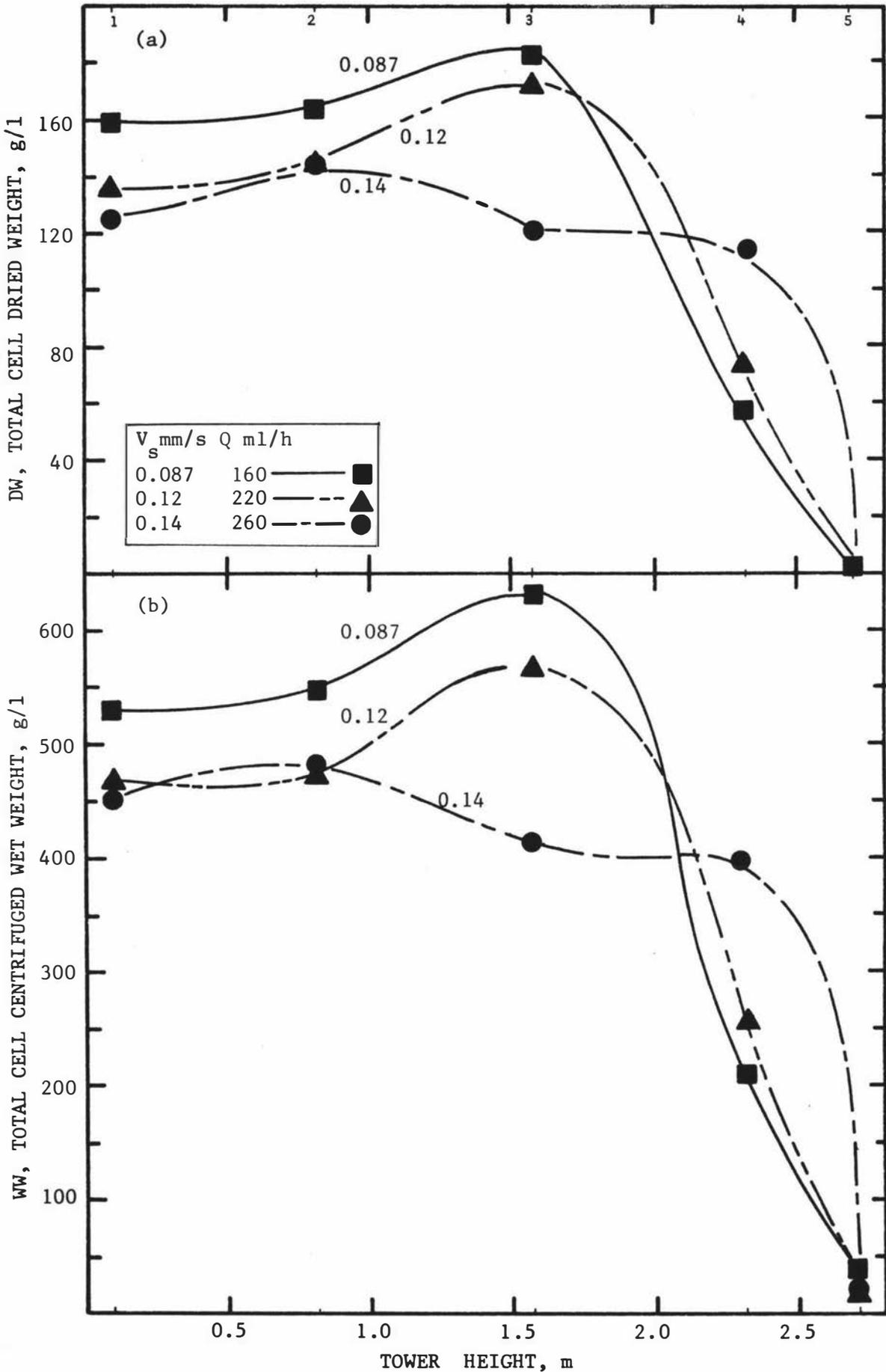
Fig. 5.8 Cell concentration vs tower height at various superficial liquid velocities. (a) Cell dried weight, (b) Cell centrifuged wet weight.
