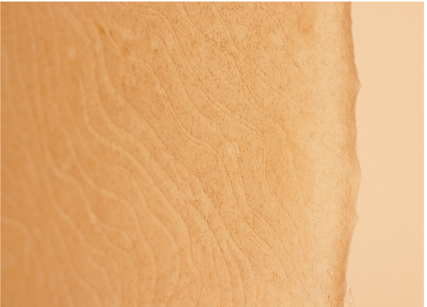
Fig. 15 Laser-engraved wool-based film
