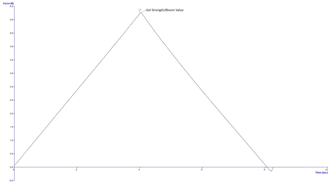
Figure 3.33: A graphic representation of the indentation test, specifically for the 10%wt specimen
