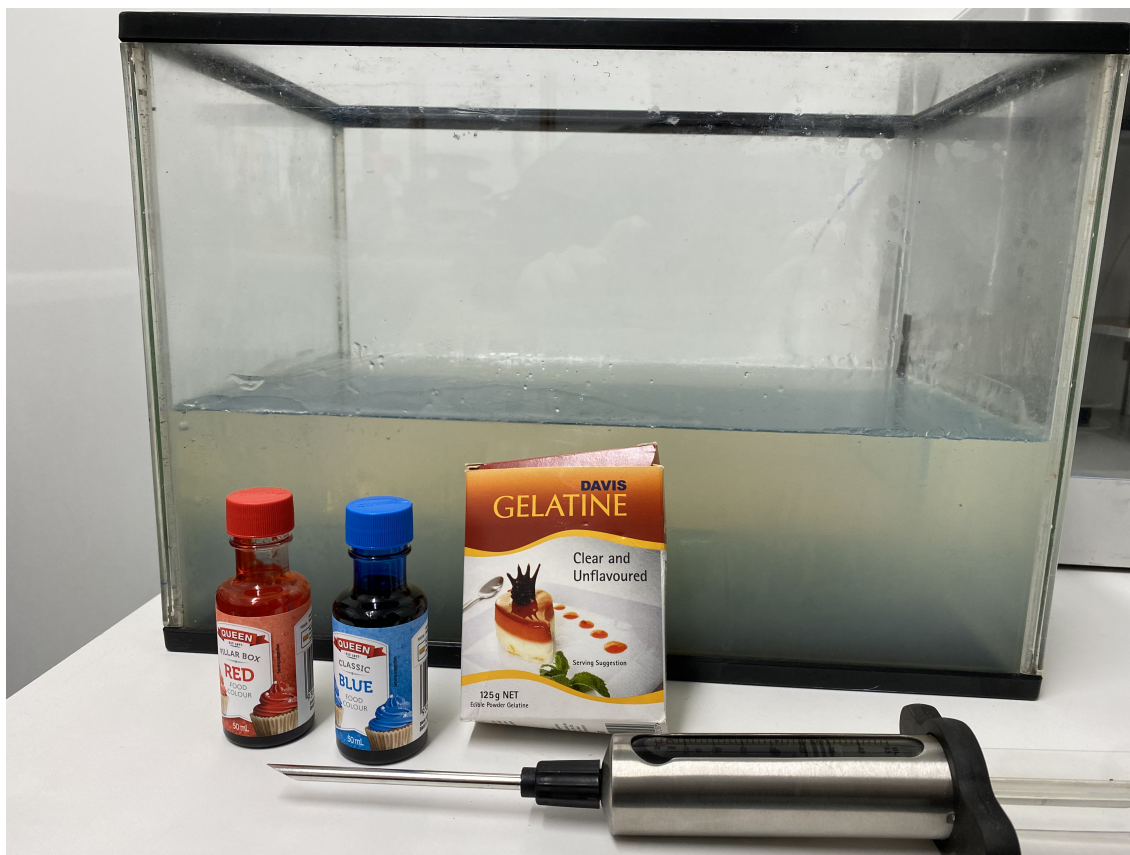
Figure 2.17: Proof-of-concept using a non-self-healing gel and dye to indicate the needle tracks.
