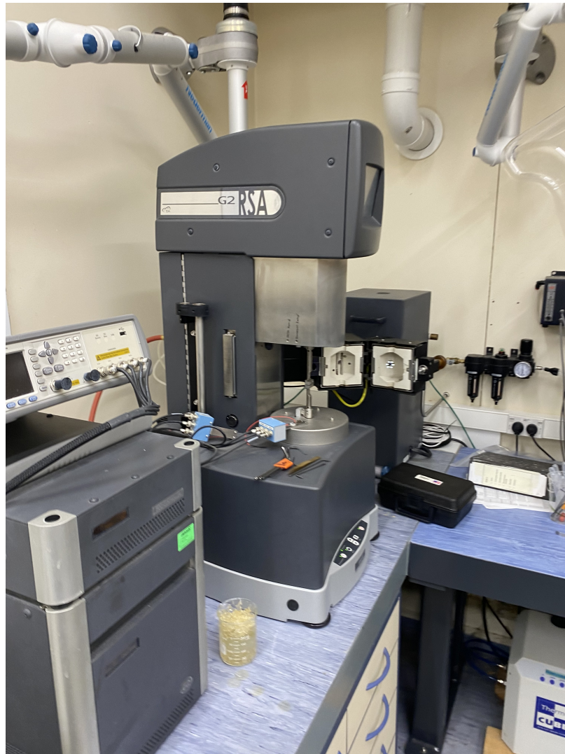
Figure 3.18: Gelatine cube compression testing machine — Dynamic Mechanical Analysis RSAG2
