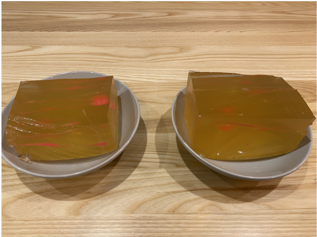
Figure 5.6: Separated blocks ( 250mm x 200mm x 150mm) of the gelatine phantom body enclosing the formed alginate fibres which is ready for extraction by subjecting the blocks to a temperature > 35^{\circ}\text{C} .
