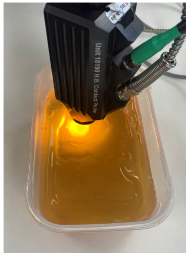
Figure 3.13: The measuring of the gelatine spectra using the ASD
