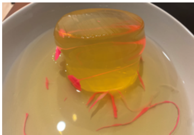
Figure 5.7: Partially-extracted calcium alginate fibres formed inside of gelatine using sodium alginate as the deposition and calcium chloride as the “binder” or reactant. The gelatine melts at > 35^{\circ}\text{C} .
