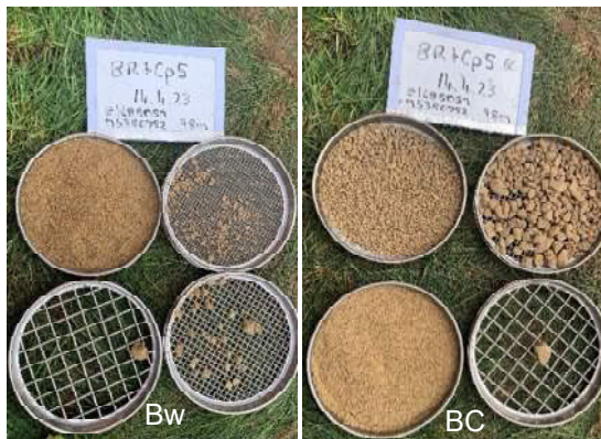
Sieved horizons for Transect C Pit 5. Size grades >20mm (coarse) ,>6mm (medium), >2mm (fine).
