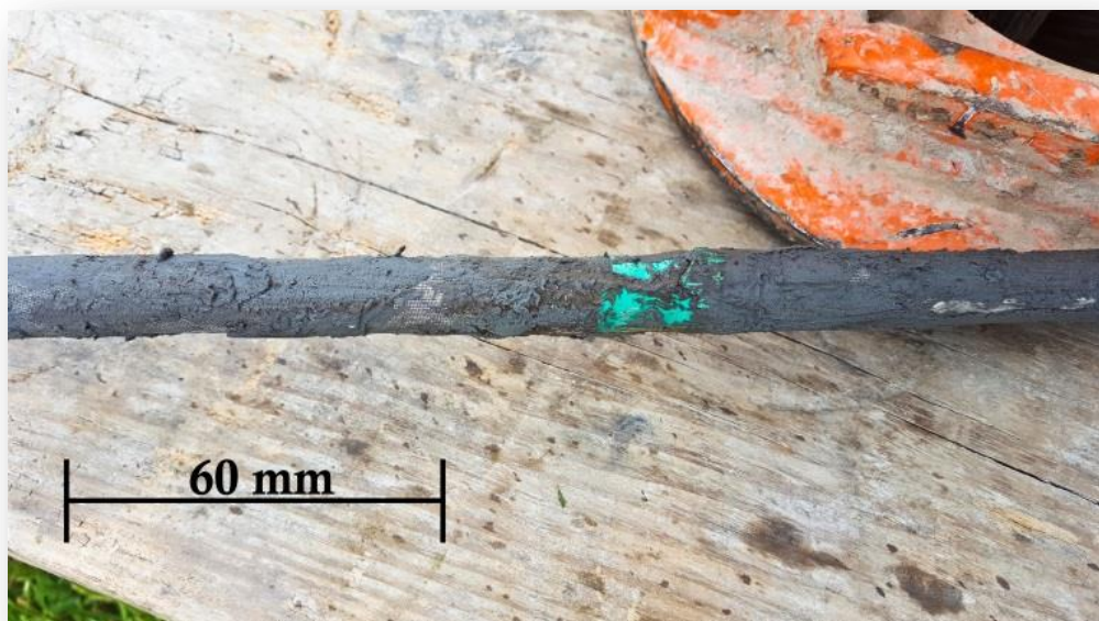
Figure 48: Clogged screen. Careful management of screen depth was required to avoid clogging by fine suspended sediments.
