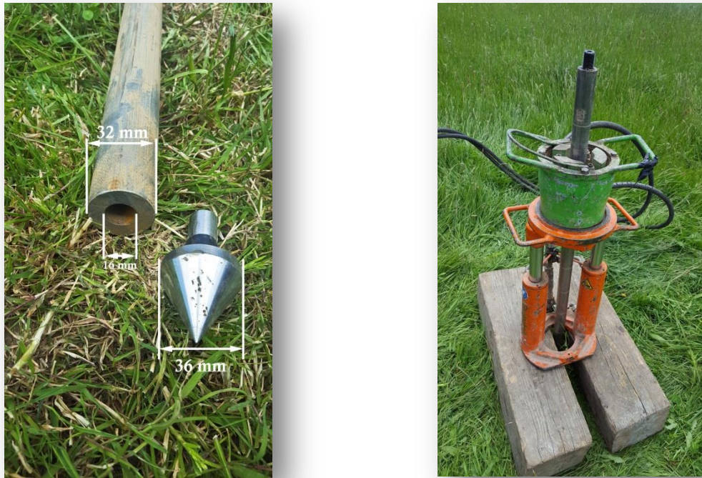
Figure 43: Left: CPT Rod, sampling head and sacrificial tip with dimensions. Right: Hydraulic lifter assembly, Green collet chuck clamps on the rods when jack (orange) is raised. Timber blocks stop the assembly from being forced into the ground when raising the drill rods in soft conditions.
