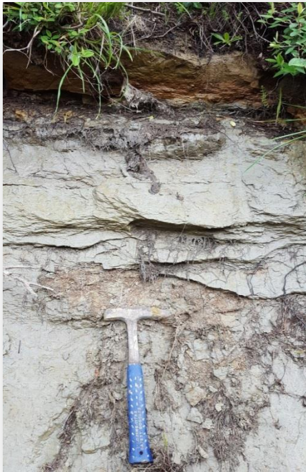
Figure 104: Onoke group sediments in a road cutting (Alfredton Road, Eketahuna 40°39'59.0"S 175°47'22.8"E) 7 km West of site 50.3. It is difficult to determine the provenance of water recovered from site 50.3 but it may be water trapped in the fractured mudstone or the slightly more permeable sediments directly on top of the contact between the overlying layer.
