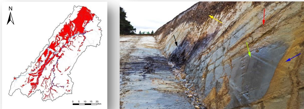
Figure 29: Pleistocene sediments tend to be distributed in the expansive central plains of the Tararua GWMZ and the rolling hill country north of Dannevirke (left). The complex sequence of lacustrine and fluvial sediments (right, road cutting north of Whakaruatapu River 40°14'81.7"S 176°15'27.7"E) is indicative of the latter stages of the demise of the Ruataniwha Strait.. Arrows indicates peat and lignite (black arrow), lacustrine mudstone (chartreuse), pumice sands (blue), eastward dipping bedding planes (red) and angular unconformity between Pliocene and Pleistocene sediments (Map generated in ArcGIS 10.2 using shapefiles from Heron, 2014; Land Information New Zealand, 2011b).
