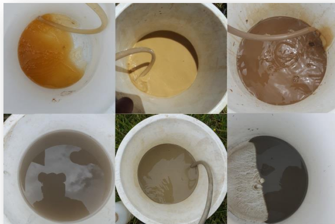
Figure 49: A range of different coloured water collected soon after pumping initiated. The appearance of the groundwater indicated of the nature of substrate the well was drilled into. Generally the water had cleared by the time physical parameters had stabilised enough for sampling to proceed.
