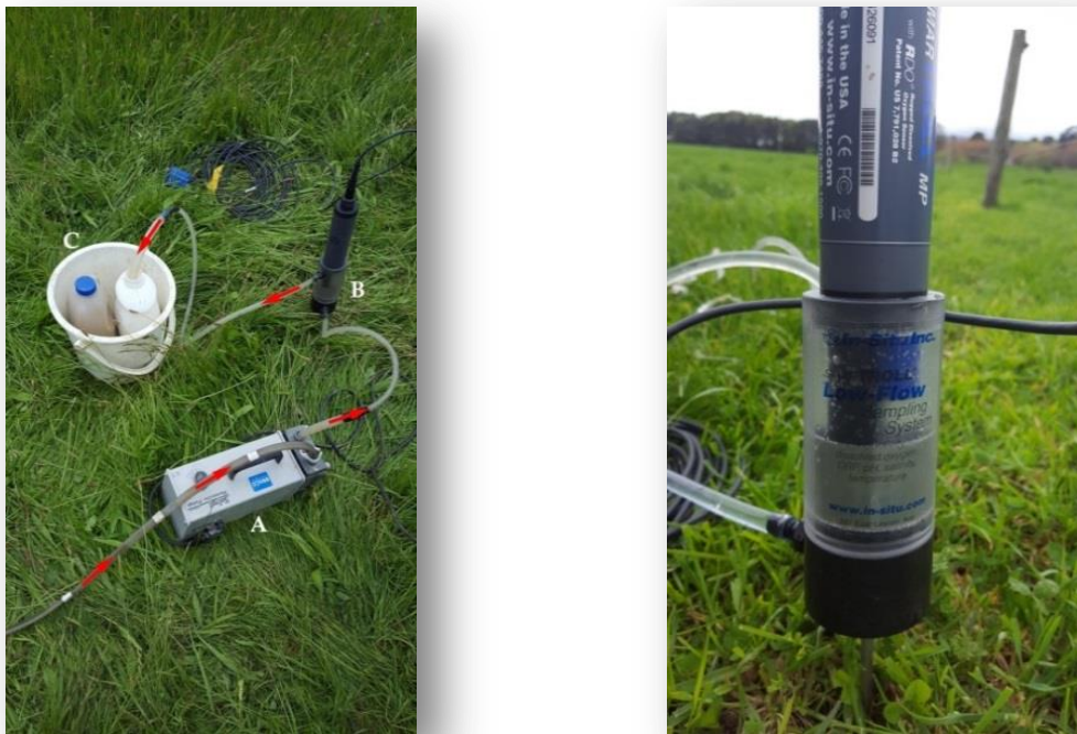
Figure 44: Left: Pump setup. Peristaltic pump (A), smarTROLL low flow cell (B) and container unit (C). Red arrows indicate flow direction. The bucket collected overflow ensuring a clean, mud free work area. The 2 litre containers were filled alternately and reduced the risk of well failure resulting in no samples collected. Right: SmarTROLL low flow cell; essential for pumping at low rates in less permeable facies.
