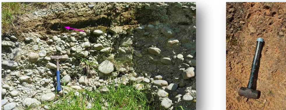
Figure 31: Gravels range from (left) large, sub angular clasts with high hydraulic conductivity such as the facies found in the Mangatainoka Plains (Namu Road, Mangatainoka ,40°24'18.9"S 175°53'11.1"E), to fine rounded to sub-rounded pebble sized clasts with poor hydraulic conductivity (right), (continued on following page).
