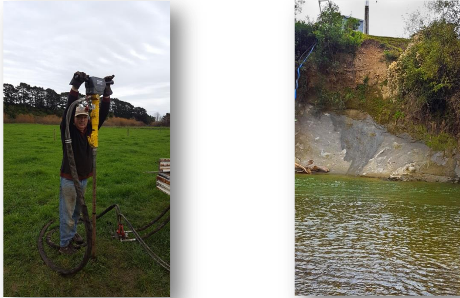
Figure 47: Beginning a well with the direct-push method (left). At times it was necessary to add more mass to the hammer to break through a difficult layer. When progress was arrested, it was difficult to determine whether a large gravel clast was the cause or well indurated mudstone as illustrated in the right hand image (Manawatu River, Kumeroa 40°20'34.5"S 175°58'59.9"E).
