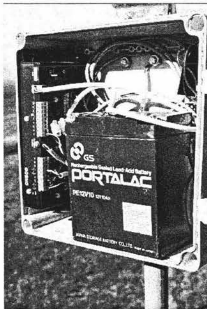
(b) the datalogger and battery
