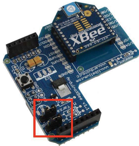
Fig 24: Arduino shield XBee-USB jumpers
