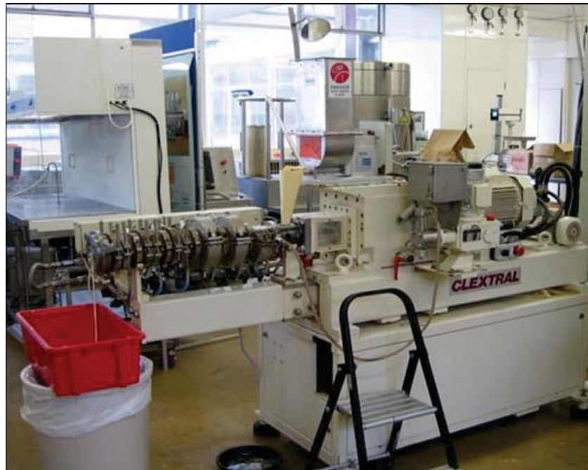
Figure 2-6 : A twin- screw extruder Clextral BC21, Firminy Cedex, France at Massey University, New Zealand
