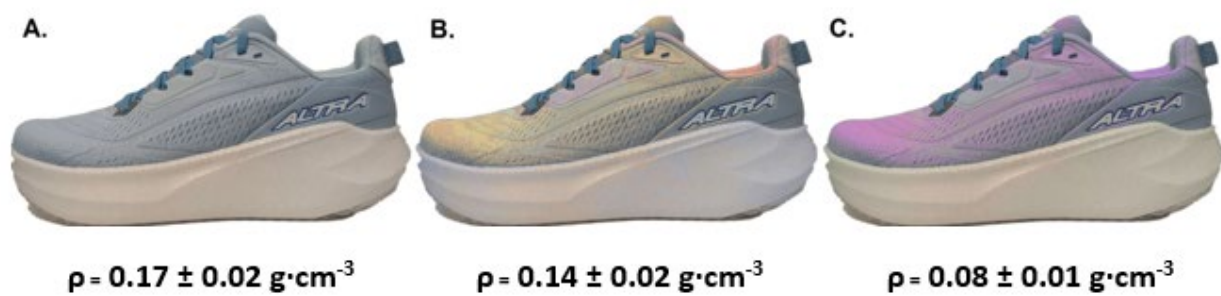
Figure 4.1. The three geometrically identical shoes used for the in vitro and in vivo experimental protocols, identified as Shoe A: high- \rho midsole, Shoe B: mid- \rho midsole, and Shoe C: low- \rho midsole, including the manufacturer's density specifications for each midsole
