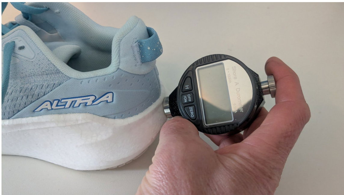
Figure 2.10. Example of Shore A measurement
