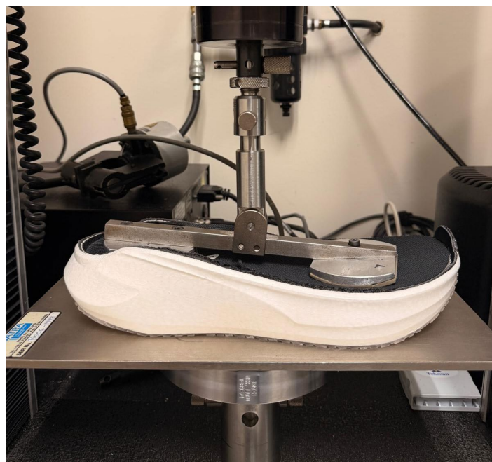
Figure 2.6. Shoe and Allied Trades Research Association (SATRA) Test Method TM183:1998 Whole Shoe Cushion Assessment, compressive testing machine with the upper of shoe removed to show the mechanical foot
