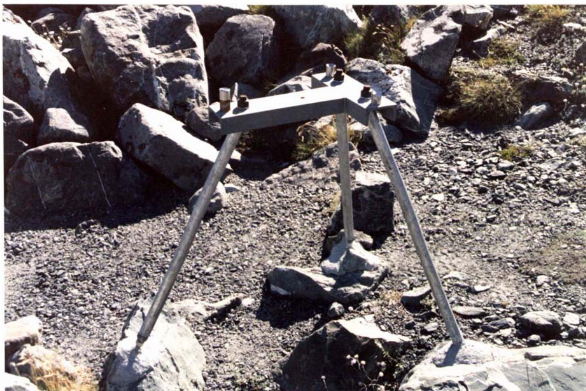
b: Kinematic mount base on tripod.
