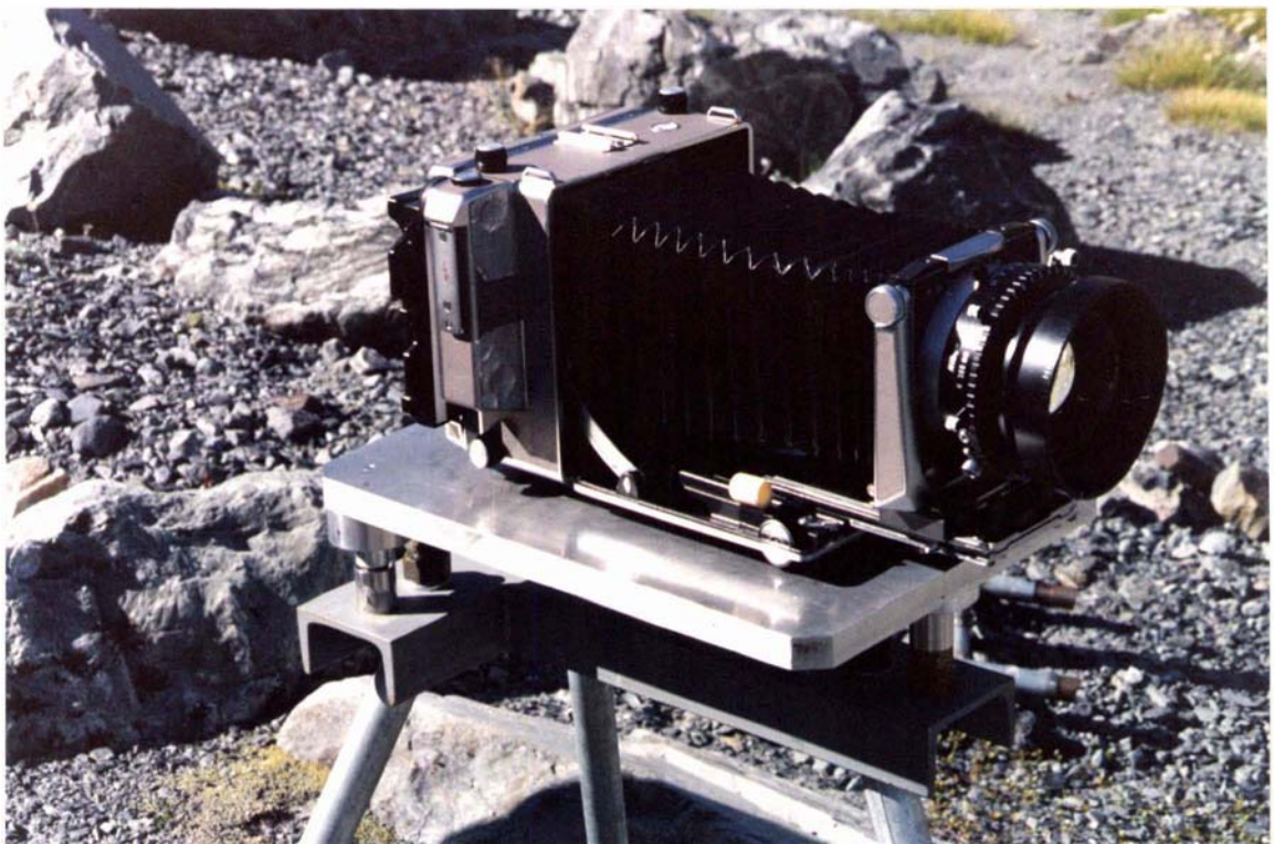
d: Camera is mounted on top half of kinematic mount. When the camera is placed on the tripod, the three hemispherical contacts under the top half sit in the three shaped fittings of the bottom half.
