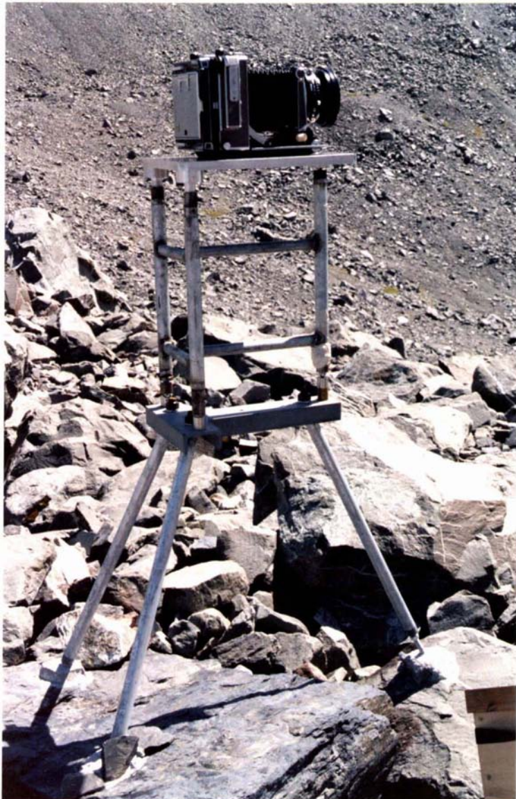
Figure 4-25: 400mm frame placed on rigid tripod to put the camera through a vertical in-plane translation.
