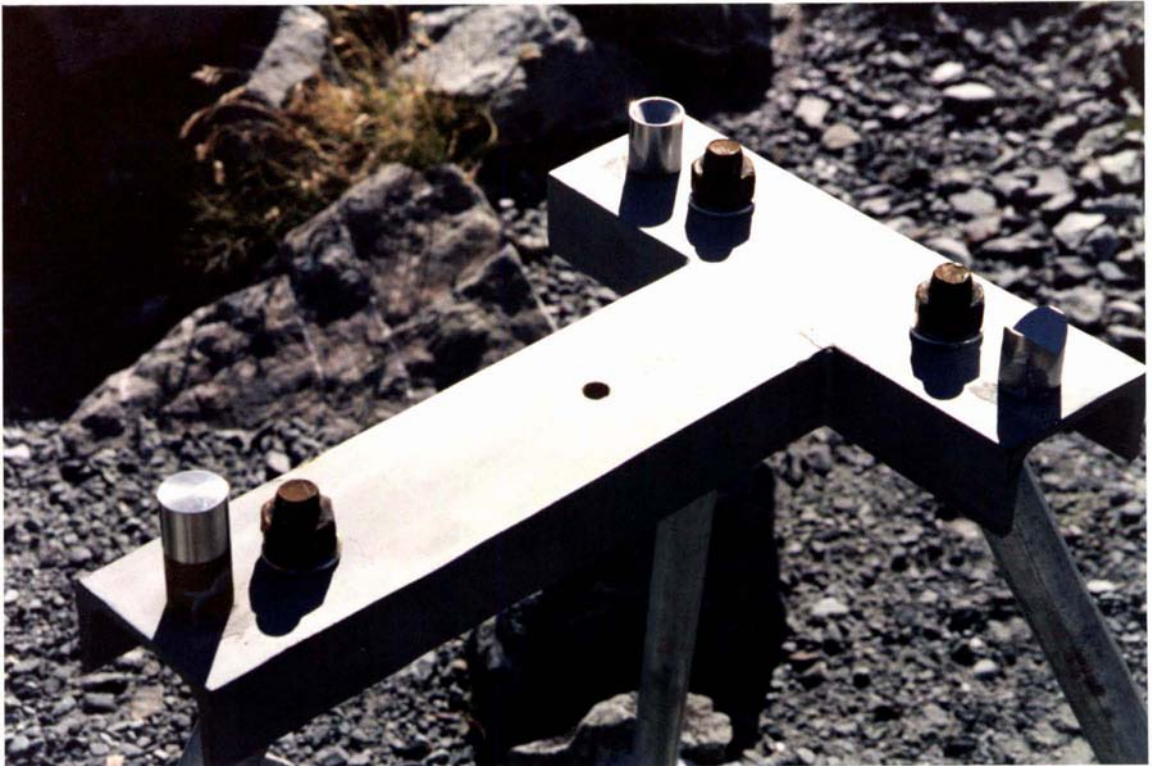
c: Kinematic mount base with flat, concave hemispherical and V-shaped fittings.
