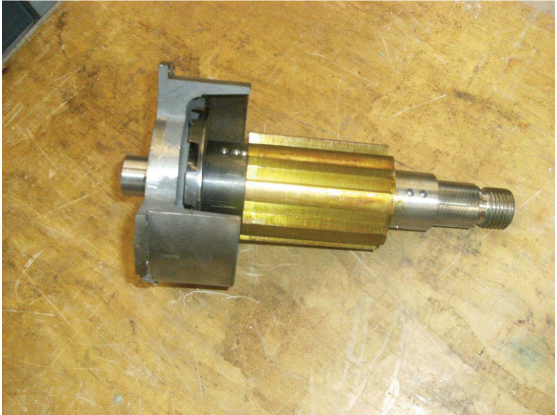
DVR SRM Rotor With Rear Shaft Bearing Housing. Note The Rotational Balance Drillings
