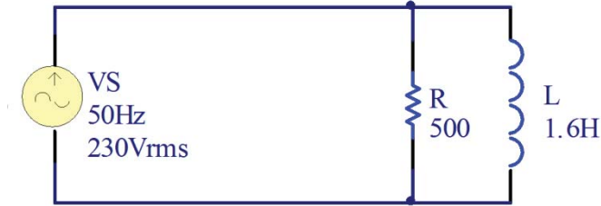
Figure 4-7: AC Circuit With Resistive And Inductive Loading
