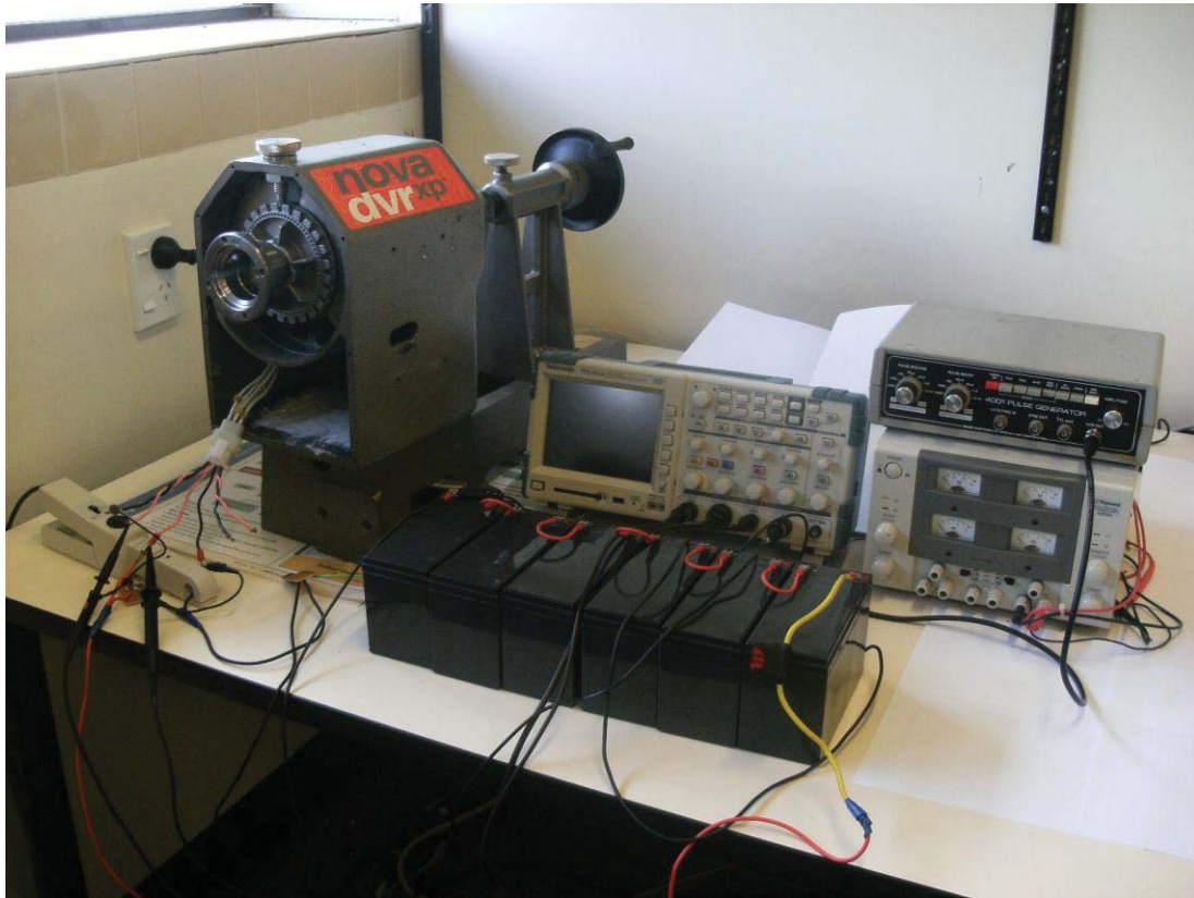
Experimental Setup of Teknatool DVR. Showing 72V Lead-Acid Battery Array, Tektronix Isolated Oscilloscope, Current Probe, DC Power Supply, And Function Generator
