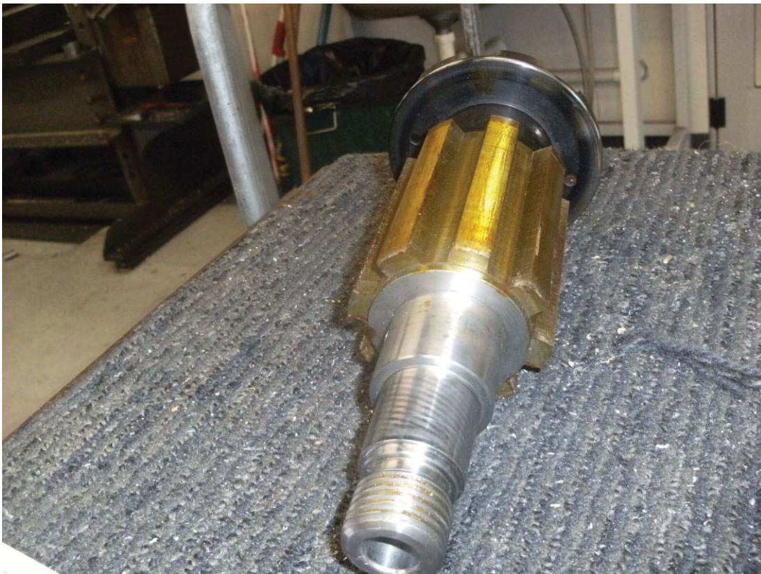
DVR SRM Rotor Showing 8 Trapezoidal Salient Poles
