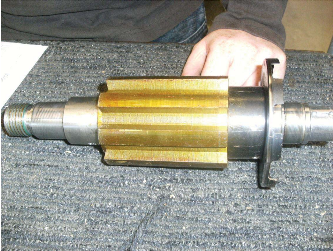
DVR SRM Rotor Showing Laminates And Rotary Position Encoder Wheel
