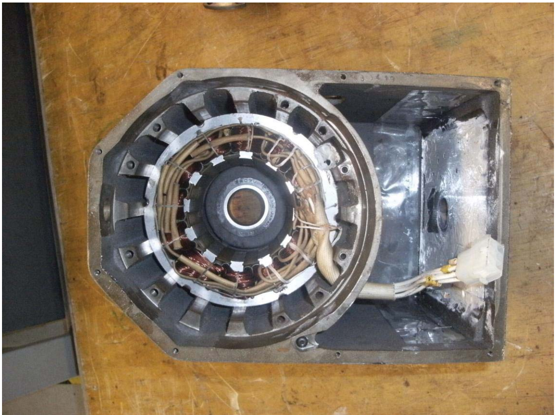
DVR SRM Iron Stator Housing Showing Windings And Electronics Cavity
