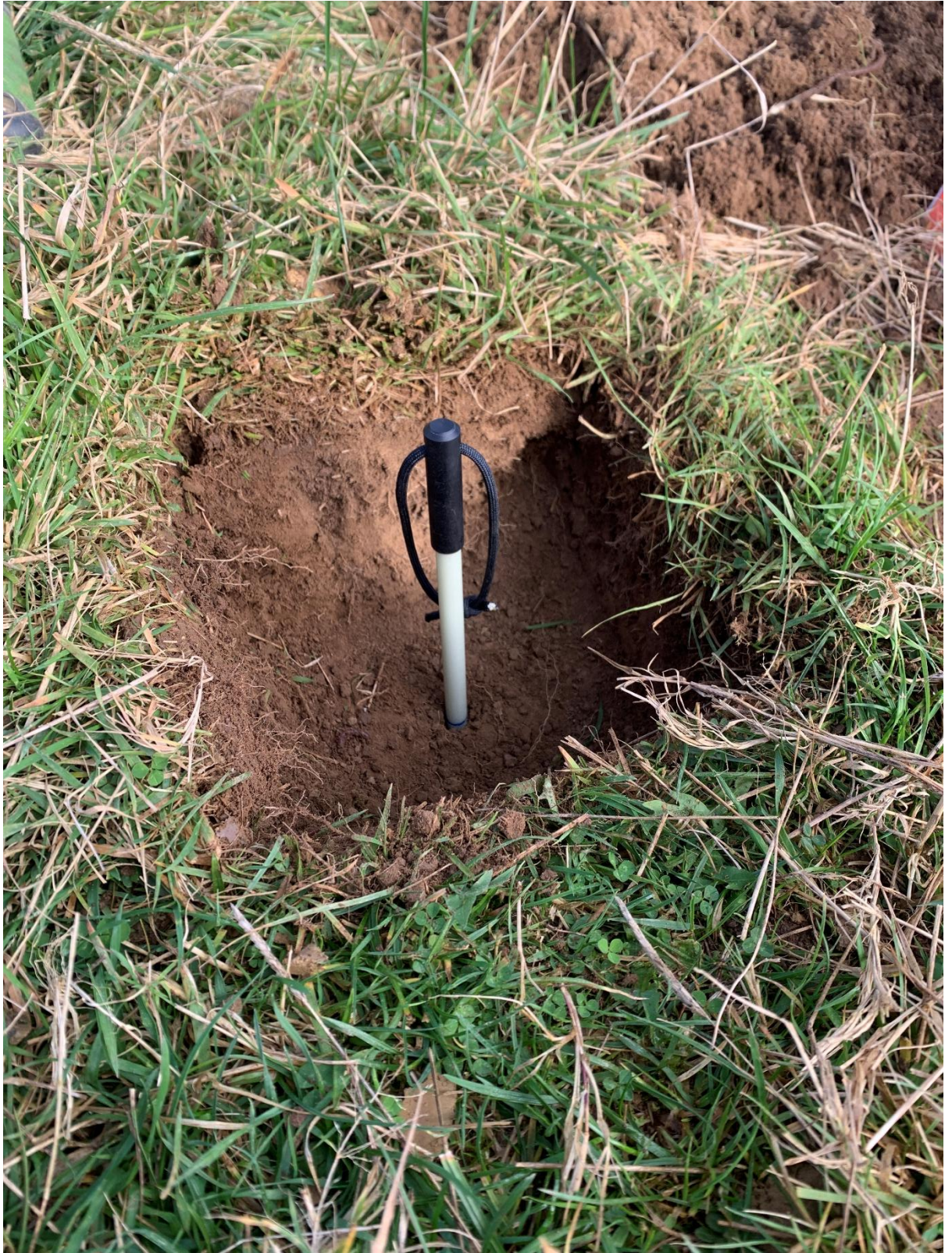
Figure E.2: Pre-drill is used to prepare a hole for the soil redox probe, drilled to the appropriate depth 10 cm below the surface.
