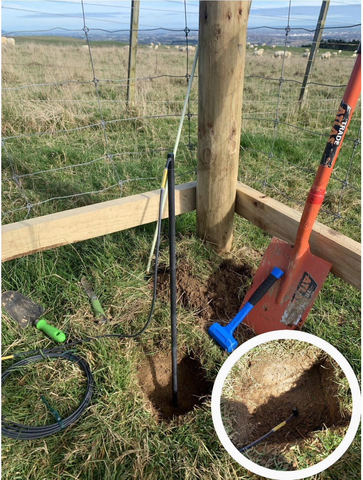
Figure E.3: Redox probe is gently hammered into the pre-drilled hole, 10 cm below the ground surface. Inset photo shows depth after being hammered in and subsequently covered over.
