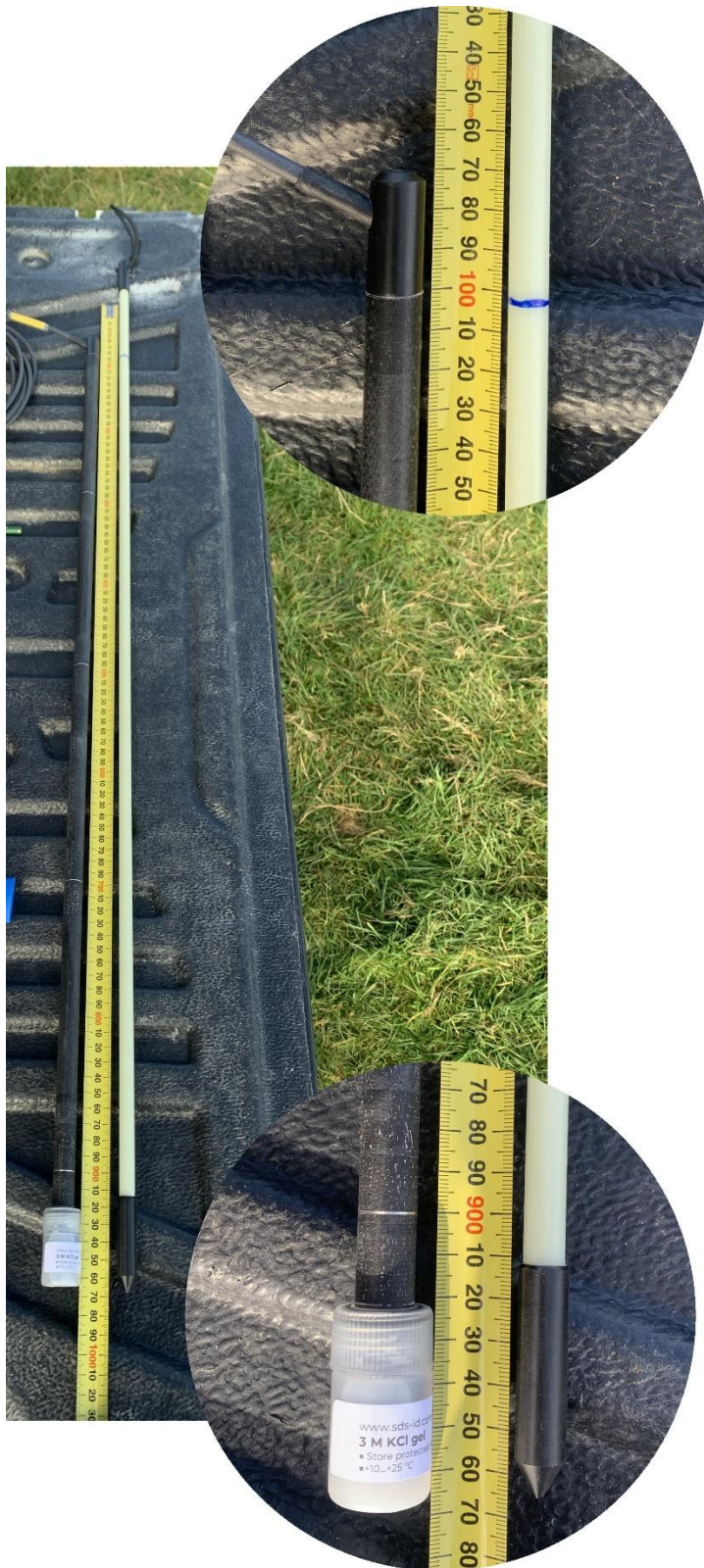
Figure E.1: Soil redox probe next to tape measure and pre-drill auger. The ORP-80-4-D soil redox probe has four platinum electrodes at 20, 40, 60 and 80 cm, but drilled 10 cm below the ground surface to a depth of 30, 50, 70 and 90 cm as shown in the photo. The plastic cap with electrolyte fluid was removed just prior to installation.
