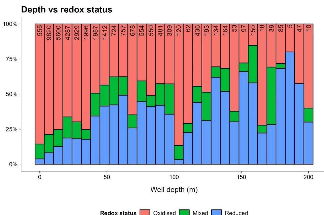
Figure 3.9: Relative distribution of groundwater redox status (derived from groundwater quality samples) per depth across New Zealand. The number of samples is shown at the top of each bin. Reproduced with permission from Springer Nature.
