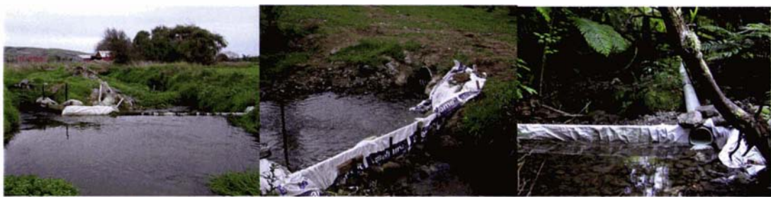
Figure 2. Weir and diversion structures used for experimental flow reductions at Booths Creek (left photo, intensive agricultural land use), Kiriwhakapapa Stream tributary (middle photo, low intensity agricultural land use), and Reef Creek tributary (right photo, pristine forested catchment). All streams are located in the lower North Island, New Zealand.
