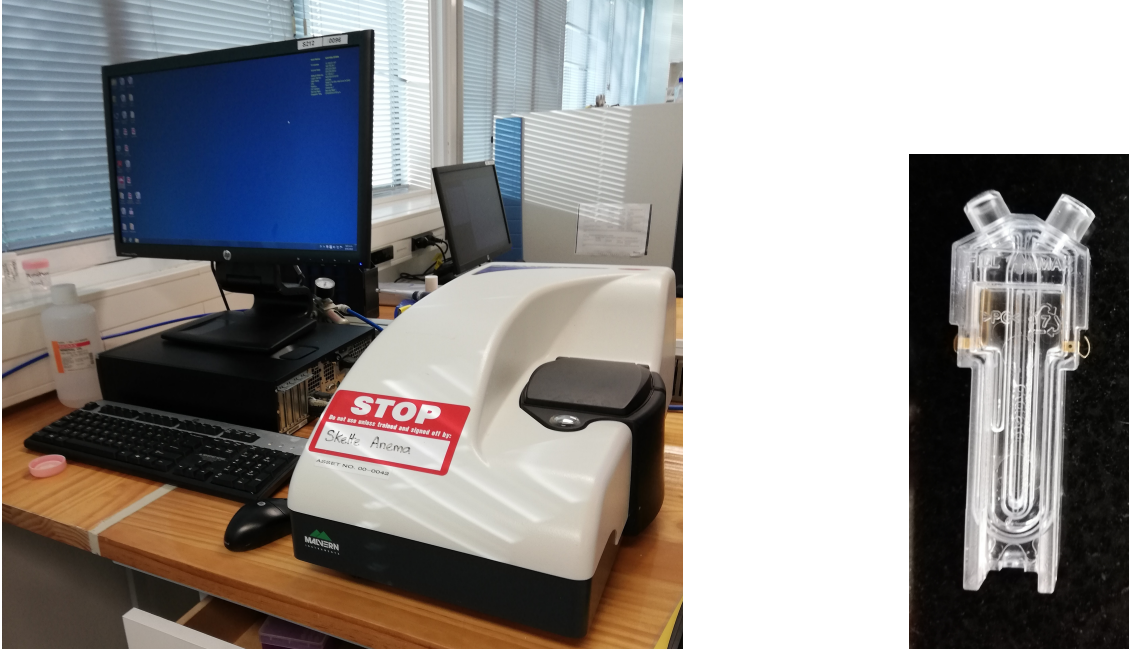
FIGURE 2.6: Zetasizer Nano used for measuring the zeta potential of the sample and the folded capillary cell to which the sample was injected (Malvern Instruments Ltd [51]).
