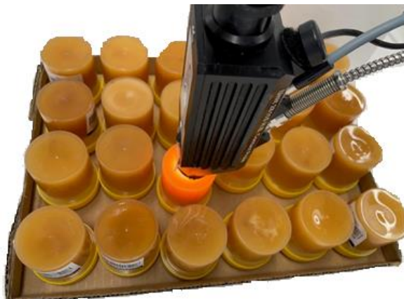
Figure 4.2. Scanning of reflectance spectral data of 1451 honey samples through the container transparent base using ASD spectroradiometer
