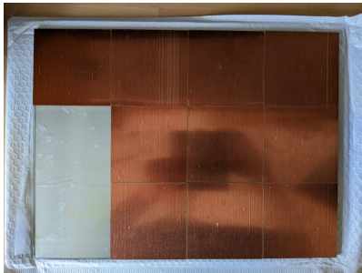
Figure 3.4: Calibration board backside with partially applied copper plates.
