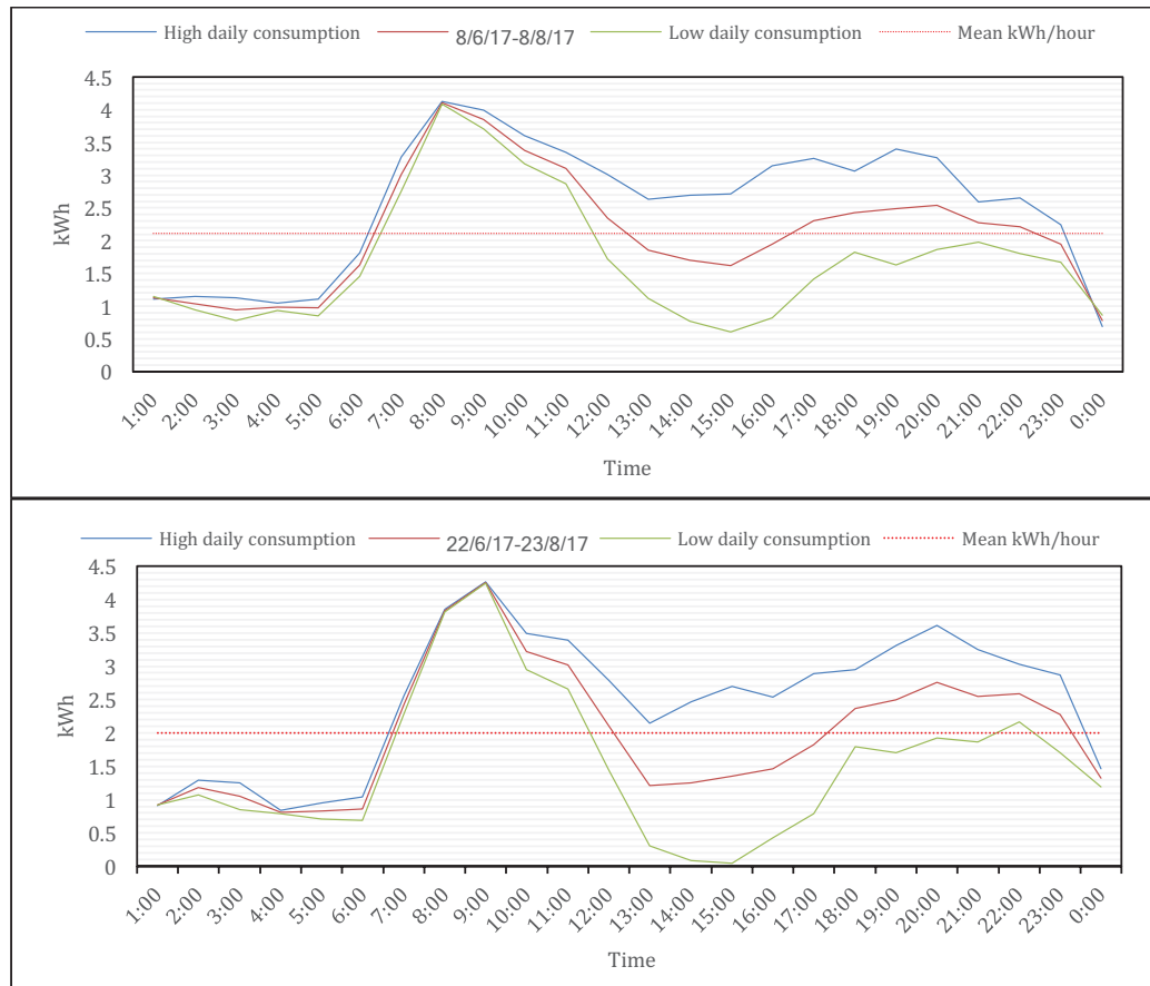
Figure 4.2: Winter 24h electricity use profiles – Top: Contact Energy Data; Bottom: Metering Data.
