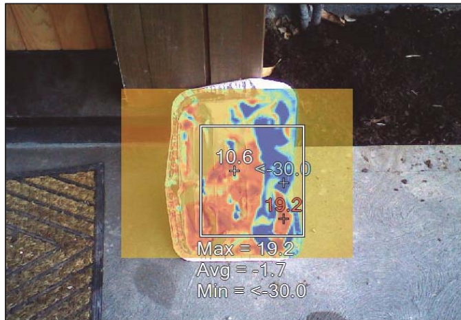
Figure 3.6: Visible image and thermogram of the aluminium baking pan.
