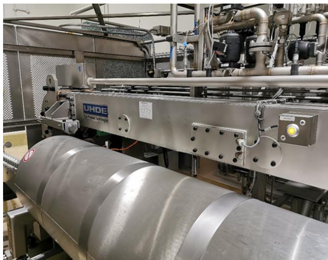
Figure 4.1 High-pressure processing (HPP) unit used in this project to treat avocado halves to inactivate PPO enzyme.
