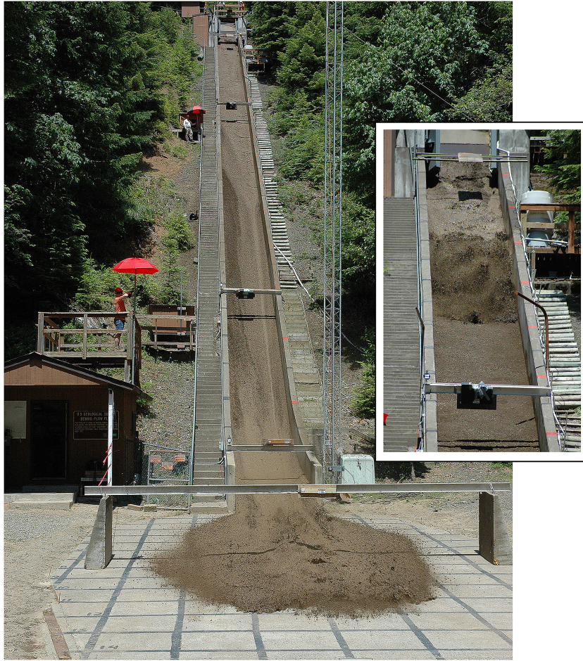
Figure 2.10: Photographs of a USGS flume experiment (U.S. Geological Survey, public domain), as presented in Iverson (2020), showing a debris flow entraining and interacting with wet bed sediment. Inset highlights the debris flow front and underlying sediment.
