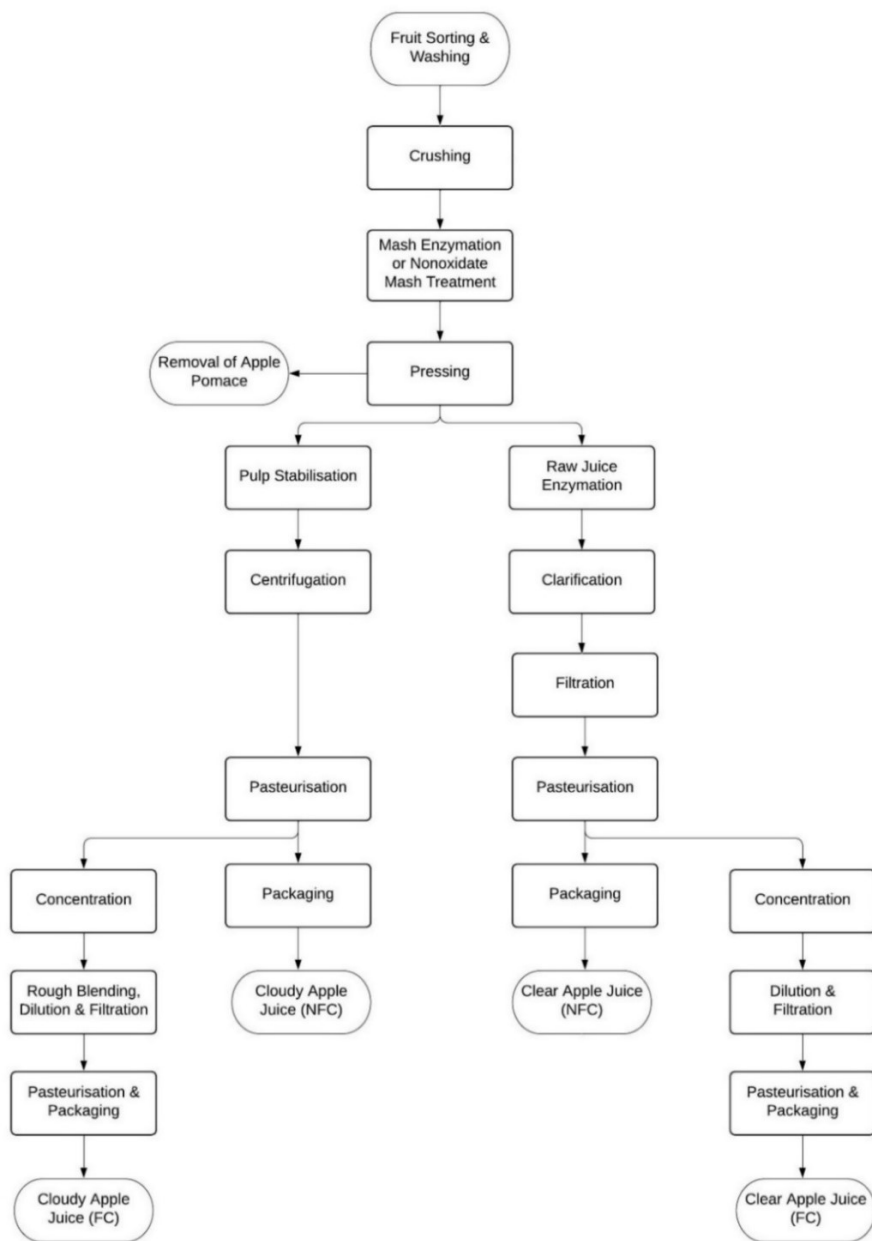
Figure 6. Flowchart of the process for both clarified and cloudy apple juice from concentrate (FC) and not from concentrate (NFC) adapted from Duan et al. (2023). 4
