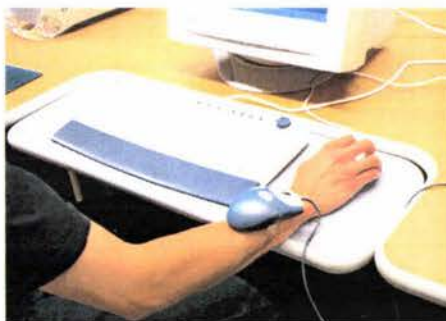
fig.40 Tests with different vibrations of a commercial force-feedback mouse fixed onto the lower arm.
