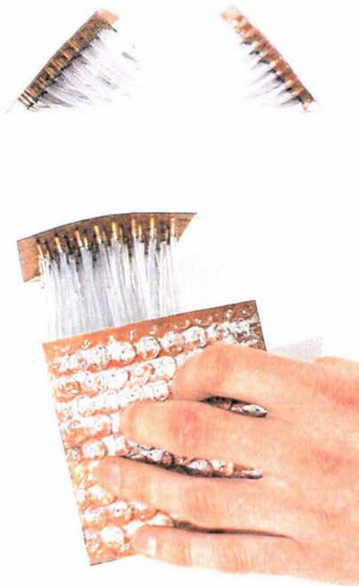
fig.37 Hydraulic Tactor Array designed to test tele-touch
