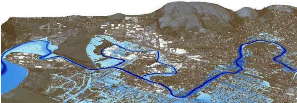
Figure 3 Hydraulic model studies Model for flood zone prediction - Heathcote River flooding prediction, southeast Christchurch (based on pre-earthquake topography) (NIWA, 2016c)
