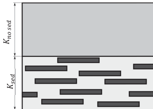
Figure 7.1 Settling of the filler in the coating profile
