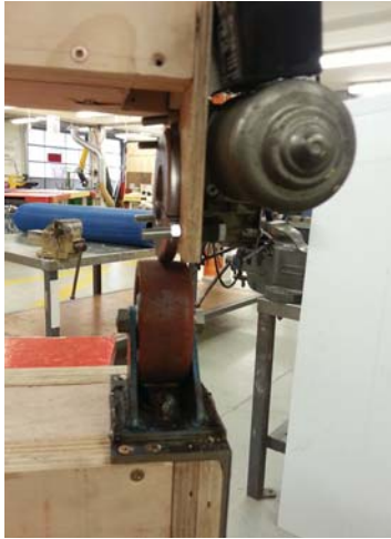
Figure 33. Adjustable press wheel for fold line width.
