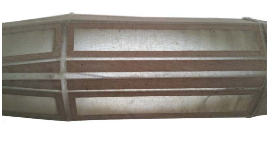
Figure 51. Transfer of light through the skin. Canvas over plywood frameless sheet to form alternative.
