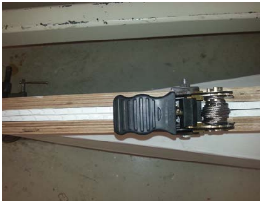
Figure 35. The trigger initiating and controlling the setup. A simple geared strap ratchet was used as a proof of concept in prototyping to wind the cable and create the tension to deploy the kayak.
