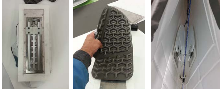
Figure 40. Foot rests and rudder steering pedals, from left to right: 1. The adjustable mechanism for low volume pack down. 2. The foot pedals with padding it pops up from flat. The nested position of the peddles for pack down.
