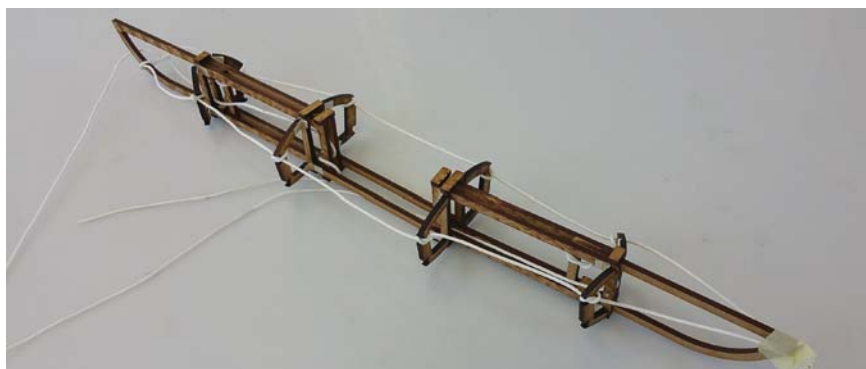
Figure 59. The chines replaced with cable. The cable would be tensioned allowing the skin to sit over the top.
