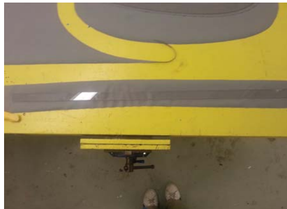
Figure 41. The polycarbonate cockpit rim. The cockpit rim is used to attach a sprayskirt and to stiffen the area around the cockpit for entry and exit.
