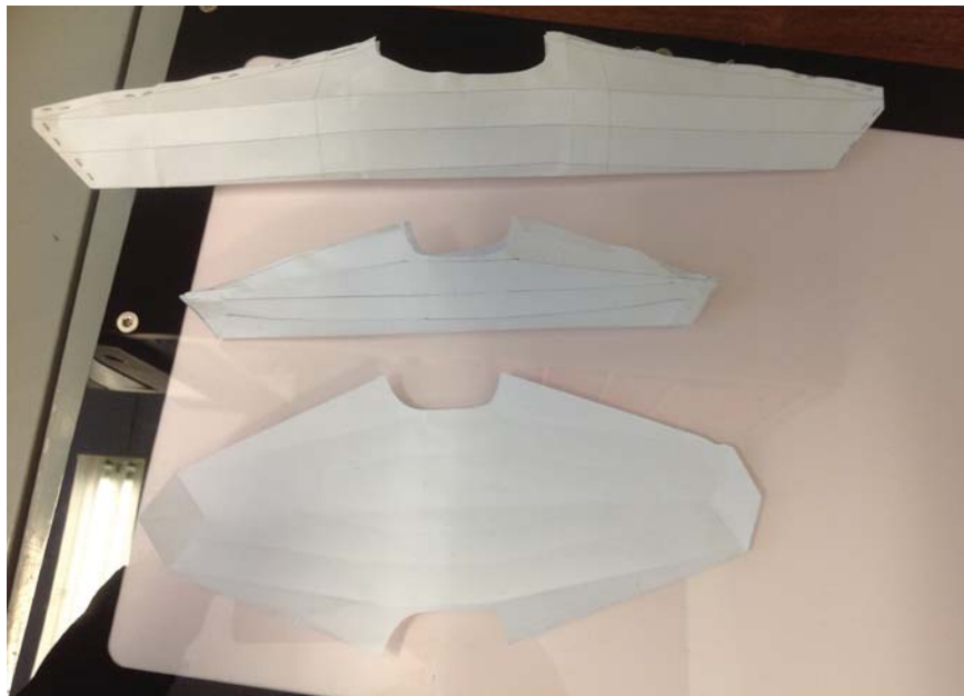
Figure 23. Iterations of paper kayak patterns. Early paper prototypes to understand pattern and material response, combining the Oru with my pattern ideas.
