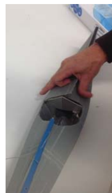
Figure 28. The cable pulls the kayak into shape.
