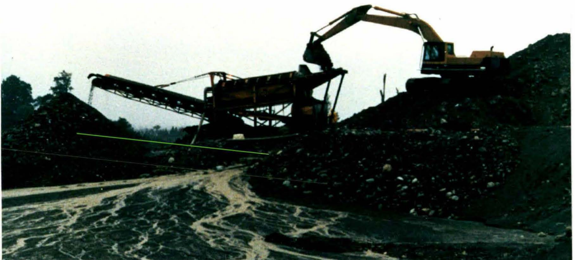
Figure 5.1: A hydraulic excavator and rotary screening plant working at a mining claim within Tuckers Flat (photo L. J. Brown)
