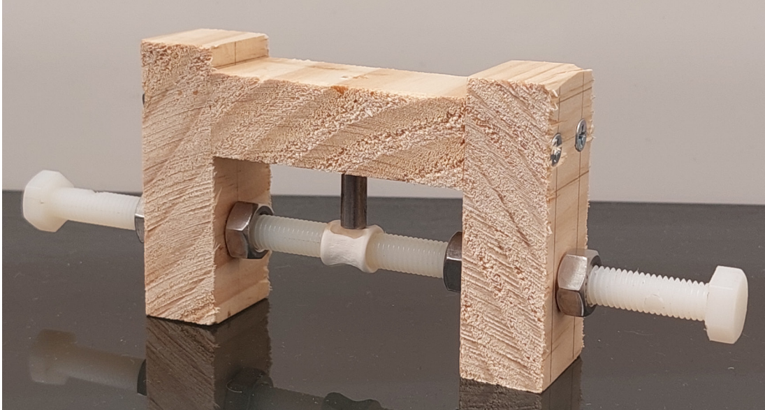
Figure 4.2: Custom made gluing stand to ensure that the cutting axis was in line with the focal axis of the vertebrae.
