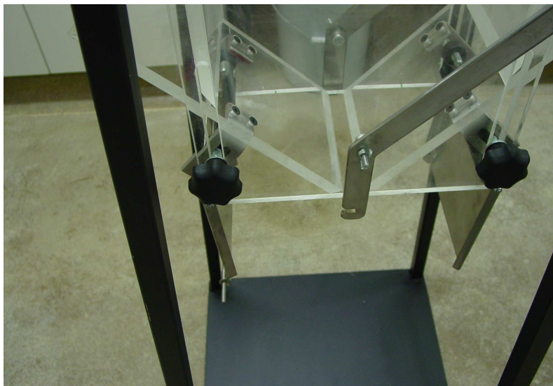
Figure 4.7: trapdoor that initiates flow
