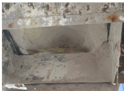
Figure 1.8: Shows an agricultural lime bridging in an aircraft hopper during flow trials, (Grafton et al , 2009b)
