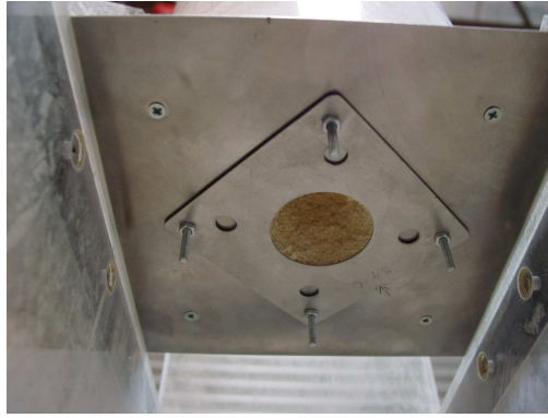
Figures 4.2: Overview of Beverloo device no flow, bridging over 37 mm orifice
