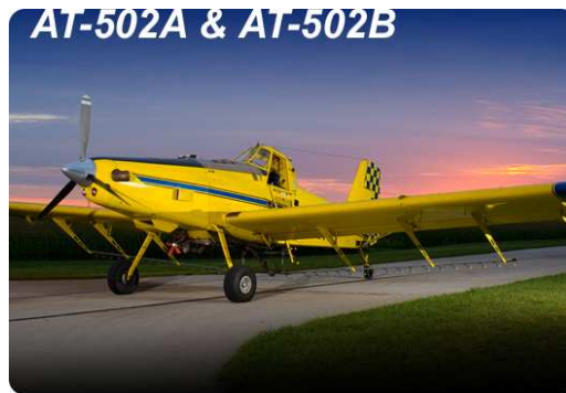
Figure 1.5: An Air Tractor 502 a conventional agricultural aircraft set up for spraying with CP nozzles. Source: Air Tractor Inc. Website
