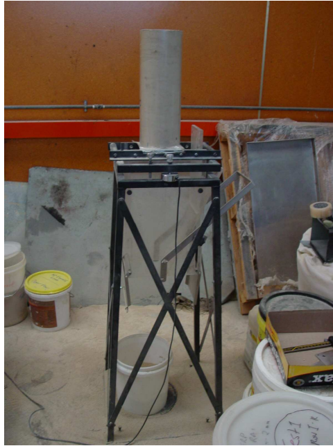
Figure 4.1: The perspex flow cylinder on frame resting on a 50 kg button load cell calibrated in LabView 8.2 student edition
