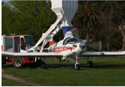
Figure 1.4: A Cresco agricultural aircraft with tricycle undercarriage being loaded with bulk solids on a grass airstrip. Source: Wanganui Aero Work (2004) Ltd Website
