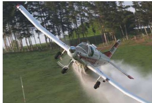
Figure 5.1b: Cresco 08-600 spreading superphosphate on North Island hill country (from Wanganui Aero Work (2004) Ltd website).
