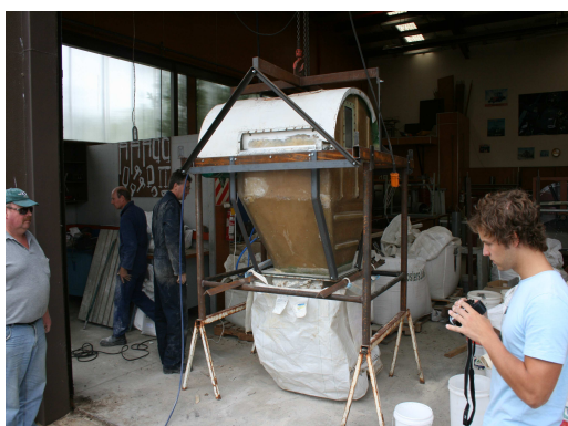
Figure 1.8: Shows an agricultural lime bridging in an aircraft hopper during flow trials, (Grafton et al , 2009b)
