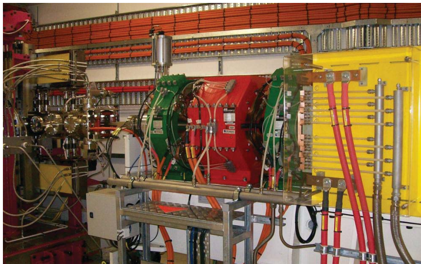
Figure 2. Magnets around the stainless steel pipe that contains the high energy electrons control the position of the electrons within the pipe as it goes around the synchrotron ring.
