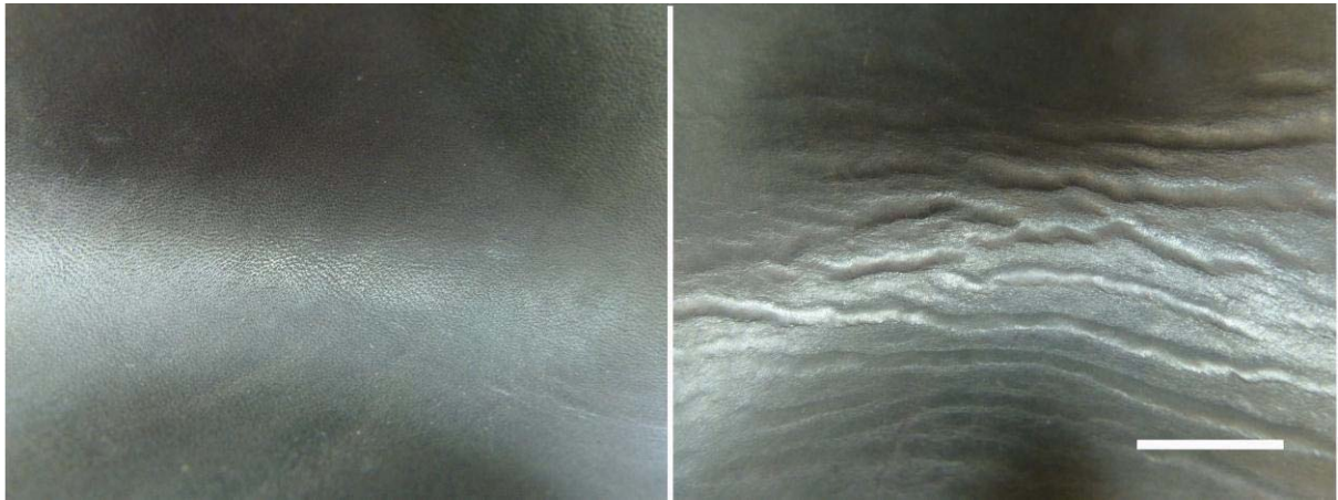
FIGURE 2: PHOTOS COMPARING THE SURFACE APPEARANCE OF TIGHT (LEFT) AND LOOSE (RIGHT) LEATHER WHEN BEING FOLDED INWARDS SLIGHTLY WITH THE GRAIN SIDE UP. THE SCALE BAR IS 2 CM.
