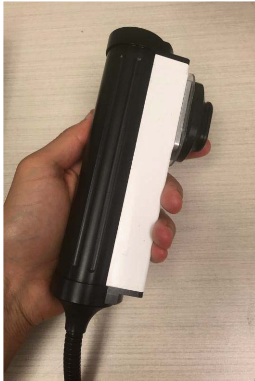
FIGURE 12: PHOTO OF THE TRANSDUCER PROBE USED FOR THE ANALYSIS ON LEATHER AND ADM MATERIALS. THIS TRANSDUCER WAS PURCHASED ALONG WITH THE DERMASCAN C USB DEVICE FROM CORTEX TECHNOLOGIES IN DENMARK.
