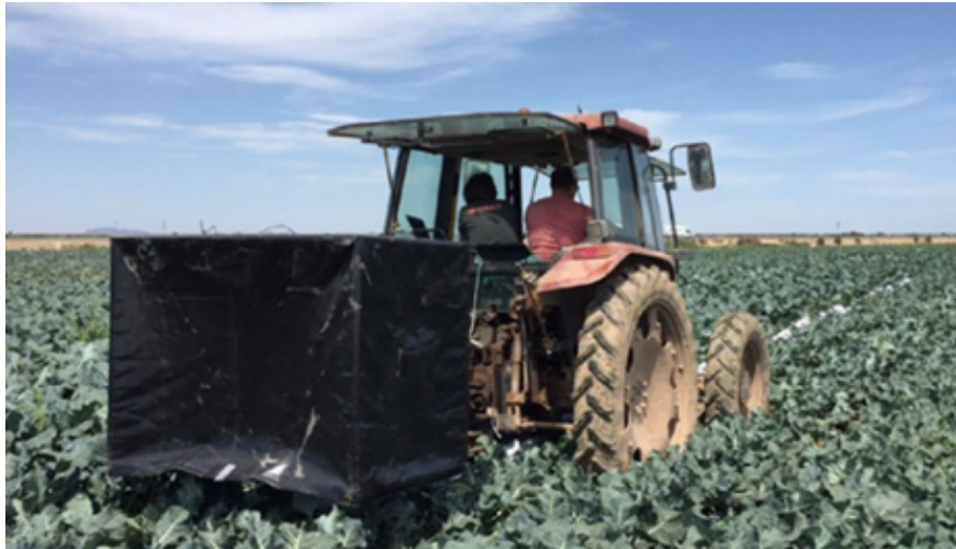
Figure 3.0.3: Experimental setup using tractor with enclosure and RGBD camera[43].
