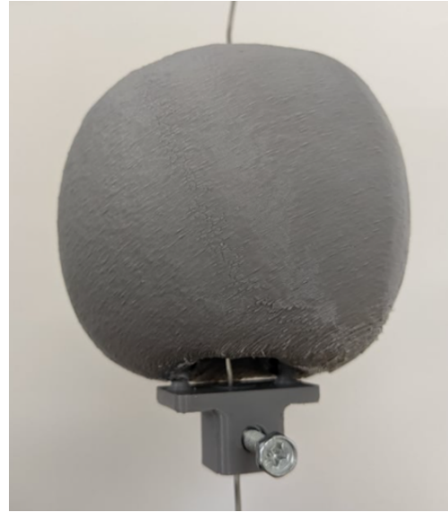
(b) 3D printed mount in position with 3D printed apple
